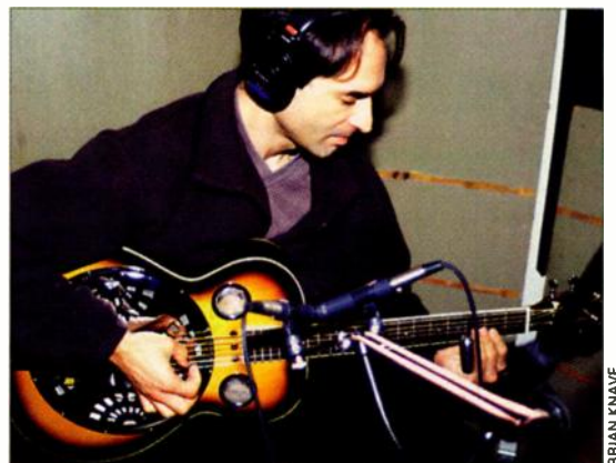
FIG. 2: Coincident-pair stereo-miking is good for capturing a realistic, although narrow, stereo image. This pair of Neumann KM 184 cardioid condensers sounded great on Weingarten's resonator guitar.
