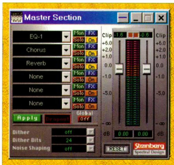
FIG. 3: The Master Section contains the controls for WaveLab 's real-time effects-processing functions. Here we see the EQ, Chorus, and Reverb effects in use, with the remaining three effects "slots" still free.
