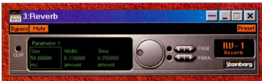
FIG. 4: Each VST effects plug-in presents an effects-rack appearance similar to its hardware equivalent.
