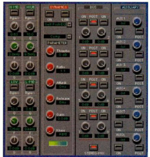
FIG. 3: Steinberg's Cubase VST/24 is one of several programs that offer support for the DSP Factory. In the Upper display of the DSP Factory Input Console, you can view channel EQ, dynamics controls, aux send levels, or bus send levels.
