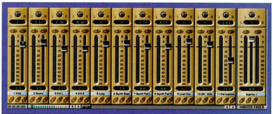
FIG. 2: In this example, the kick drum and one drum loop are right in the center of the mix, as in a live band. Because the synth bass has a heavy low-frequency content, I have panned it in the center, which also helps lock it in with the kick. The lead vocal and guitar solo are in the center and set hot. They don't occur at the same time, and they have different spectral content than the kick drum, drum loop, and bass, so each instrument will be distinct.
