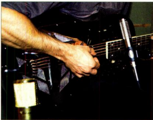
FIG. 4: We experimented with ribbon mics, in this case a Royer Labs R-121. The final position of the ribbon mic ended up being about two inches back and an inch or so higher than shown here, with more of a downward angle.
