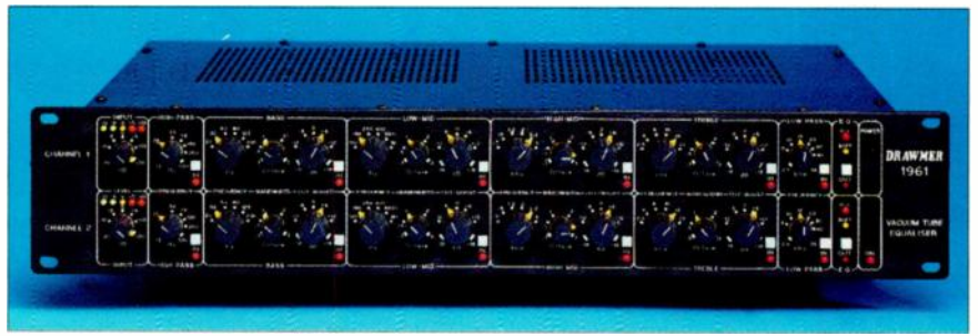
Equalizers such as this Drawmer 1961 are useful for timbrally separating instruments that are in the same range.
