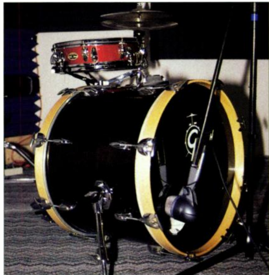
FIG. 5: The integral stand clamp on the Shure Beta 52 mic wouldn't work with a squat floor stand, so we had to use a boom.
