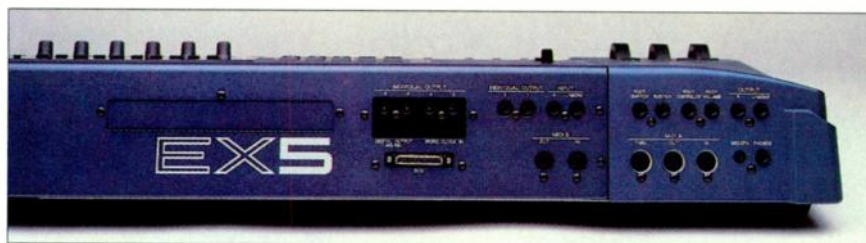
Yamaha offers several expansion options for the EX5. Shown here are the SCSI interface card and 4-channel analog-output board.
