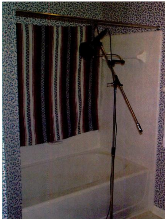
FIG. 1: Recording vocals in a shower stall requires proper mic placement. Here the singer stands in the center of the tub; the blanket dampens excessive reflections.
