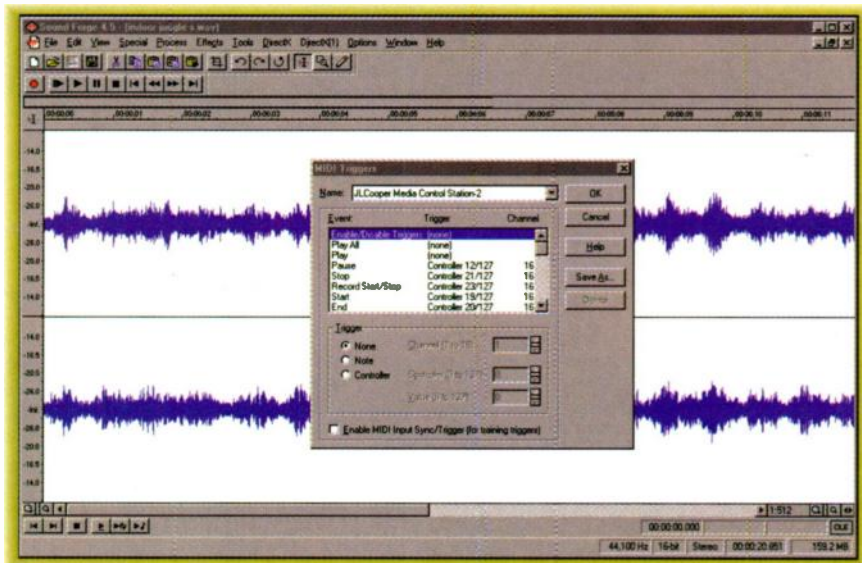
FIG. 2.3: MIDI triggers can be used to control many of Sound Forge's commands, including basic transport and editing options.
