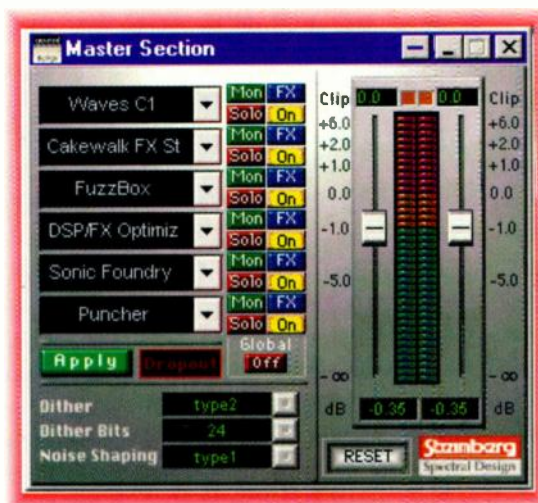
FIG. 2.8: The Master Section in WaveLab provides access to all the plug-ins you have loaded. Up to six plug-ins can be running at once, and you can change their settings in real time.
