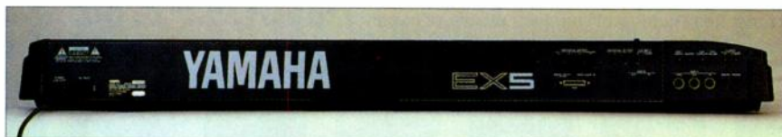
The stock EX5's rear panel provides two analog inputs and outputs, a headphone jack, and three footswitch jacks, in addition to MIDI In, Out, and Thru ports.
