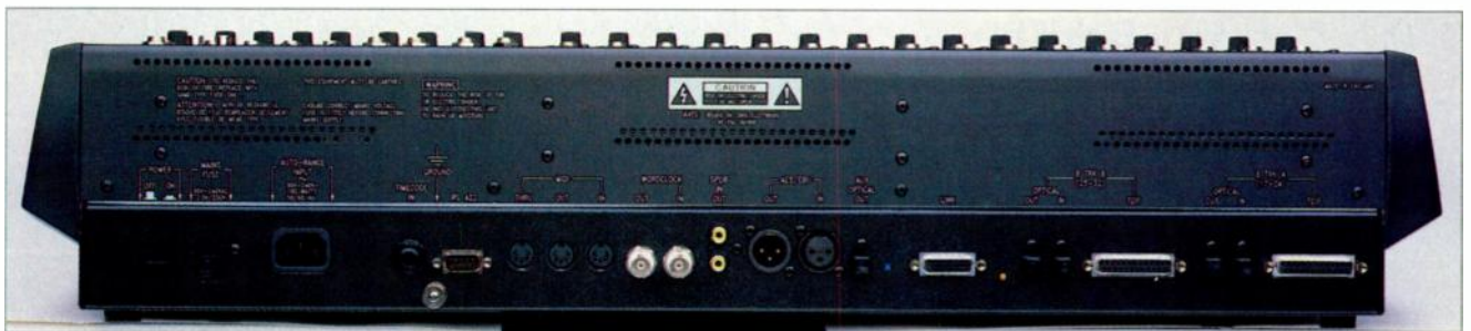
FIG. 1: In addition to flexible analog I/O, the Digital 328 has several digital I/O options, including floating S/PDIF and AES/EBU, two sets of TDIF ports, two sets of ADAT Optical ports, and a separate ADAT Optical aux output. You also get a variety of control ports and a Link port for cascading two consoles.
