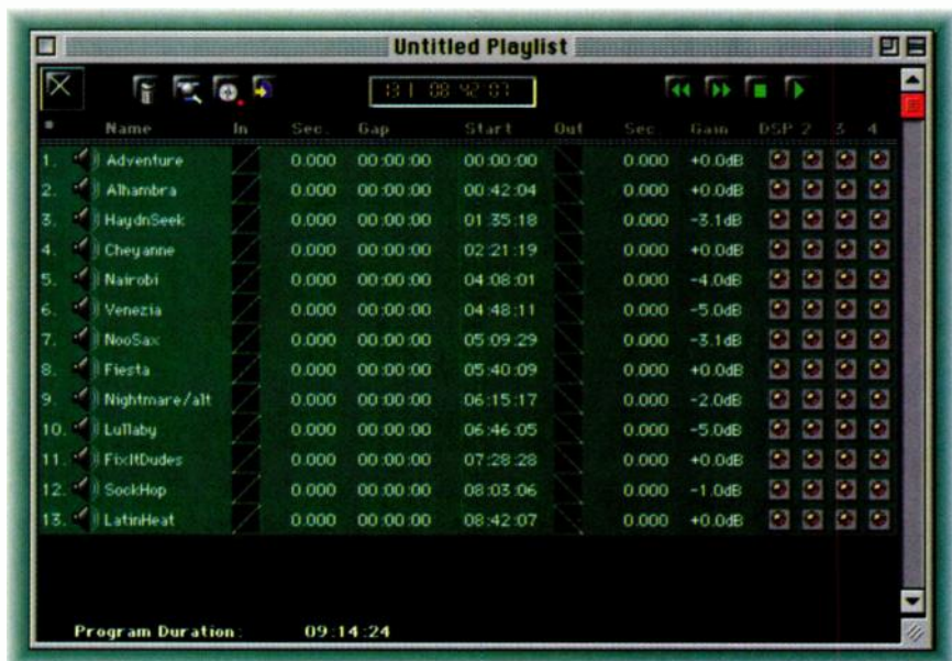
FIG. 1.7: Peak is the only program in this group that offers true playlist editing. You can apply up to four plug-in effects per event and sync the list to incoming SMPTE time code for post-production work.
