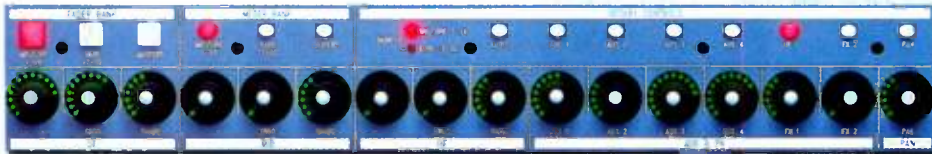
...OR A ROW OF 16 AUXES OR FX SENDS FOR THE 16 FADERS BELOW THE E STRIP.
