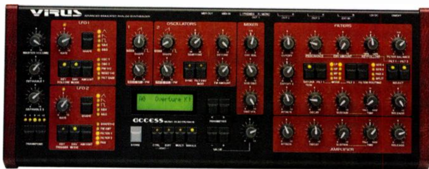
The Access Virus is a compact physical-modeling synthesizer designed to emulate analog synth sounds. Features include an arpeggiator, vocoder, and easily upgradable operating system.
