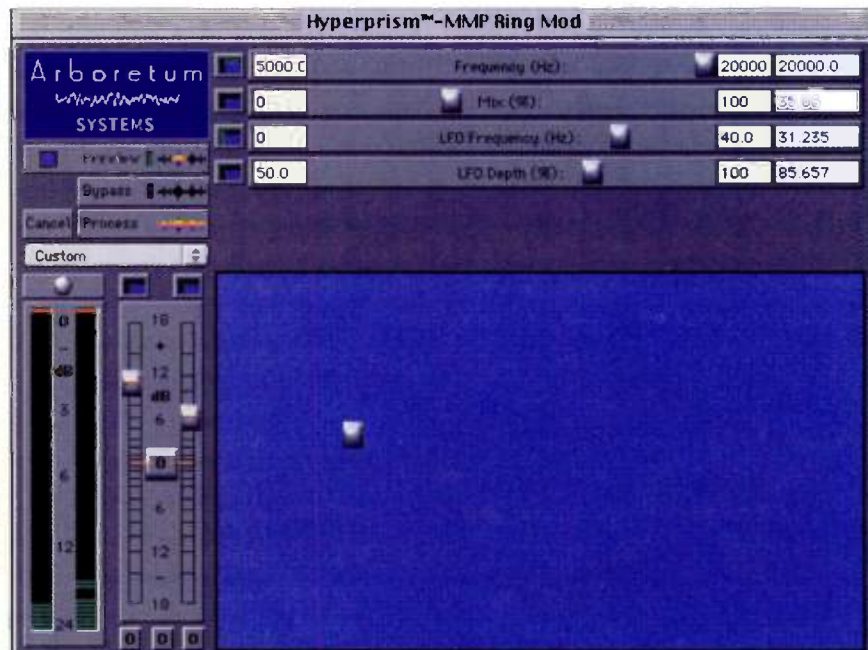
FIG. 2: The Ring Modulator effect multiplies a sound by a sine wave to add additional components to the signal.
