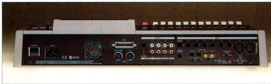
FIG. 1: The VS-1680's eight RCA outputs (center) can serve as individual channel outputs or can be grouped into pairs to function as the master, aux, and monitor outs. Each pair is assigned separately. The coax and optical digital S/PDIF outputs (lower right) can carry different signals simultaneously, but the digital inputs are an either/or proposition.
