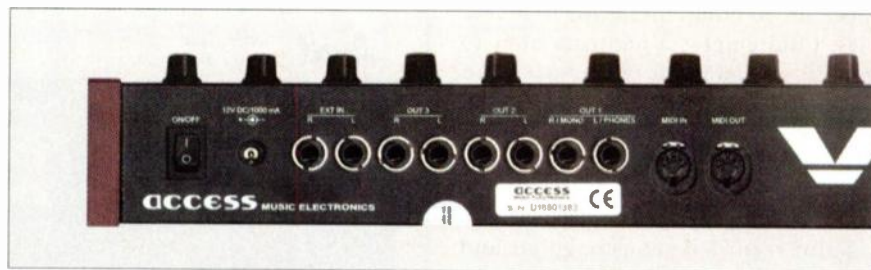
FIG. 1: The Virus's six unbalanced 1/4-inch outputs can be configured as three pairs of stereo outputs. One of the six doubles as a stereo headphone jack. The audio input jacks feed into the filter section and allow you to apply distortion, panning, amplification, envelopes, and effects.
