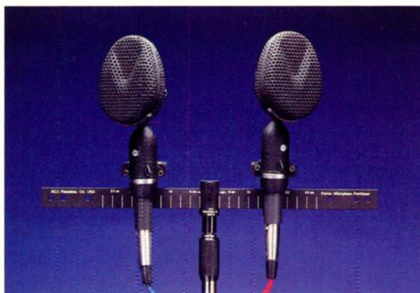
Designed by the BBC and renowned for its smooth sound, the Coles 4038 ribbon mic is just as useful today as it was when first introduced in the mid-1950s. Here, two 4038s are positioned on a stereo bar.
