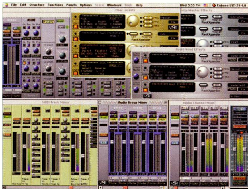
FIG. 4: You'll need a pretty big monitor if you want to use all of Cubase VST/24's audio and MIDI mixers and effects. The new MIDI Track Mixer appears in the lower left, showing several of the available XG and GS editing controls.
