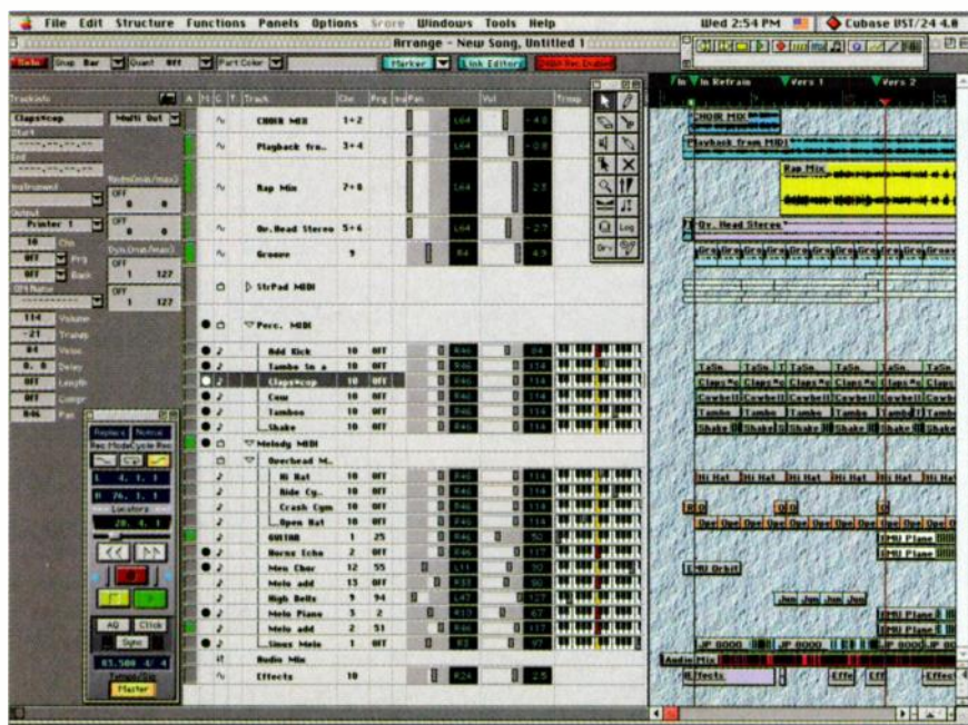
FIG. 1: Cubase VST/24's newly enhanced Arrange window includes an expandable Inspector section with additional parameters. The Arrange window also lets you display faders for volume and panning and miniature keyboards for quickly transposing MIDI Tracks. The new customizable toolbar appears in the upper right, just above the new Markers Track.
