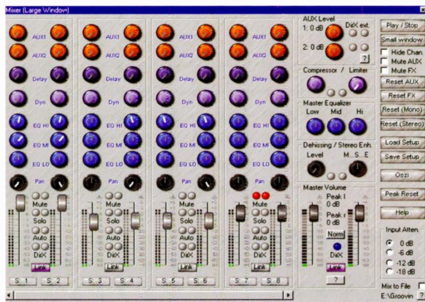
FIG. 2: The Mixer window now lets you simultaneously access DirectX plug-ins from within each track, auxiliary sends, and the Master Volume section.
