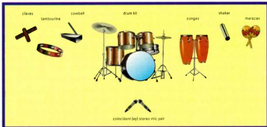
FIG. 2: To create stereo samples of percussion, I first make a "map" of where the instruments will be positioned on the soundstage. Then, rather than move the mics around, I move the musicians, placing them at the spots I have chosen for their particular instruments.
