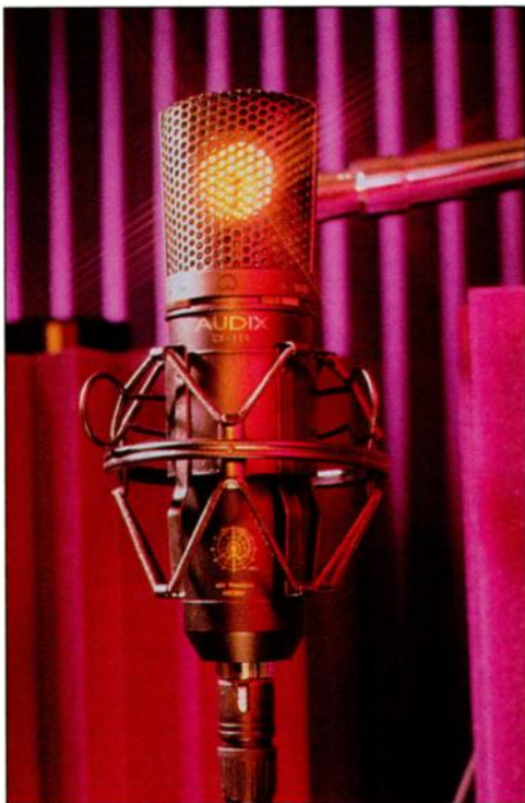
The Audix CX-111 is a cardioid-only, true condenser mic featuring a 1-inch diaphragm, 10 dB pad, and 200 Hz bass rolloff. It sounds great and is very affordable.
