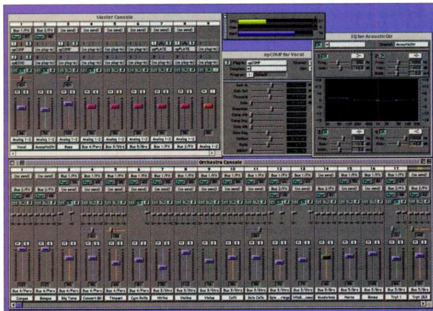
FIG. 1: Vision DSP 's console is shown here with the CPU/Disk/RAM window, an EQ window, and Opcode's opCOMPVST compressor plug-in.
