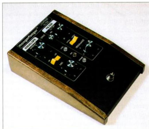
FIG. 1: The Moogerfooger Lowpass Filter is a voltage-controlled, variable-resonance filter that offers control of signal mix, cutoff frequency, and envelope amount.
