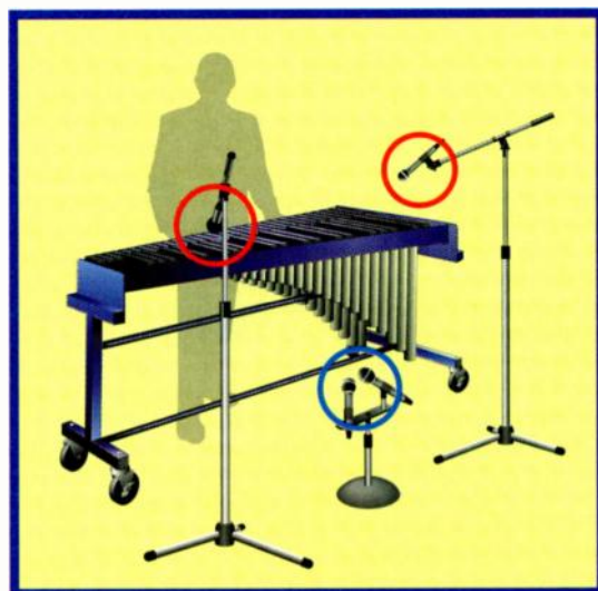
FIG. 4: To emphasize the attack of a mallet instrument, position the mic pair above the bars, pointed down (red circles). For a mellow, more resonant, less percussive tone, pull the mics back from the instrument and position them lower, aiming up toward the resonators (blue circle).
