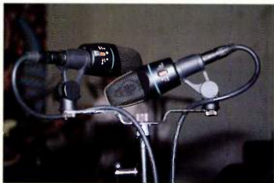
This close-up shows the XY configuration of AKG C3000s the author used to record the Apes of God.
