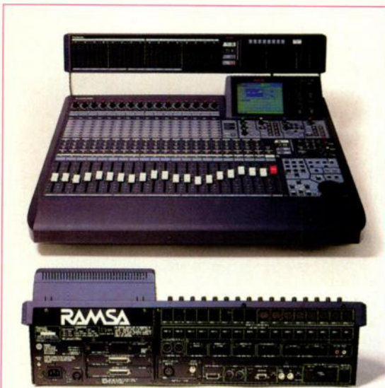
Designed for the musician, the Panasonic/Ramsa WR-DA7 provides dedicated front-panel controls for EQ, dynamics, pan, and aux send and bus assignment. The stock I/O is limited, so if you buy this board you'll need to budget extra money for expansion cards.
