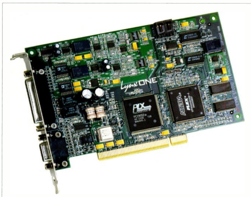
Lynx Studio Technology's LynxOne audio card is an excellent choice for mastering. With support for digital I/O at rates of up to 96 kHz at 24-bit resolution, A/D/A converters that offer 48 kHz and 24-bit support, 32 MIDI channels, and word clock, the LynxOne is suitable for today's professional studio.
