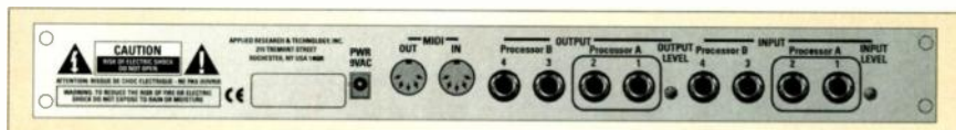
FIG. 1: The back panel of the DMV-Pro is as uncomplicated as the front panel, with an input- and output-level button, four discrete unbalanced 1/4-inch inputs and outputs, and MIDI In and Out ports.
