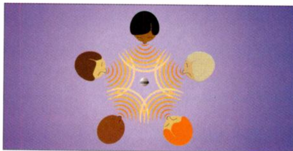
FIG. 1: Even when confined to a single track, you can capture a realistic a cappella performance using a dual-capsule mic in omnidirectional mode.
