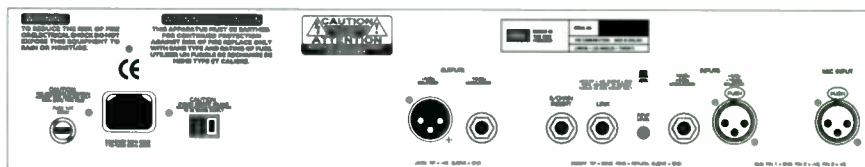
FIG. 8: The back panel of the Radius 40 includes both a link jack and a combination sidechain/insert jack.
