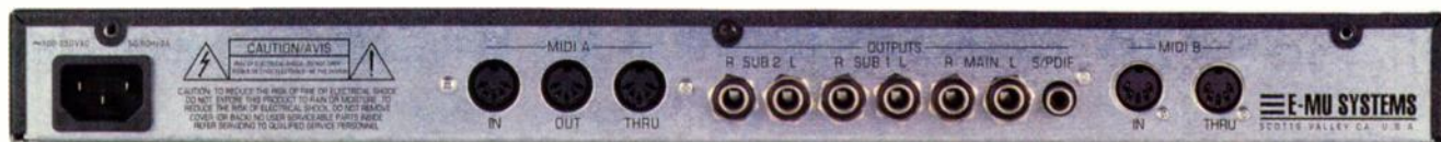
FIG. 1: The Proteus 2000 offers two sets of MIDI ports as well as analog and digital outputs. The digital output duplicates the main outs.
