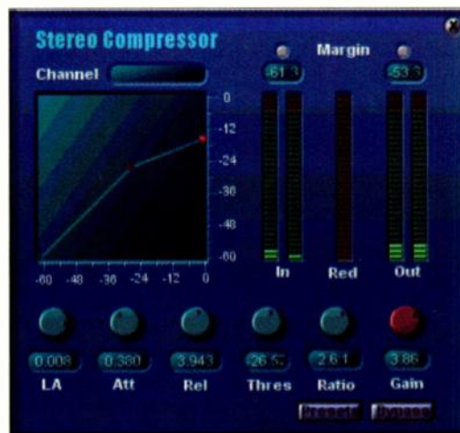
FIG. 4: Pulsar has several useful effects, including the compressor shown here. Notice the input/output curve and real-time meters.
