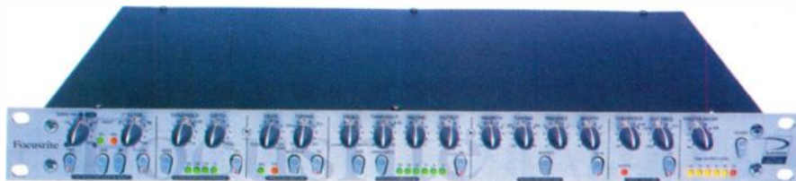
FIG. 5: Focusrite's Platinum VoiceMaster contains a Class A mic preamp, an opto compressor, and an opto de-esser.
