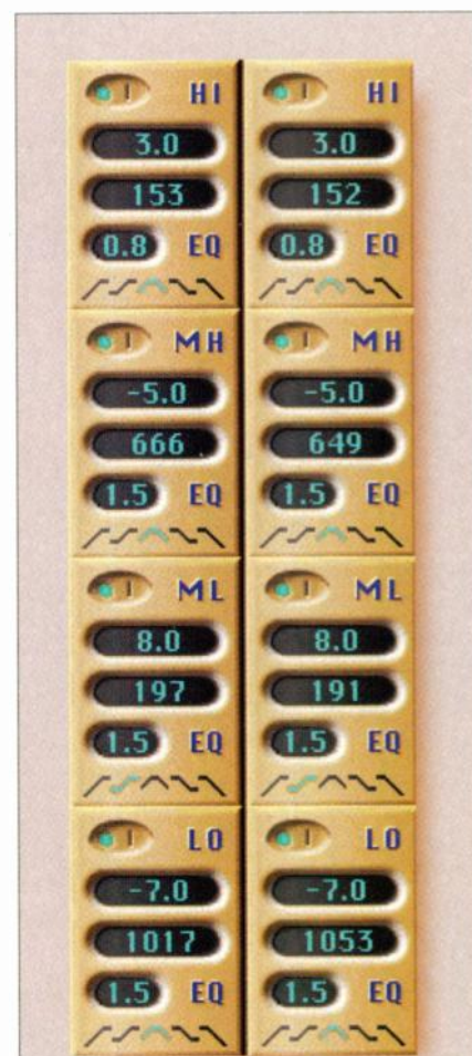
FIG. 4: The EQ for an overhead pair of drum mics, displayed in Ensoniq's Paris hard-disk recorder. The only other drum mics were on the kick drum and snare. For each EQ band, the top parameter is gain, the middle parameter is frequency, the lower parameter is bandwidth, and the bottom icon indicates the filter type (bandpass or shelf). Note that the Paris defaults to a bandwidth of 1.5 for shelving filters.
