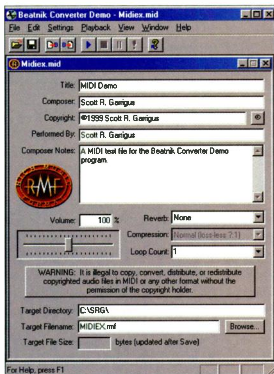
FIG. 1: Beatnik Converter enables you to create RMF files that hold the MIDI and audio files used in your composition.
