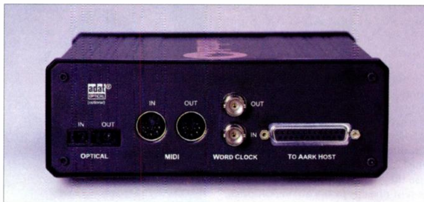
FIG. 2: The back panel of the Aark 20/20+ interface box has optical S/PDIF I/O—which can also be used for 8-channel Lightpipe I/O when the ADAT expansion option is installed—as well as MIDI In and Out ports and a pair of BNC connectors for word-clock I/O. The front panel provides eight channels of analog I/O and two channels of electrical S/PDIF.
