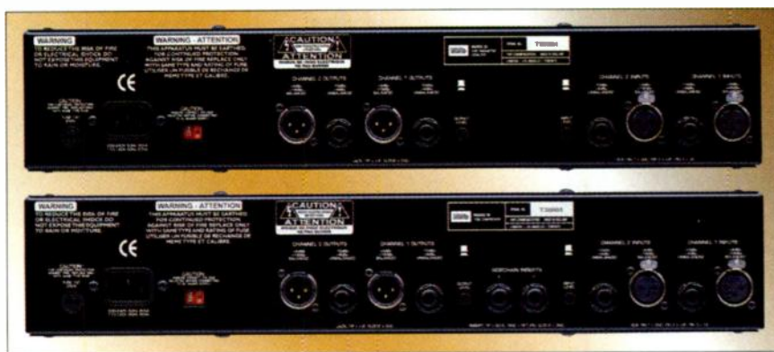
The Radius 20 (top) and Radius 30 have balanced +4 dBu and unbalanced -10 dBu I/O. To make interfacing even easier, rear-panel input- and output-level switches convert the balanced connections to +18 dBu and the unbalanced connections to +4 dBu. The Radius 30 (bottom) also offers a sidechain insert point for each channel.
