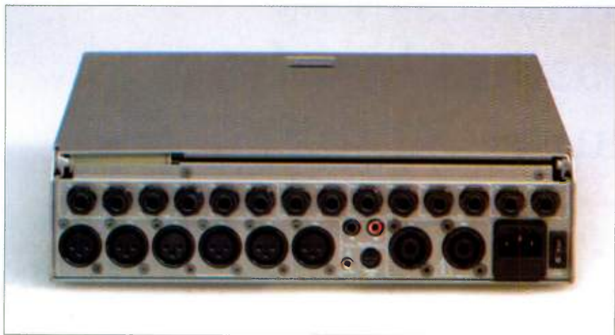
The NoteMix provides six dedicated mic/line channels and four double-duty channels on TRS jacks. The 1/4-inch line inputs double as inserts when the XLR channels are used for mics.
