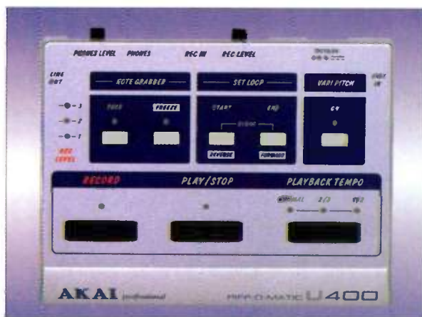
FIG. 1: The Akai U400 Riff-O-Matic packs several great features into a compact, die-cast aluminum box.
