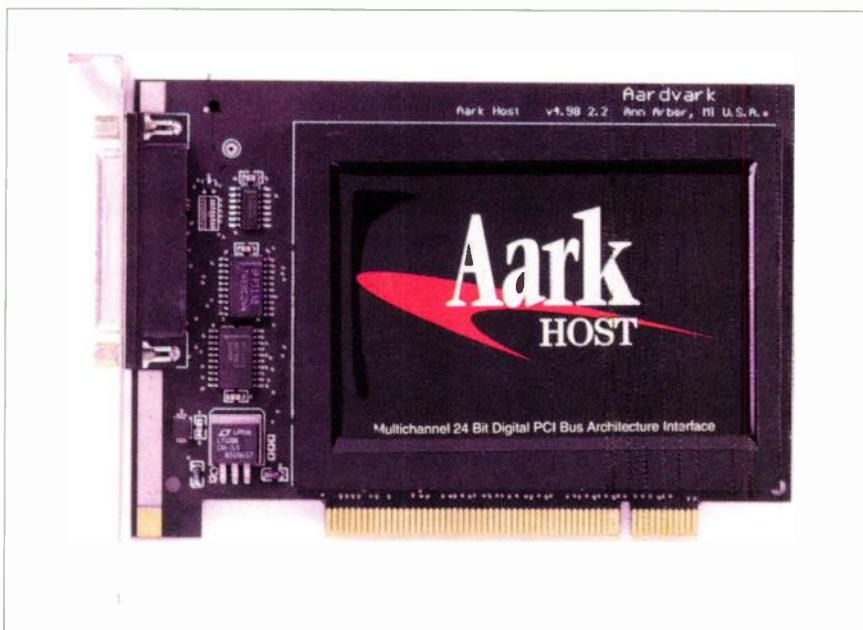
FIG. 1: The circuitry of the Aark 20/20+ PCI host card is well shielded in a protective casing to reduce exposure to RF interference from within the computer.
