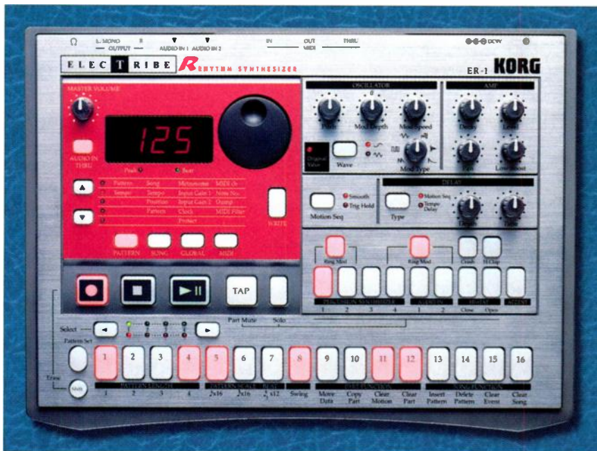
FIG. 1: Although the Electribe ER-1 certainly qualifies as a drum machine, it's more than just an old-fashioned beatbox. Designed specifically for live performance of contemporary electronica/dance music, it is more like a real-time percussion synthesizer integrated with a loop-oriented pattern sequencer.
