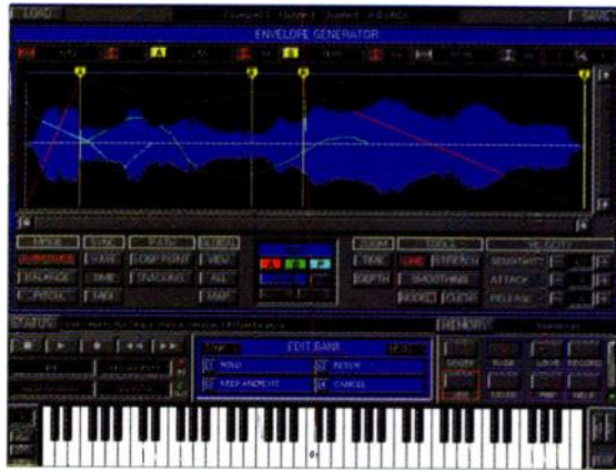
FIG. 4: The system's advanced envelope-editing capabilities allow you to create complex envelopes for pitch, panning, and amplitude.
