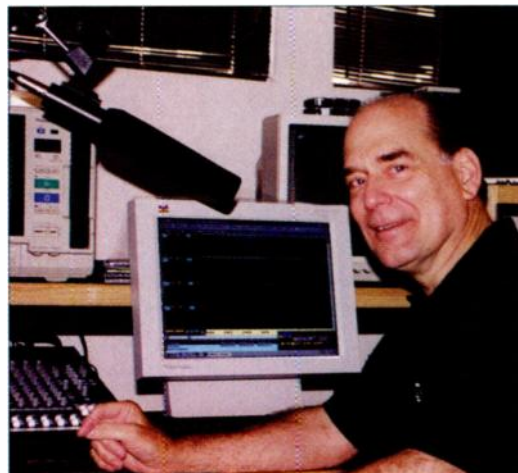
Don Elliot, house voice for Los Angeles-based KFI AM and KOST FM, uses a PC running IQS Software Audio Workshop (SAW) as his primary recording and editing tool. His home studio includes JBL 4411 monitor speakers, a Sennheiser 416 microphone, and a Mackie 1604 VLZ compact mixer.
