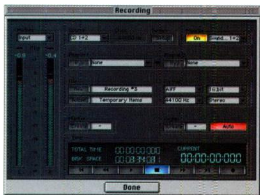
FIG. 2: Spark's Recording dialog box allows you to keep adding takes into the same file by automatically creating new regions.
