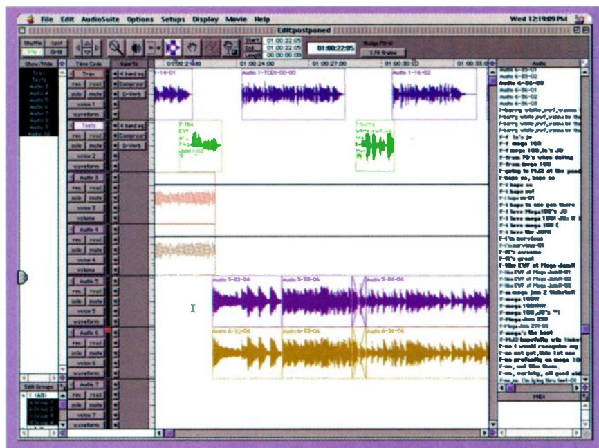
FIG. 1: Here is a good example of how the various tracks of a radio spot are typically organized: VOs on tracks 1 and 2, in addition to two stereo music beds. Note the crossfade in the middle of tracks 5 and 6. This provides a smoother transition from one music segment to another.
