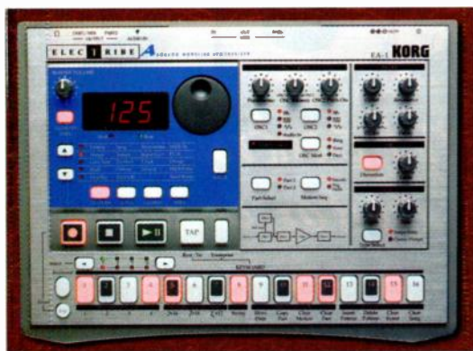
FIG. 3: The EA-1 uses physical modeling to emulate some of the simpler classic analog synthesizers. Like the ER-1, it is aimed at the live dance/electronica market and integrates a real-time synth with a loop-oriented pattern sequencer.
