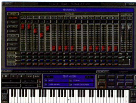
FIG. 5: Space Station Pro's Main Mixer gives you volume, pan, attack, and release controls for each MIDI channel. The faders can be grouped to prevent cumbersome mouse movements.
