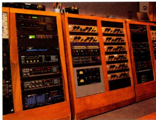
FIG. 1: The equipment racks at Loud Studio are well appointed with premium vintage gear. Note the Fairchild Limiter (the giant, dual-channel box) and eight Pultec EQP-1A3 program equalizers.
