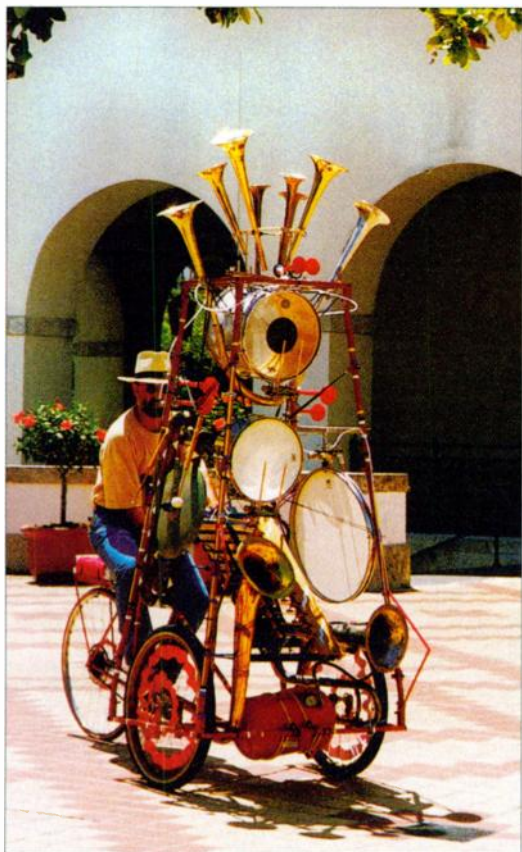
FIG. 2: Trimpin built six customized tricycle rickshaws equipped with automatically operated musical instruments for his Miami Klangflotte . Each tricycle receives messages via a wireless MIDI system, allowing the entire group to play in sync.
