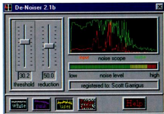
FIG. 4: Using the noise-print method, the De-Noiser plug-in lets you remove continuous background noises such as hiss.
