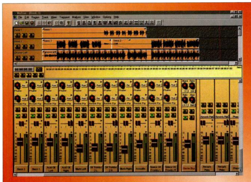
FIG. 1: The main workspace in MxTrax provides a split-screen view, with multiple waveform displays on top and a customizable mixer section below.
