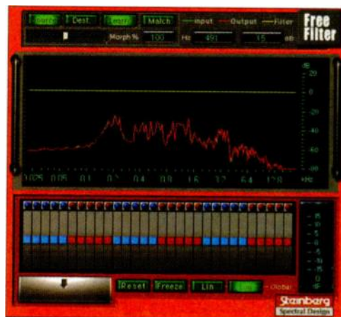
FIG. 1: Steinberg’s FreeFilter can provide you with a detailed spectral analysis. The logarithmic display shown here is especially useful when tweaking the high end of the spectrum.
