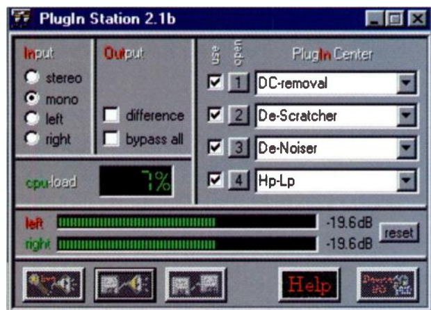
FIG. 1: The PlugIn Station is the command center where you choose what type of processing to use and define the plug-in chain.
