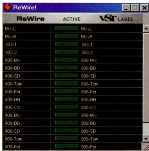
FIG. 2: Steinberg's ReWire allows the audio output of a program to appear inside a Cubase VST mixer. Here, the individual drum sounds of Steinberg's ReBirth application are shown inside Cubase .
