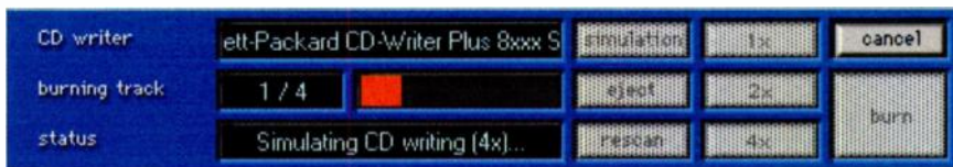
FIG. 3: Clean's CD-burning dialog box contains all of the controls for putting audio tracks on CD-R.
