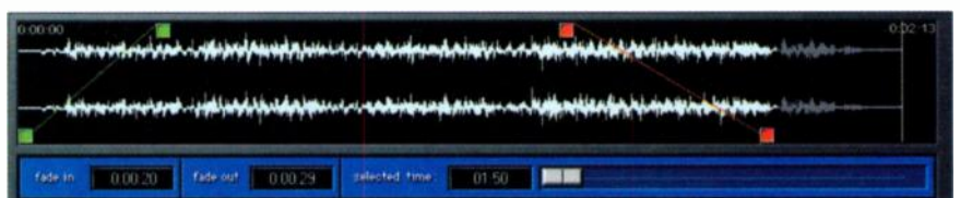
FIG. 2: You can draw Fade In and Fade Out markers directly on the waveform to specify beginning and ending volume fades for the current track. A time display shows the lengths of the fades in hours, minutes, and seconds.
