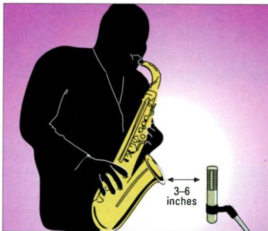
FIG. 2: You can attenuate the bristling highs of an alto sax by positioning the diaphragm of the mic partially beneath the lip of the bell.
