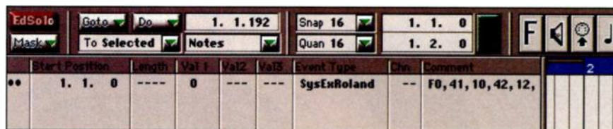
FIG. 5: Here's an example of the code used to circumvent the GM drum default.
