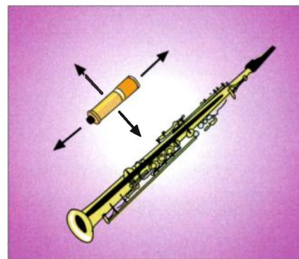
FIG. 1: A single, large-diaphragm condenser mic, preferably a tube model, can be located to capture a balanced image of soprano sax. Move the microphone toward the mouthpiece to accentuate highs, and toward the bell to increase "honk" and cutting power. You can bring the mic closer to the instrument to emphasize warmth and midrange or pull it back to provide a more open, natural sound.
