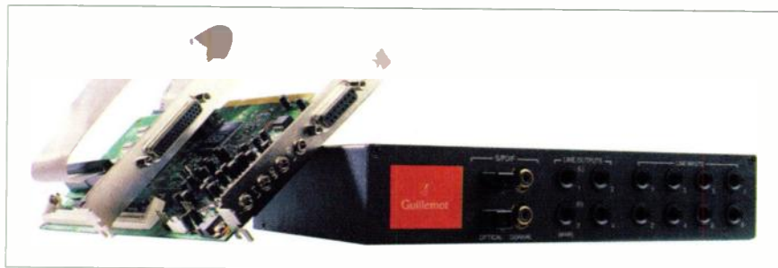
The Guillemot Maxi Studio ISIS is a well-equipped sound card with multiple analog and digital I/O options. An audio interface keeps the system's converters outside of the computer, and a game mode provides DSP processing for those moments when busy musicians just want to relax a bit.
