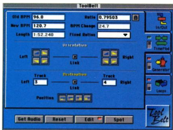
FIG. 3: The TimeMod page provides time compression and expansion based on various parameters. In this example, the ratio is specified in bpm.
