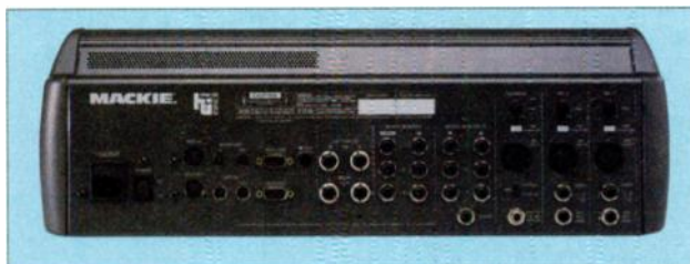
FIG. 2: In addition to its numerous audio inputs and outputs, the HUI is laden with control ports. Along with its MIDI ports, it has Relay outputs for toggling electrical switches, and ADB extension ports so you can keep your Mac keyboard near the Mackie control surface. Another 9-pin jack is supplied for future external control devices. The RS-232/422 port is provided for connecting to a digital audio workstation, but many DAWs are not compatible with it.
