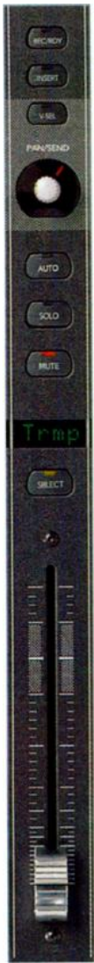
FIG. 1: The HUI channel strip includes many common features. But the Pan/Send knob is actually a V-Pot, a programmable control that lets you set Pro Tools I/O assignments and send destinations. You set its function with the V-Sel switch. The Insert switch calls up inserts for editing and aids in accessing Pro Tools plug-ins. The Scribble Strip (above the channel-select button) lets you label channels, but only with four characters.
