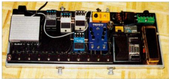
FIG. 2: By creating a pedalboard with a dedicated power supply (left) and true bypass circuits (row of buttons at the bottom), you can maximize the efficiency of your pedal setup. This custom pedalboard was designed by Tom Peck of Pedalboards.com.
