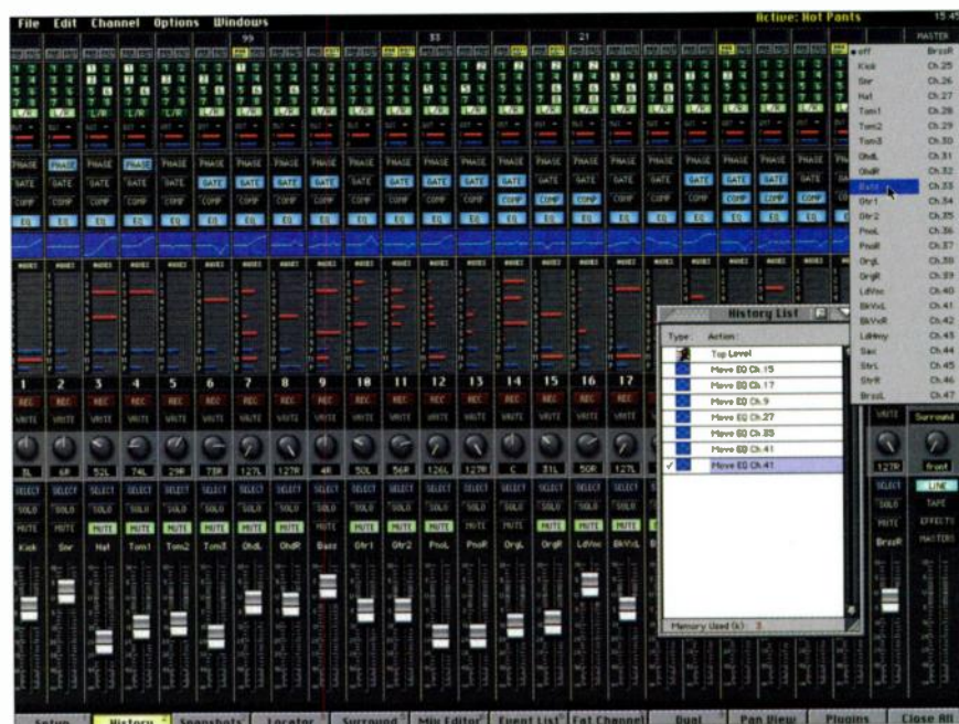
FIG. 2: Using the D8B's remote CPU, you can install a monitor, keyboard, and mouse, and control your mixes onscreen. This screen is from the recently released OS version 3, which adds inserts and cross-patching.
