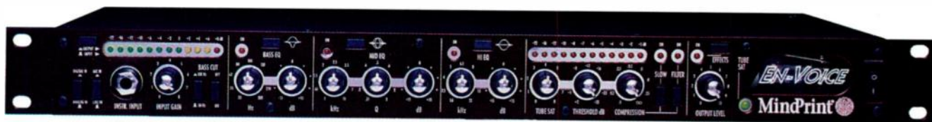
The En-Voice's preamp, equalizer, and tube compressor sections offer a wealth of tone-shaping options.
