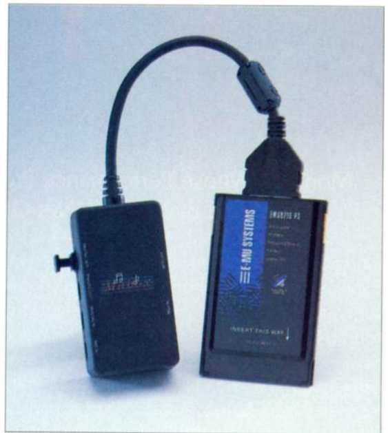
FIG. 4: E-mu's powerful EMU810ps PC Card combines analog audio I/O, S/PDIF output, MIDI I/O, wavetable ROM, and SoundFont samples in a PCMCIA card for laptop music production.
