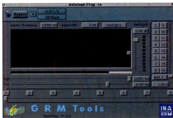
FIG. 2: Apply GRM Tools' Band Pass plug-in to pitched, sustained material and drag the control cursor around the outer edge of the black "work area" to create a descending overtone sweep.
