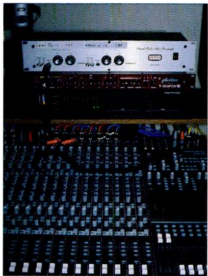
Two of my favorite boxes for warming up digital signals are the Rolls RP220 Dual Tube Mic Preamp and the MindPrint En-Voice voice processor.
