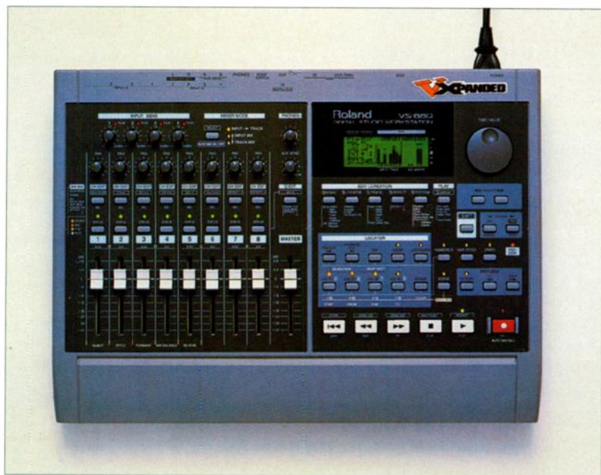
FIG. 3: The powerful recording and editing features of the VS-880 are accessed by using button combinations and the data wheel.
