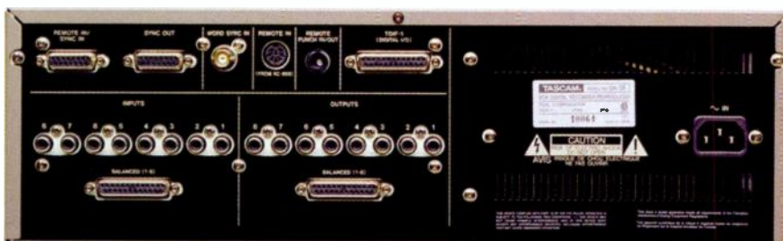
FIG. 2: The analog I/O options of the Tascam DA-38 include RCA jacks for unbalanced signals and 25-pin D-sub connectors for balanced signals. Digital I/O is via the TDI/F interface.
