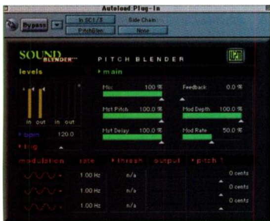
FIG. 4: Try placing a plug-in such as PitchBlender from WaveMechanics across the reverb returns to process the reverb signal.
