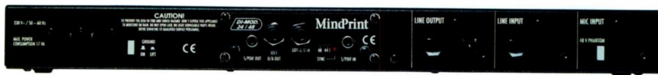
FIG. 1: With the exception of the \frac{1}{4} -inch instrument input, all connections are made through the XLR and \frac{1}{4} -inch TRS jacks on the back panel.
