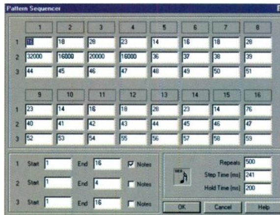
FIG. 2: Audio Architect's Sequencer is based on analog pattern-based sequencers and provides 16 steps for each of three channels. You can use this module to create numerous types of dynamically changing sounds.
