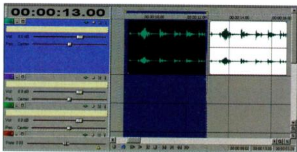
FIG. 4: To punch in, just highlight an event and then drag the Selection bar to the preroll and postroll points.
