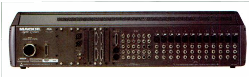
FIG. 1: Mic and line level connections are made via the D8B's rear panel. That's also the location of the card cage, where you can install optional I/O, effect, and sync cards.
