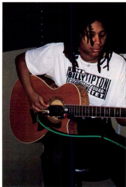
FIG. 1: Shelley Doty's Taylor 612-C guitar is miked with a stereo pair of GT Electronics AM30 microphones. (The other mic is off-camera to the left.)
