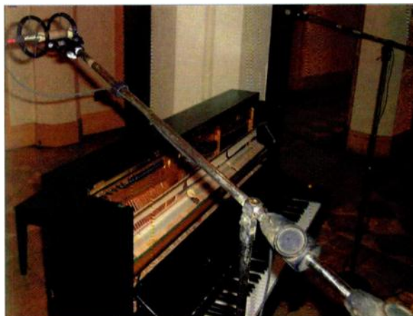
FIG. 5: A pair of small-diaphragm cardioid condensers are pointed at each other, four to six inches from the edge of the opening and two to three feet above. Also try angling the mics downward 20 degrees or so.
