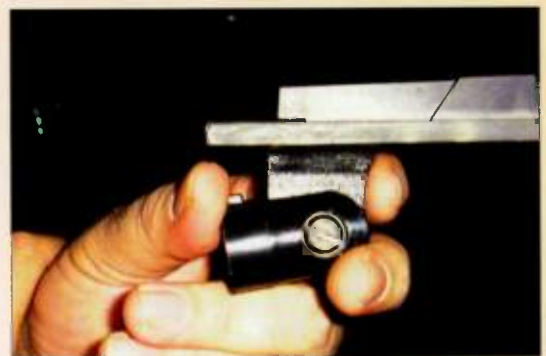
FIG. A: Mark Pinske holds up a modified Radio Shack Realistic PZM to show the all-important gap between the capsule and the boundary.
