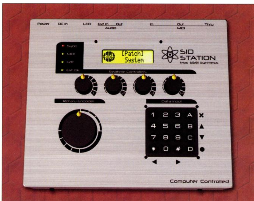
FIG. 1: The futuristic-looking SidStation has an astutely designed user interface. For example, the four user-definable control knobs reside above the data wheel and keypad.
