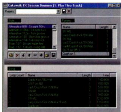
FIG. 5: Use the Session Drummer to assemble MIDI drum tracks by selecting Patterns from Styles and combining them into a Song.
