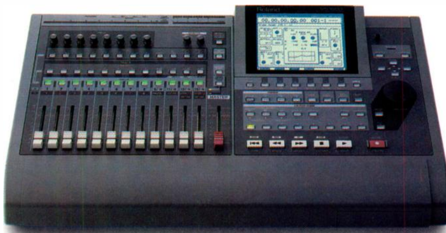
Bouncing with effects frees up the Roland VS-1680's processors for use on other tracks.
