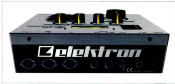
FIG. 2: The SidStation's back panel features MIDI In, Out, and Thru connectors, an audio input and output, a DC input, and a knob to adjust the LCD contrast.
