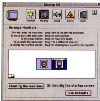
FIG. 5: The Monitors & Sound control panel lets you tell your Mac how you want your displays arranged. Simply click on the Arrange button and drag the monitor icons into position.
