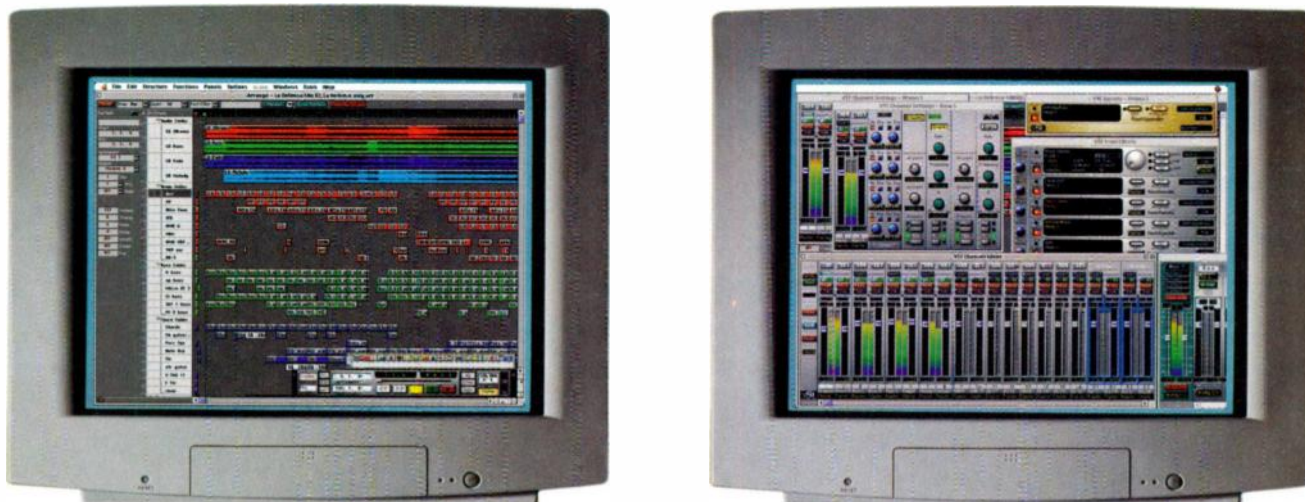
FIG. 3: A sophisticated digital audio sequencer such as Cubase VST can easily fill two monitors. If you move the Mixer view and the various other VST views to the right, you can devote the left screen to the Arrange window.
