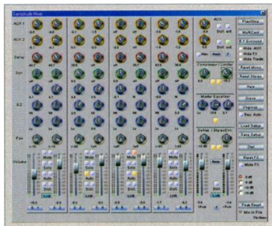
FIG. 13: The Mixer screen in Samplitude 2496 is not only very slick, but very functional. Real-time adjustment is possible, even on multiple tracks simultaneously.
