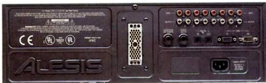
FIG. 4: As you might expect, the Alesis ADAT XT20 includes ADAT Optical connectors.
