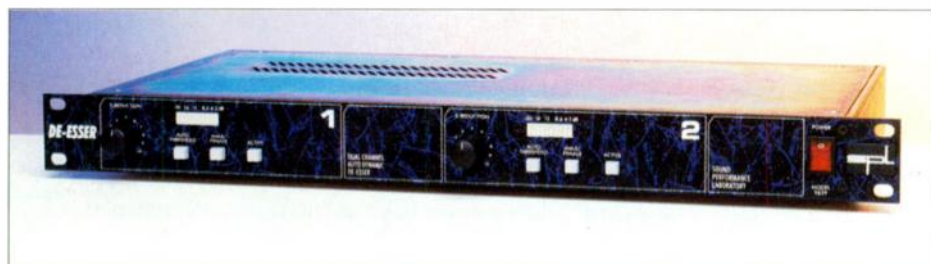
The SPL Model 9629 Dual Channel Auto Dynamic De-Esser parts company with conventional de-essers, employing a special circuit that scans the signal for esses and then reduces them by feeding a phase-inverted signal of the unwanted frequencies back into the signal path.
