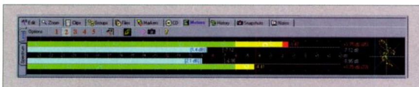
FIG. 10: WaveLab offers a set of sophisticated VU/peak-hold meters (with numerical readouts) as well as a handy Phase meter on the right.
