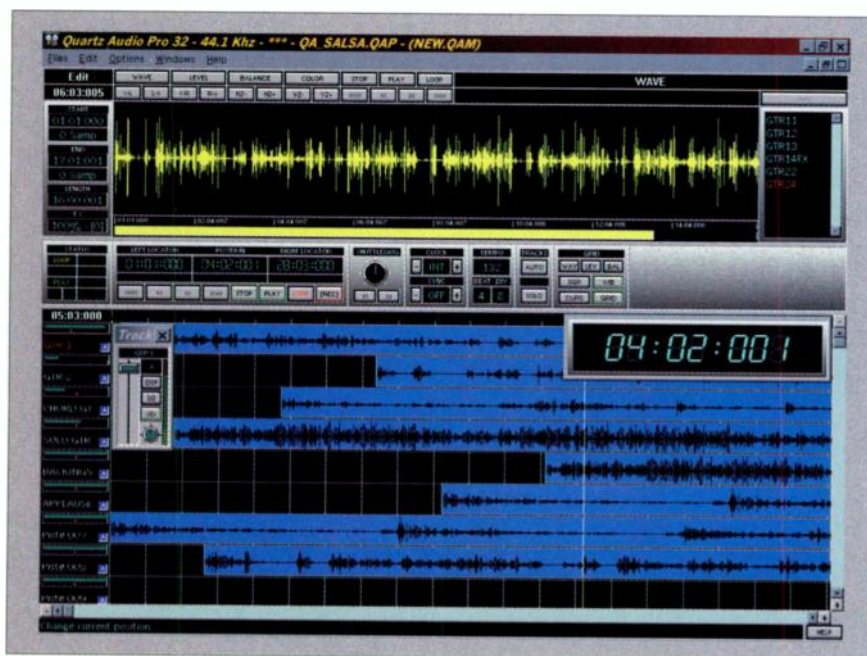
FIG. 3: The main screen in Quartz Audio Pro 32 includes the Mixing Grid in the lower part, a set of transport controls in the middle, and a changeable display at the top. The Edit Elements display (shown here at the top) lets you import and edit audio files before adding them to the mix.
