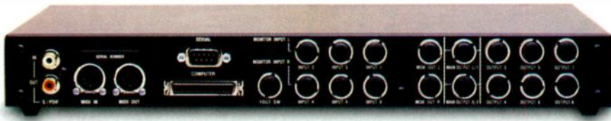
FIG. 2: The rear panel features MIDI In and Out, RCA S/PDIF I/O, six balanced TRS inputs, two Main and two Monitor outputs on balanced TRS jacks at +4 dBV, and six unbalanced outputs at -10 dBu.
