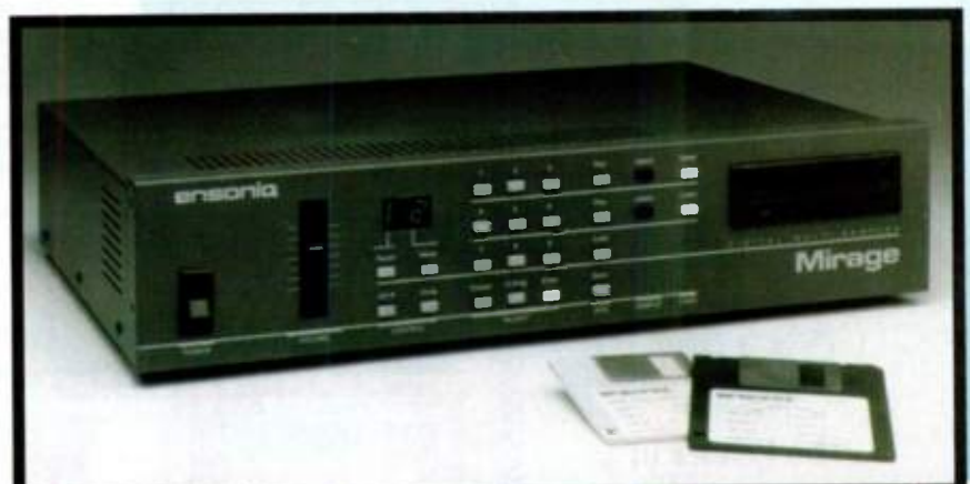
FIG. 2: Among the earliest digital samplers was the Ensoniq Mirage. It was supported by numerous third-party manufacturers that offered both hardware accessories and software enhancements.
