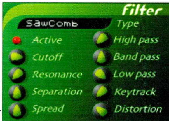
FIG. 2: Vibra9000 's Filter window contains a menu of the various filter selections. I've selected the Saw Comb filter, with no highpass output, medium bandpass output, maximum lowpass output, and a bit of distortion.
