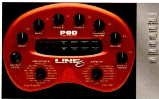
FIG. 1: Cakewalk Pro Audio 9 provides tools for building custom templates to be used with external MIDI and audio gear. The panel shown here is a preset template for use with the Line 6 Pod.
