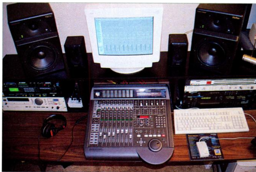
FIG. 4: Teaming a physical control surface, a digital audio sequencer, and an audio patch bay makes for a very strong combo. The author's mixing station, complete with a HUI, Pro Tools, and a PM-216 patch bay, is shown here.
