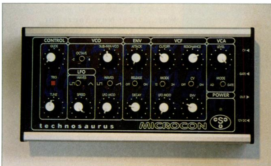
FIG. 1: The controls on the front panel of the Technosaurus Microcon are well placed, with 12 knobs and 7 switches fitting into its tiny footprint.
