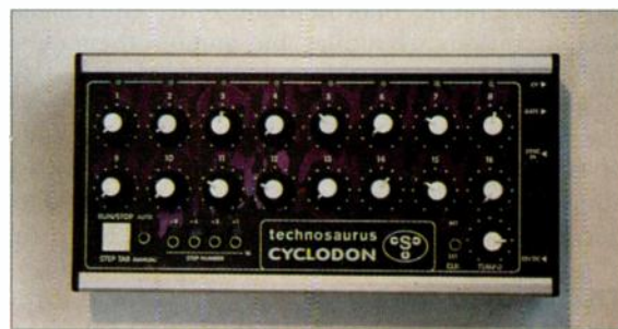
FIG. 2: The Cyclodon allows you to change the number of steps in the sequence in real time.
