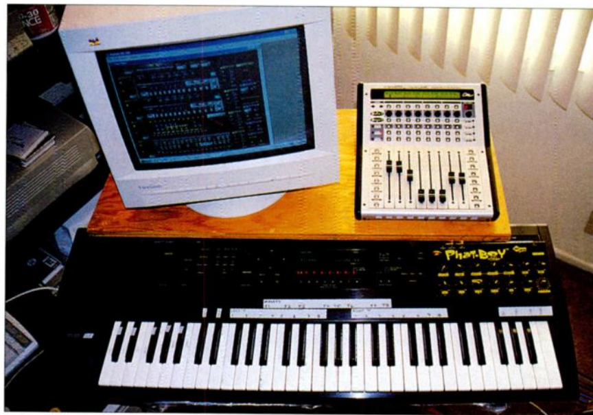
FIG. 3: Among the various MIDI control surfaces on the market today, the keyboard is often overlooked as a resource. Here, the keyboard sits near the Keyfax PhatBoy and the CM Automation MotorMix. Tape strips are handy reminders of the controller maps I've assigned to the keys.
