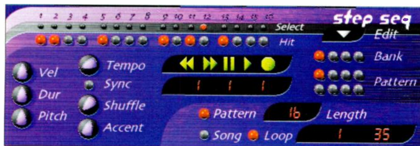
FIG. 4: In Gamma's Step Sequence section, you enter beats with the Hit buttons and activate accent, velocity, duration, and pitch with the Select buttons.
