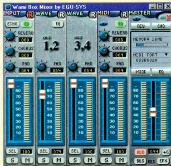
FIG. A: The Mixer applet in Ego Systems' WaMi Box controls the input and output levels and also provides hardware-based chorus and reverb. The Box offers two audio inputs, four audio outputs, and 16 channels each of internal and external MIDI.
