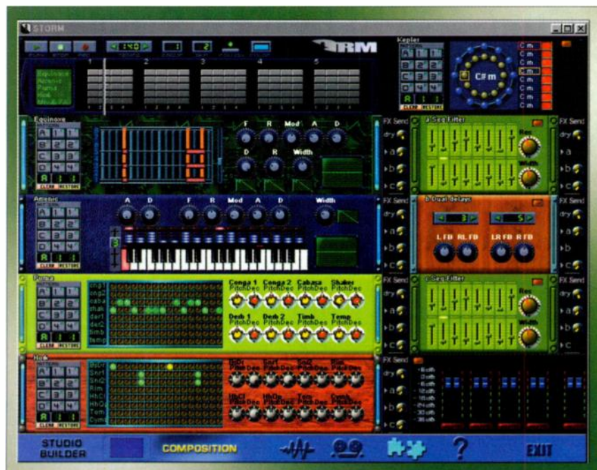
FIG. 6: The main interface in Arturia's Storm resembles a rack full of gear, including synths, effects, a mixer, and a sequencer. All of the devices sync to a global clock.
