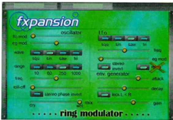
FIG. 3: Ring Modulator's LFO and Envelope Generator can each be fed one of four typical synthesizer waveforms. A virtual LED indicates the selected waveform.
