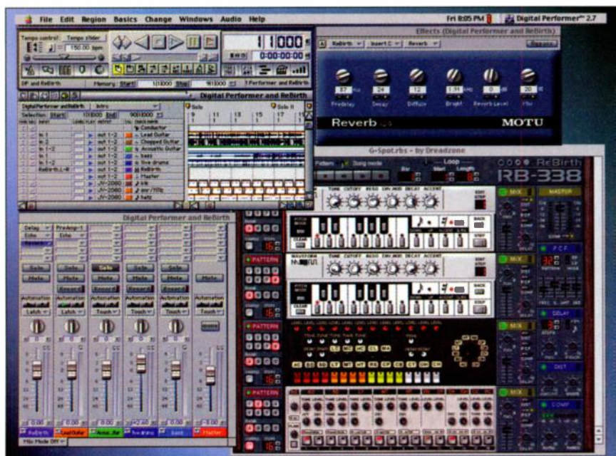
FIG. 1: Using ReWire technology, ReBirth can stream 24-bit audio directly into the mixer of Mark of the Unicorn's Digital Performer .
