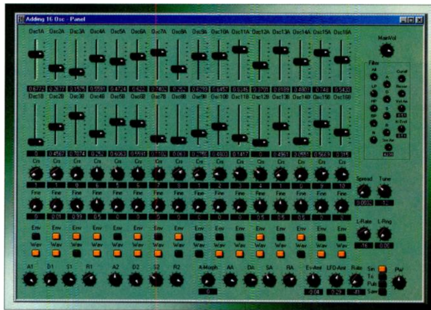
FIG. 2: Reaktor provides dozens of modules with which you can build elaborate synth designs. The synth pictured here uses additive synthesis with filters and envelopes to create sound.
