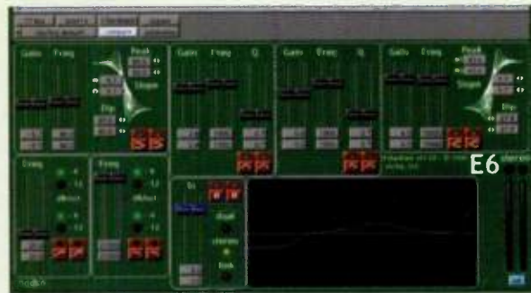
Filterbank , by McDSP, allows you to create your own stereo or mono EQ plug-in using up to six bands.
