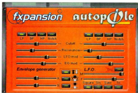
FIG. 2: AutopOle uses many of the sound-shaping tools found in synthesizers. The routing-switch buttons in the bottom center of the display control the configuration of the two filters.
