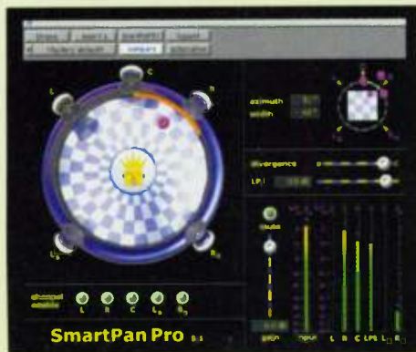
SmartPan Pro , by Kind of Loud Technologies, allows you to precisely position audio elements within an LCRS, 5.1, or 7.1 surround mix.
