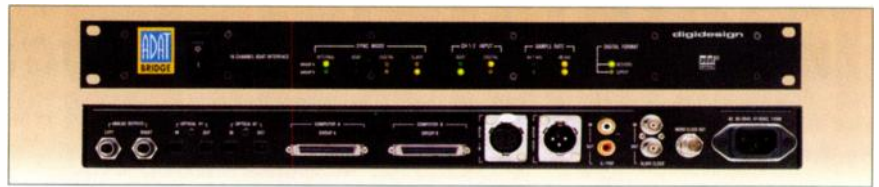
FIG. 3: The ADAT Bridge I/O gives you a number of interface options, including S/PDIF, AES/EBU, Lightpipe, and slave clock I/O. Analog and word clock outputs are also included.
