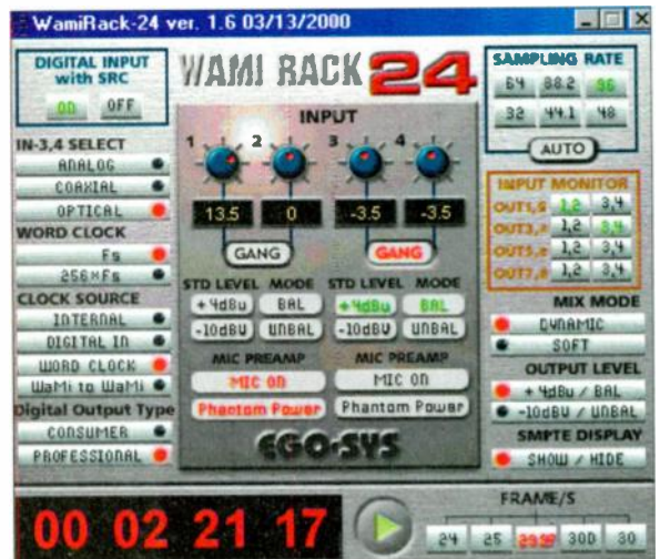
FIG. 2: Control Desk provides access to all of the WaMi's settings, from output level to mic preamps and phantom power. The sample rate can be set manually or automatically, and each pair of inputs can be monitored in real time through any pair of outputs.
