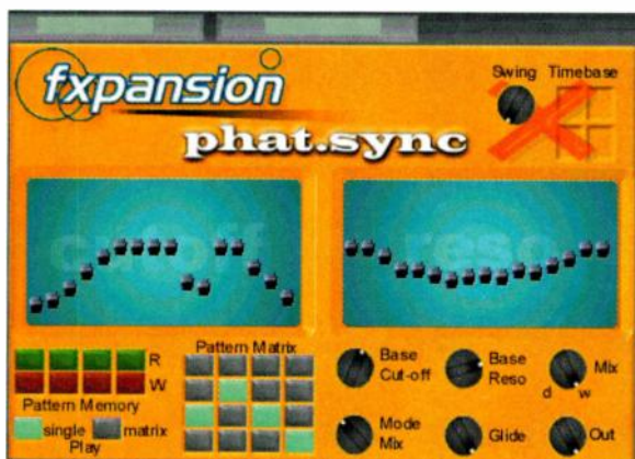
FIG. 1: Using PhatSync 's Pattern Matrix, you can switch from one frequency-and-resonance setting to another either by clicking on a button or sending MIDI messages from your sequencer.
