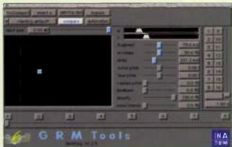
The Shuffler , from the GRM Tools, vol. 1, bundle, randomly slices an audio file into small parts and reassembles it according to user definitions.
