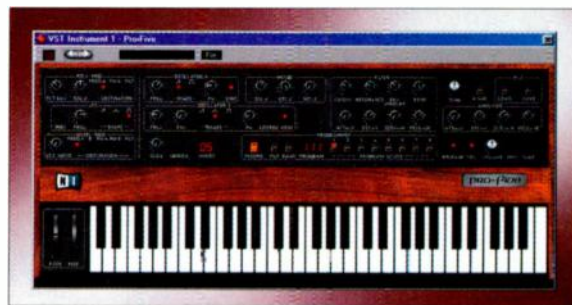
FIG. 11: Pro-Five is a virtual version of Sequential Circuits' Prophet-5 with a number of digital enhancements. It offers up to 32-note polyphony and has a keyboard that can be toggled on and off.
