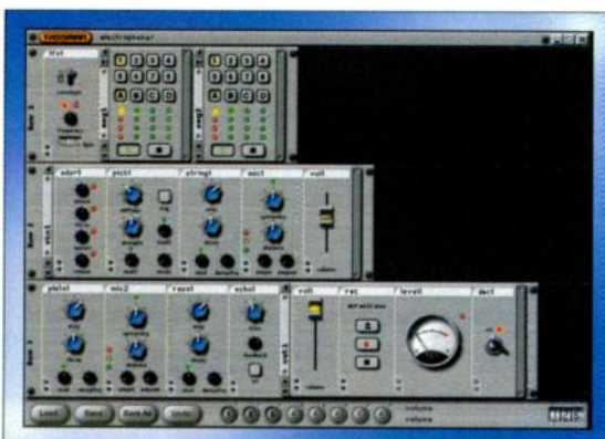
FIG. 1: Tassman offers a number of physical models among its many synth modules. Pictured here is a synth that contains a pick, string, and metal plate, as well as a sequencer and several modulation sources.
