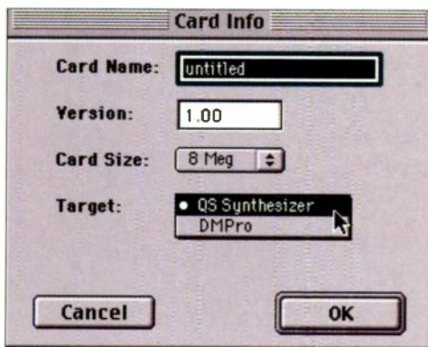
FIG. 1: The Card Info window lets the user customize the name of the card and assign a version number. Entering the size of the card will allow you to keep tabs on remaining memory.
