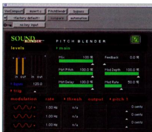
The powerful SoundBlender , by Wave Mechanics, lets you combine a variety of effects—including delays and filters—using a modulation matrix.
