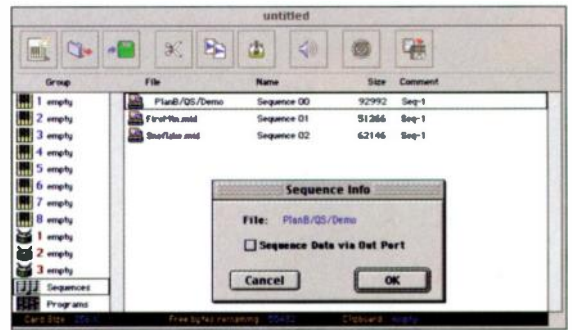
FIG. 4: The Sequence Info window allows you to choose if the MIDI data will be played on the QS or external MIDI devices.
