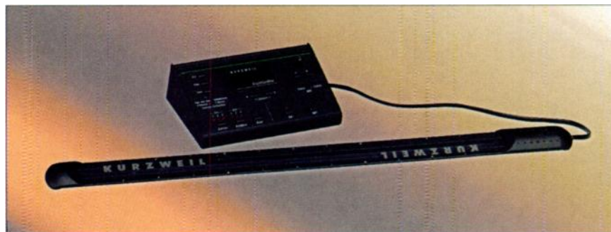
FIG. 2: More than just a ribbon controller, the Kurzweil ExpressionMate can send Note On and a variety of controller messages.
