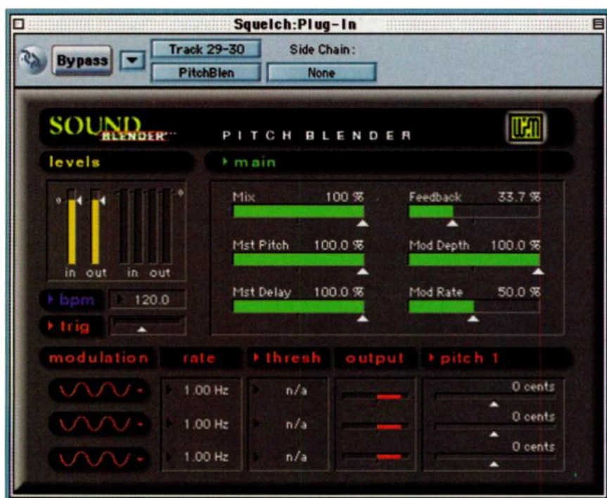
FIG. 1: PitchBlender's Main page provides controls for setting levels (on the left), six parameter sliders (in the center), and a Modulation area (at the bottom).
