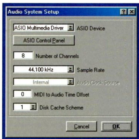
FIG. 2: The Audio System Setup dialog box appears when you run Cubasis VST for the first time. Here you access your sound card's control settings, specify the default audio channels and sample rate, and select the disk-caching scheme associated with your intended audio-production method.
