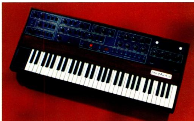
The Prophet-5 from Sequential Circuits was the first microprocessor-based programmable polyphonic synthesizer.
