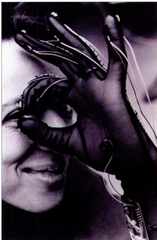
FIG. 5: Laetitia Sonami's Lady's Glove includes sensors that detect the distance between the glove and the floor.
