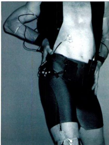
FIG. 6: The BodySynth can track up to 12 EMG sensors simultaneously for translating muscle movement into MIDI data.
