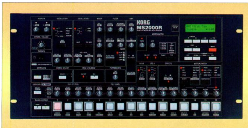
The Korg MS2000R (shown here) and MS2000 digitally model the behavior of analog synthesizers and provide lots of knobs and buttons, just like an analog synth.
