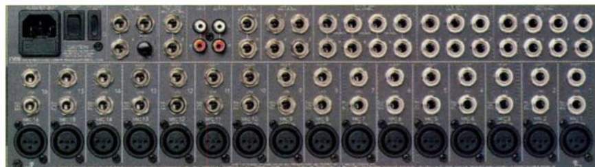
FIG. 1: The 1604-VLZ Pro offers 16 XLR inputs with phantom power, TRS inputs, stereo RCA tape inputs and outputs, and direct outs on channels 1 through 8.
