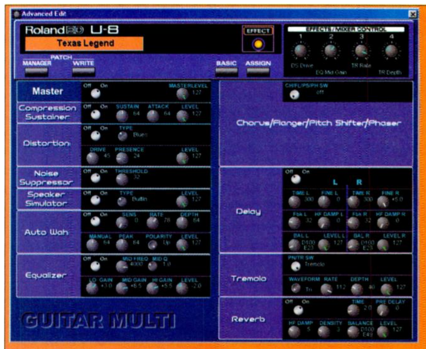
FIG. 3: In the Effects Edit window's Advanced Edit section, you control hardware effects in one of five multi-effect configurations. Clicking on the Patch Manager button takes you to the factory and user presets.
