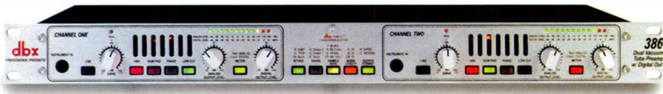
FIG. 1: The dbx 386 dual-channel analog tube preamp offers a truckload of features, including a pad, a low-cut filter, phantom power, and an instrument input for each channel. Among its major features are A/D converters that support two types of dither, two types of noise shaping, and up to 24-bit, 96 kHz conversion.
