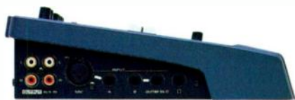
FIG. 1: The U-8's left side panel offers two unbalanced audio inputs. Input A functions in mic- or line-level mode; input B in line-level or high-impedance guitar mode.
