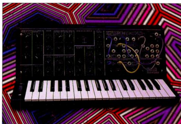
Korg's MS-20 analog mono synth has several cool features, such as a ring modulator, sample-and-hold, footpedal filter control, and pitch-to-voltage control. But its most popular feature is its patch bay.
