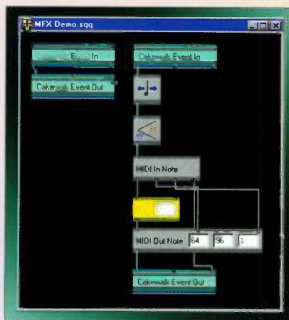
FIG. A: You can use Infinity to build Cakewalk MFX plug-ins. In this example, notes progress from Cakewalk Event In (on the right) to the MIDI Processors, which transpose them and alter their Velocity. The MIDI In Note Object then parses the data to add 7 semitones. Finally, the MIDI message is reassembled in the MIDI Out Note Object and returned to the sequencer's control.
