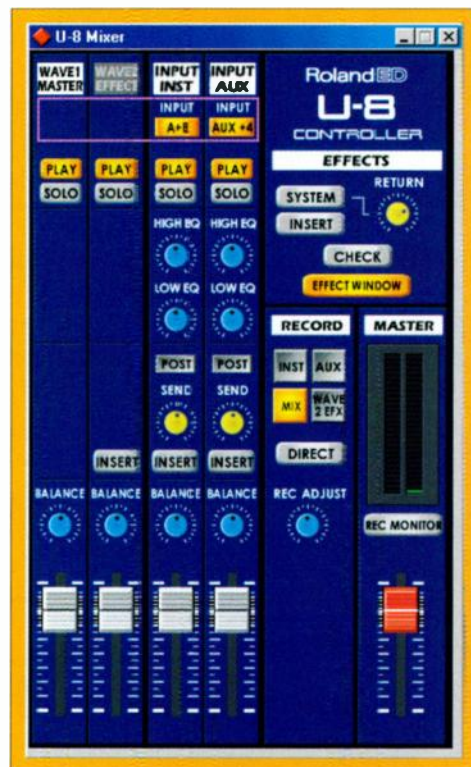
FIG. 2: The U-8 Mixer is a simple but powerful mixer applet that controls audio routing for the U-8. The Record buttons select the recording source; the Input buttons select input types. You can apply effects during recording or simply monitor them while you're recording dry.
