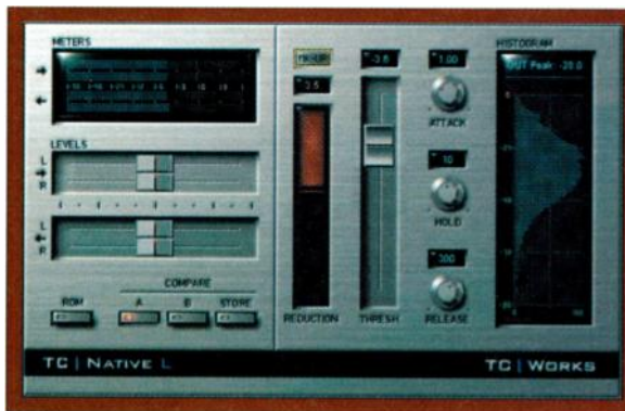
TC Works' TC Native Bundle 2.0 retains the three plug-ins found in version 1.0 and adds TC Native L , a single-band limiter with automatic makeup gain and a histogram tool.
