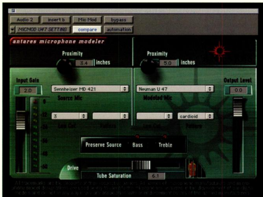
FIG. 1: The Antares Microphone Modeler gives you the opportunity to create a hybrid of two mics with the Preserve Source buttons.
