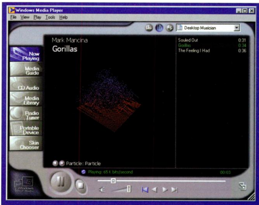
FIG. 3: Version 7 of the Windows Media Player features playlists and file management along with the ability to "rip" files directly from CD to WMA format. Along with direct links to Microsoft's online media guide, it offers facilities for loading WMA files into portable players.
