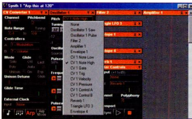
FIG. 3: Assigning an input signal to a module proves as simple as clicking on a parameter, then choosing from a list of sources. Available inputs for the Oscillator module are shown here.
