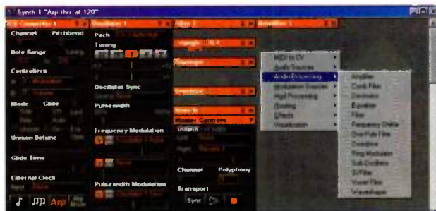
FIG. 2: The VAZ Modular interface avoids clutter by allowing you to "roll-up" each module so that only its name appears. It also uses an efficient menu system for picking the various modules you'll use in your synth designs.
