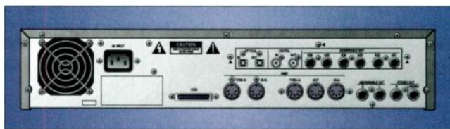
FIG. 2: The A5000 has two MIDI In ports for reception on up to 32 MIDI channels. The AIEB1 expansion board provides six additional analog outputs along with optical and coaxial S/PDIF I/O.
