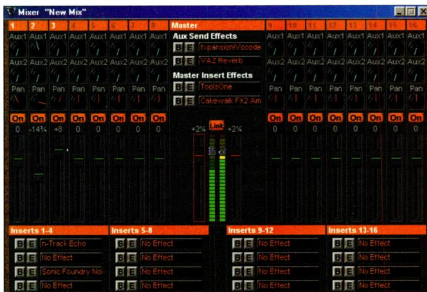
FIG. 1: The Mixer window in VAZ Modular is the first step for creating new Synth designs. It also provides access to the Aux, Insert, and Master effects.
