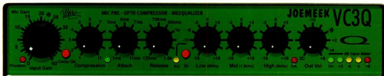
FIG. 1: The Pro Channel VC3Q combines a mic preamp, a photo-optical compressor, and 3-band EQ in a half-rack unit.
