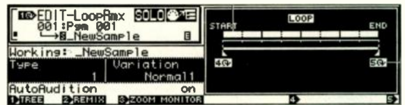
FIG. 4: The Loop Remix feature divides loops into segments and randomly reorders them. You can also save successful remix algorithms for later use.
