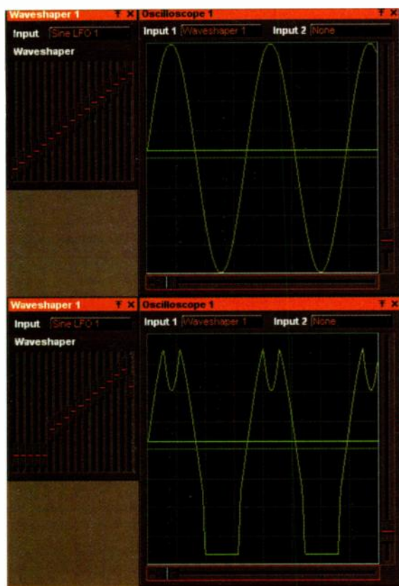
FIG. 4: The Waveshaper module is used to modify the harmonic content of an audio source. Here, a linear transfer function (top left) produces no change to the output sine waveform (top right), while a nonlinear curve (bottom left) alters the waveform to produce clipping (bottom right).
