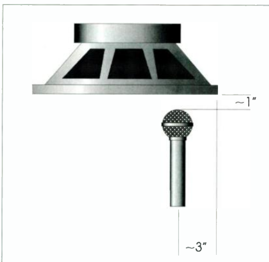
FIG. 3: The typical way to mic an electric-guitar amp is to position the mic about 1 to 2 inches in front of the speaker, offset from the center of the cone.
