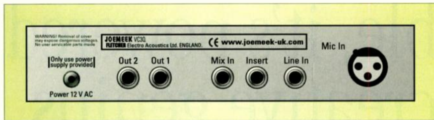
FIG. 2: Despite its diminutive size, the Pro Channel VC3Q provides dual outputs, a handy Insert, and more.
