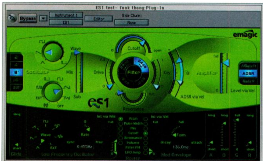
FIG. 1: From the ES1 's graphic interface, you can choose one of four lowpass filter types: 12 dB, 18 dB, 24 dB Classic, or 24 dB Fat.
