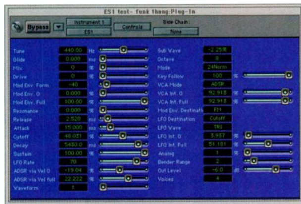
FIG. 2: The easy-to-read control screen includes five parameters not found on the graphic interface: Analog, Bend Range, Master Tuning, Voices, and Output Level.
