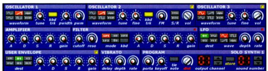
FIG. 1: Oscillator, Amplifier, Filter, LFO, User Envelope, Vibrato, and Program modules make up Dream Station's synthesis engine.
