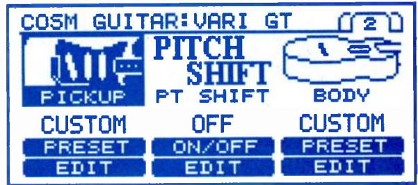
FIG. 3: Vari Guitar is the unit's most complex algorithm, offering control of pickup, tuning, and body parameters.
