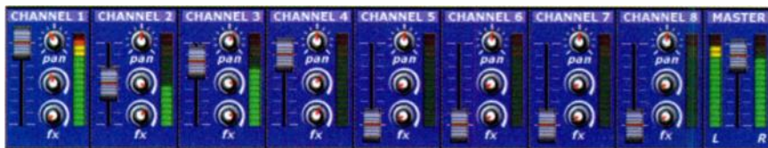
FIG. 4: The Mixer module is the last level of Dream Station's internal architecture. Programs can be assigned to any of the eight Mixer channels. These channels are then combined into one final stereo mix, which is sent to your sound-card output.
