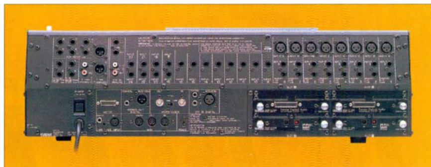
FIG. 4: The Yamaha 02R's rear panel sports six aux sends, studio and control-room monitor outputs, main stereo outputs on RCA and XLR connectors, 2-track analog inputs on \frac{1}{4} -inch TRS and RCA jacks, and 24 analog inputs. S/PDIF and AES/EBU digital I/O are provided. Other connections include word clock I/O, SMPTE and MIDI Time Code inputs, and MIDI In, Out, and Thru. You also get a meter-bridge port, a Mac (To Host) interface, and four I/O card slots.
