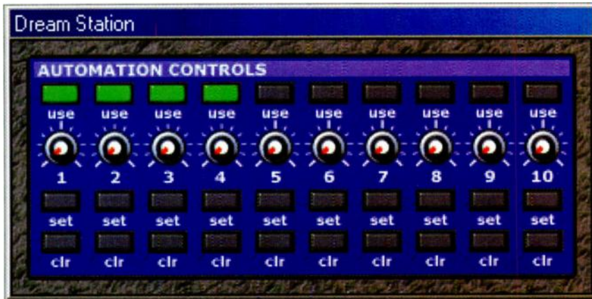
FIG. 3: The Automation Controls box lets you assign up to ten different automation controls to be recorded. You can assign the controls to any of the knobs on Dream Station's synth panel.
