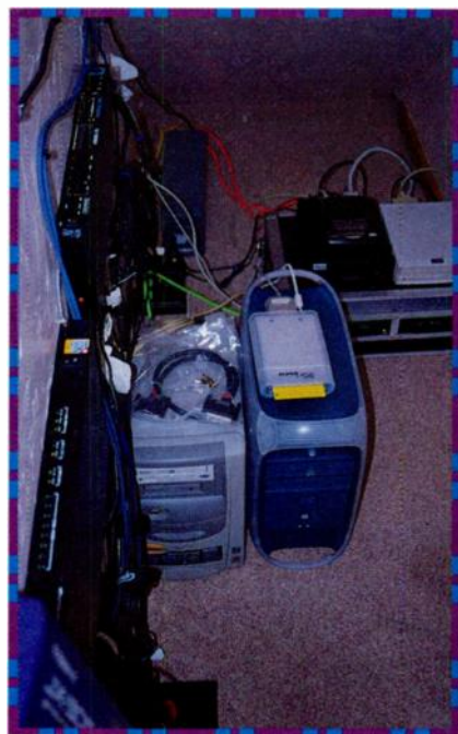
FIG. 1: A closet adjacent to the studio acts as a machine room, keeping equipment noise to a minimum. A hole drilled into the closet wall lets cables through. The computer sits on the floor, and several interfaces are bolted flat to the wall.
