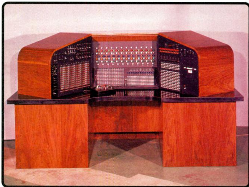
FIG. 5: This is the final version of the Raymond Scott Electronium, created for Berry Gordy of Motown. This “instantaneous composition/performance machine” was capable of playing highly complex music and is now owned by Mark Mothersbaugh.
