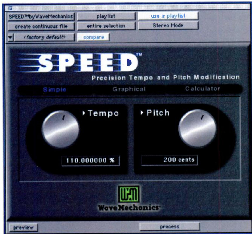
FIG. 1: Speed 's Simple control panel, one of the plug-in's several interfaces, has knobs for controlling a sample's pitch and tempo. The Preview feature is an excellent way to get an idea of how the processing will sound.
