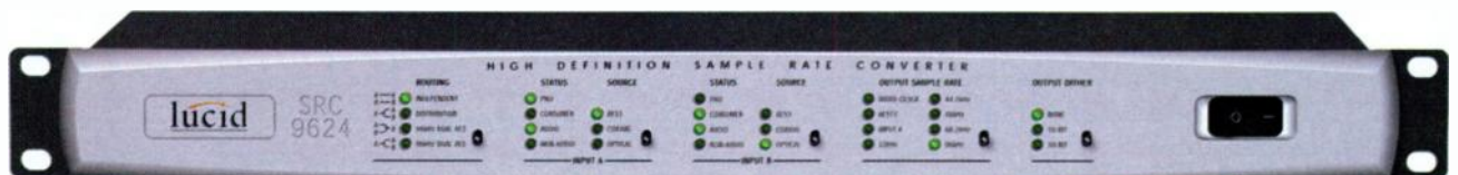
FIG. 1: Front-panel routing switches let the SRC9624 sample-rate converter work as a digital audio patch bay. Status lights indicate available signal types.
