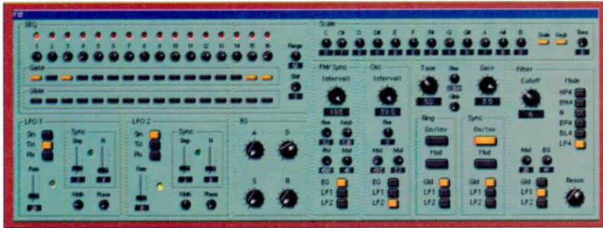
FIG. 2: The step sequencer in Dynamo's Cyclone Ensemble has a scale-correction stage in the upper right section of the Control Panel that makes it easy to create and transpose tonal sequences. The sequencer plays the compact hybrid FM synth in the lower right section of the Control Panel.
