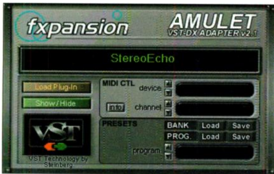
FXpansion's VST-DX Adapter software allows VST plug-ins to be used in DirectX-host applications.
