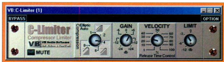
FIG. 3: C-Limiter essentially provides one function: limiting. Some basic compression features are included, but only as they relate to limiting. No attack-time or threshold parameter is provided.
