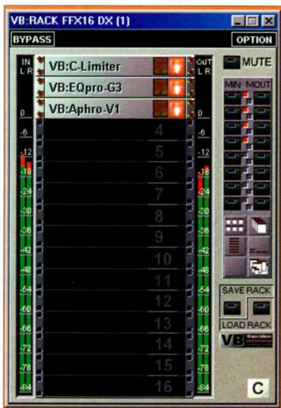
FIG. 1: FFX-16 lets you chain together any DirectX plug-ins to achieve multi-effects processing.
