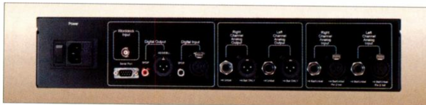
FIG. 2: The L2 Ultramaximizer is a professional unit all around. Analog I/O is +4 dBu and the signal is available from both digital outputs simultaneously.
