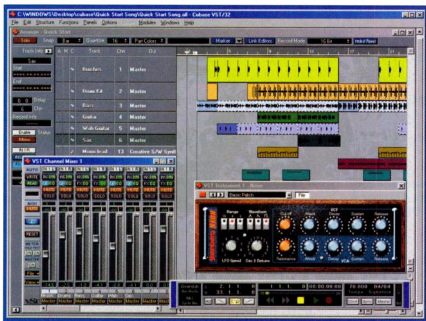
FIG. 1: Cubase VST/32 5.0 offers a redesigned user interface with many new features, including adjustable track sizes and new VST Instruments. You build compositions by combining individual clips of audio and MIDI data (called Parts) into Tracks to create Arrangements.
