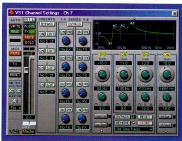
FIG. 4: You can adjust the EQ controls numerically or graphically by manipulating the EQ curve directly with your mouse.
