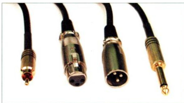
FIG. 2: From left to right, common audio-cable connectors include RCA (consumer and semipro unbalanced line cables), male and female XLR (microphone and balanced line cables), and 1/4-inch TS (unbalanced line and instrument cables).
