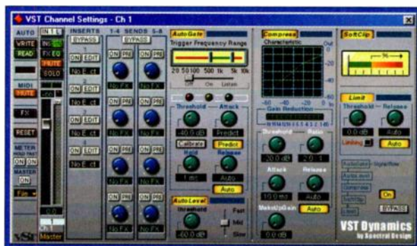
FIG. 3: Every audio channel in Cubase VST/32 provides a full set of dynamics processors: AutoGate, AutoLevel, Compress, SoftClip, and Limit.
