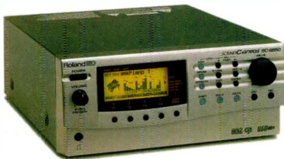
FIG. 7: Roland ED's SC-8850 Sound Canvas provides excellent-sounding GM1, GM2, and GS support, as well as USB connectivity.
