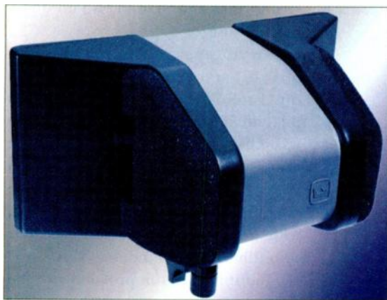
FIG. 2: A dedicated stereo microphone—such as Crown’s SASS-P Mk II, pictured above—can simplify the process of capturing a realistic stereo image. The Crown SASS (Stereo Ambient Sampling System) is a stereo PZM condenser that uses human-head-size spacing between its capsules to create a well-focused image without a “hole in the middle.”
