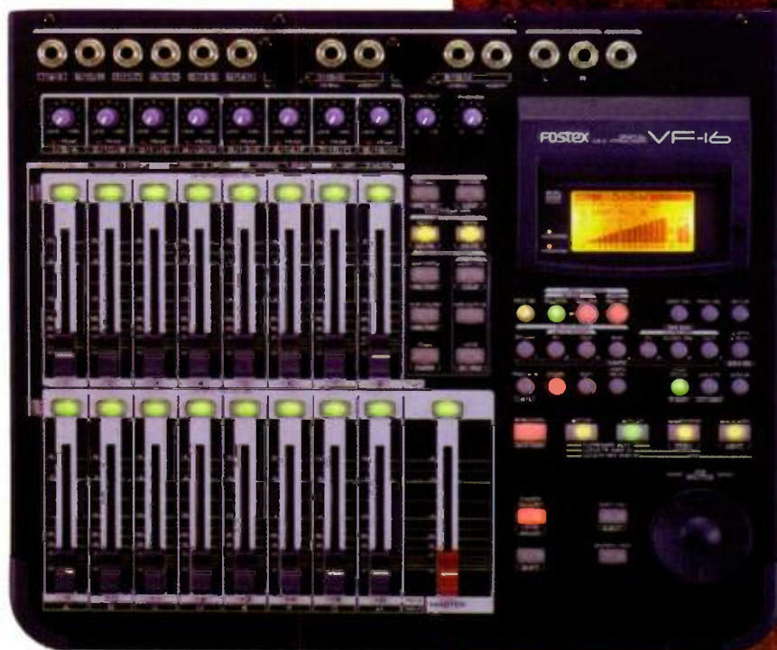
FIG. 1: The Fostex VF-16 digital multitracker offers eight analog inputs, including a pair of XLR mic inputs that you can swap with inputs 7 and 8. The VF-16 also has 16 channel faders, a graphic LCD, onboard effects and EQ, a jog/shuttle wheel, and upgradable hard drive capability.
