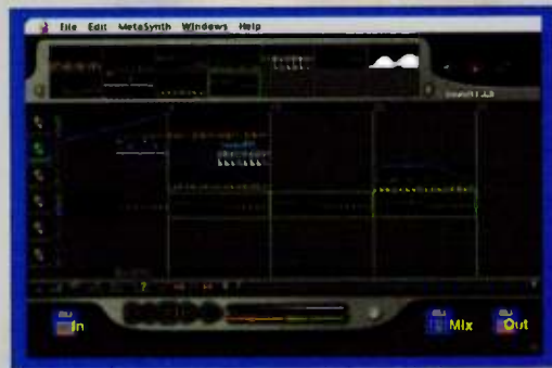
FIG. A: MetaTrack allows sound files from rendered MetaSynth presets to be arranged on separate audio tracks with independent pan, volume, insert effect, and fade curves. The top tab shows the presets in the preset library. Below it are displayed 6 of the 16 possible audio tracks.
