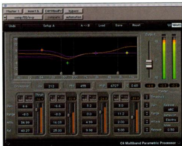
Waves' C4 can perform several processes at once. In this instance, it's being used to compress and boost the bass, compress and cut the low mids, boost the EQ of the high mids, and boost and expand the treble.
