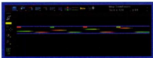
FIG. 7: MetaSynth's Note brush creates piano roll-style note sequences like the one shown here. The blue gridlines do not contribute to the sound. The color variation of the red/green lines represents panning, and the intensity variation represents volume.
