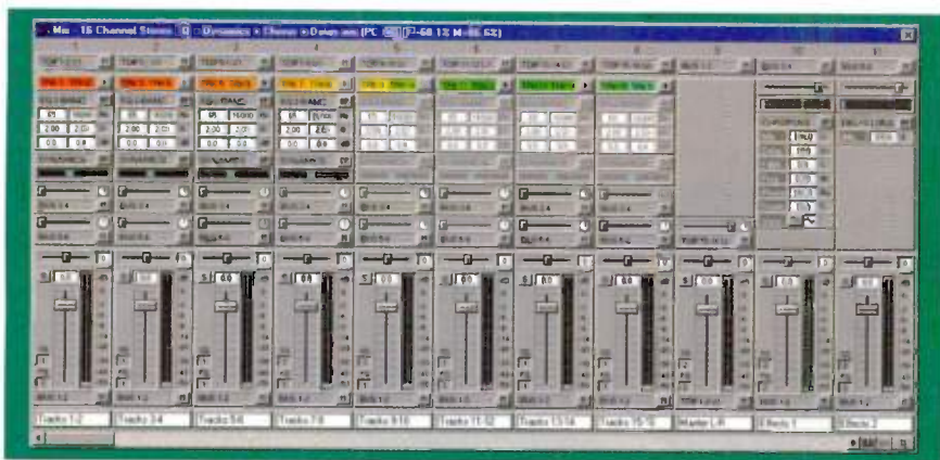
FIG. 2: The Mix window lets you route audio to the I/O connections, to the recording tracks, and to real-time effects. Sixteen internal mix buses are available.
