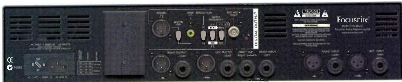
FIG. 2: In addition to the main XLR and 1/4-inch inputs, the MixMaster includes a pair of balanced auxiliary Direct Inputs.
