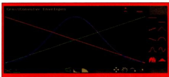
FIG. 6: The CrossConvolve window offers separate envelopes for the sound in the Sample Editor (green envelope), a sound file on disk (red envelope), and the cross convolution of the two (blue envelope).
