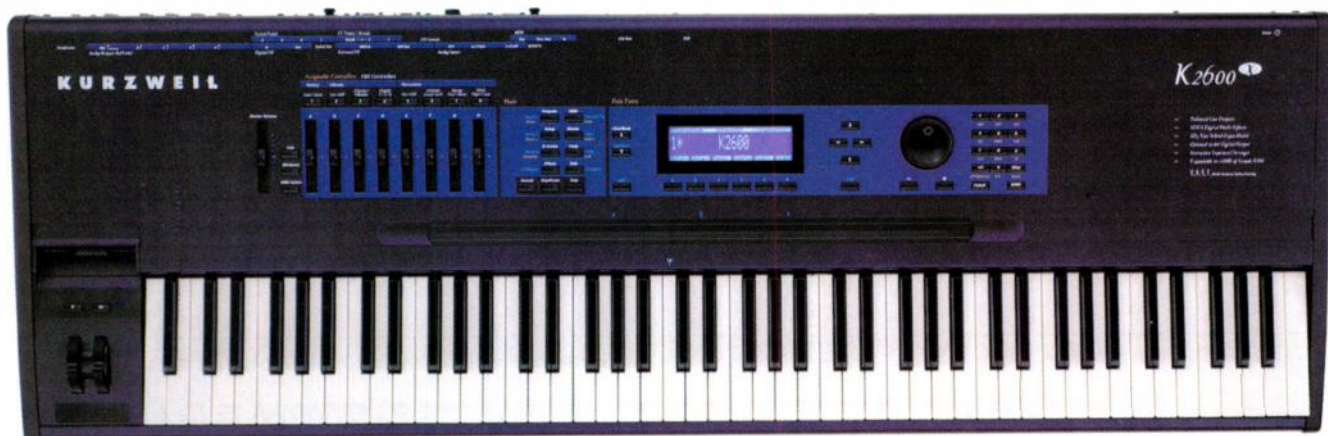
FIG. 1: The K2600's front panel hasn't changed much from the K2500 (except for the color). Prominent features include a long ribbon controller above the keyboard, a short ribbon controller below the pitch and mod wheels, two switch buttons above the wheels, eight assignable sliders, a large LCD with six soft buttons below it, a large data wheel, and an alphanumeric keypad in addition to various mode buttons.
