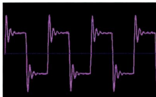
FIG. 8: By sending a square wave through a piece of audio gear and reading its output on an oscilloscope, you can see whether the circuit is ringing. If so, a ripple appears in the flat part of the waveform.
