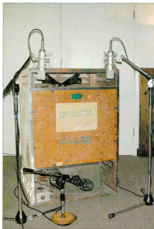
FIG. 4: A matched pair of Neumann U 87s captures a stereo image of the rotating treble-horn assembly while a Coles 4038 ribbon mic documents the lows from a Leslie 5L.
