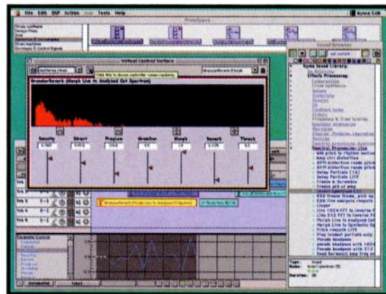
FIG. 7: Symbolic Sound's Kyma System is one of the most powerful sound-design workstations around. It's especially easy to load a "default" source sound into the system and try dozens of different manipulations.
