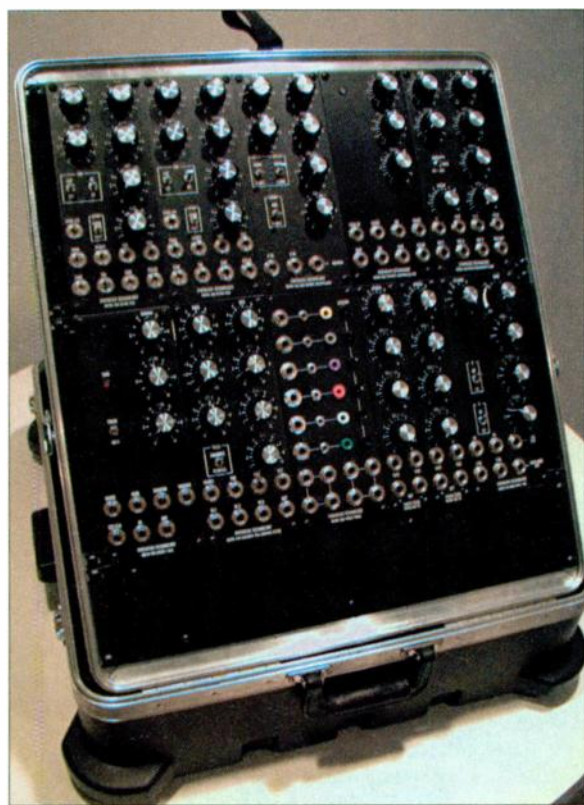
Synthesis Technology's MOTM modules are designed to fit standard 19-inch racks, so you can mount five double-wide modules side by side. The system in this photo includes a row of 6 modules, for a total of 11 modules in a portable SKB case.
