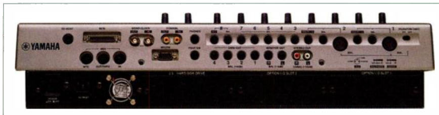
FIG. 2: The AW4416 offers a pretty good package of inputs and outputs, including full-featured mic inputs with phantom power and inserts and six TRS mic/line inputs. Channel 8 has an additional high-impedance input. Any combination of inputs and outputs may be routed to the S/PDIF digital I/O.
