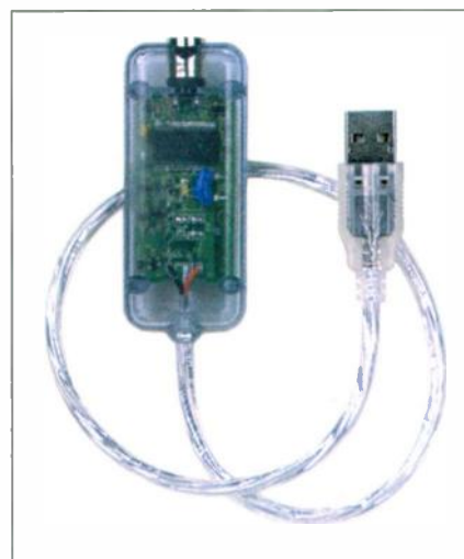
FIG. 3: The Griffin iMate USB-to-ADB adapter lets you use some old ADB dongles with the newer Macs.
