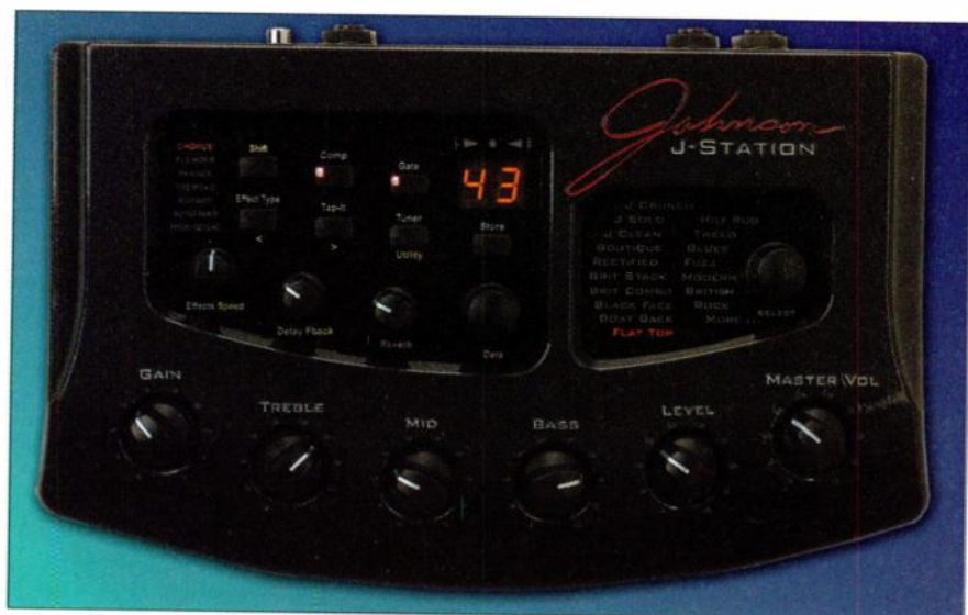
The Johnson Amplification J-Station provides models of 12 different guitar amps (and a slot for extra software-updatable models developed by Johnson), 3 bass guitar amps, and 2 acoustic guitars. Its versatile effects section can be edited at the Top Level and Deep Level.
