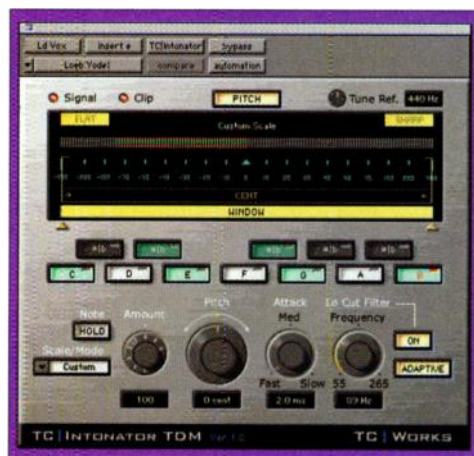
FIG. 3: TC Intonator's guitar tuner-style bar meter shows how sharp or flat the input signal is compared with a desired note in red and the amount of applied pitch correction in green. In this example, a flat note is perfectly "corrected" to B.
