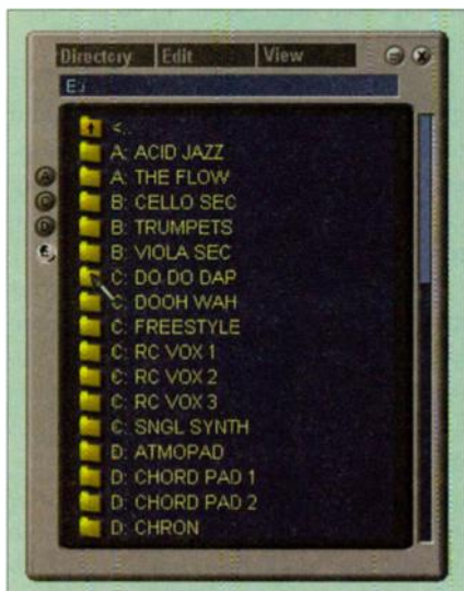
FIG. 3: The file browser shows all the available samples and programs on your system. It can also display partitions on Akai-format disks.
