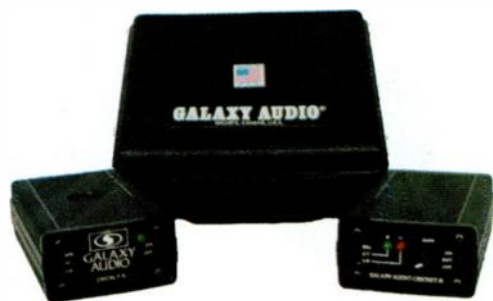
FIG. 4: The Galaxy Cricket tests speaker polarity. It includes a clicker and a listener.
