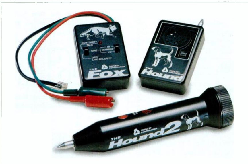
FIG. 5: The Triplet fox and hound helps trace cables in a bundle. The fox injects a signal, which is picked up by the hound.
