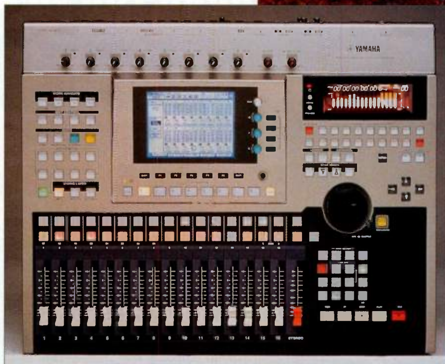
FIG. 1: The AW4416's buttons and switches are grouped according to use, with utility and mixer functions on the left and recording functions on the right. Eight sample pads are directly below the central display. A second display for metering and counter functions appears in the upper right corner.
