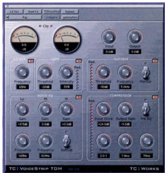
FIG. 1: TC VoiceStrip has a vintage-style interface and provides five individual effects modules, including a low-frequency cut, gate, de-esser, EQ with soft saturation, and compressor.
