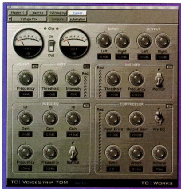
FIG. 2: When you bypass TC VoiceStrip , the entire control panel turns gray, which lets you know that the processor is disengaged.
