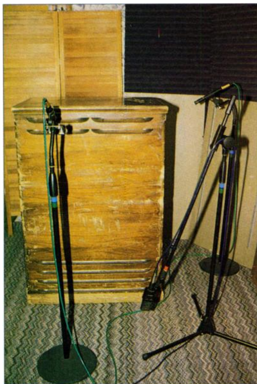
Two AKG C 460 microphones capture a stereo image of Eisenberg's Leslie model 122 while an AKG C 414 B/USL brings in the lows.
