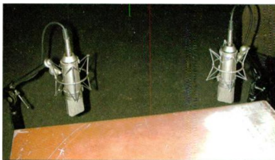
FIG. 3: When using the stereo-miking setup illustrated in Fig. 2c, angle the mics as shown so the live horn will be on axis with each mic during its rotation. Note, too, how the mics are positioned to accommodate the off-center mounting of the treble-horn assembly inside the cabinet.
