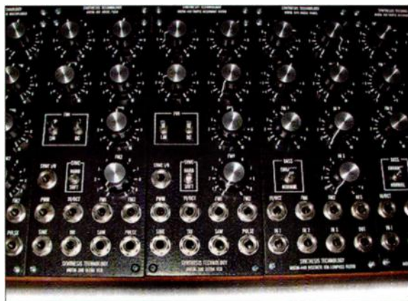
FIG. 3: Looking closer at the MOTM-300 front panel, you can see the 1/4-inch jacks conveniently placed at the bottom.
