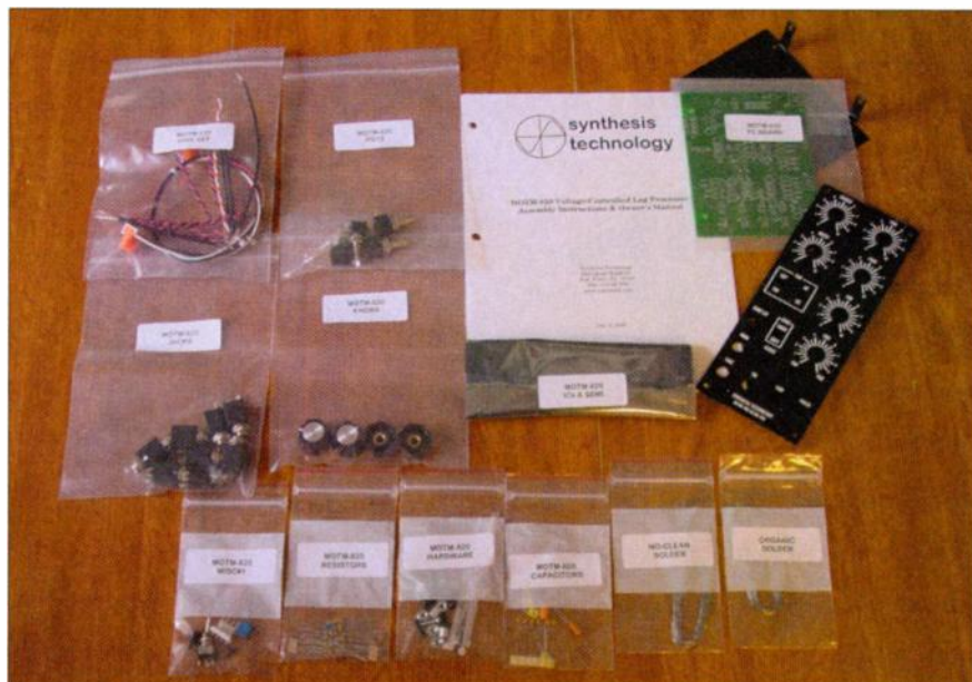
FIG. 14: This kit from Synthesis Technology contains all the parts needed to build your own MOTM module.
