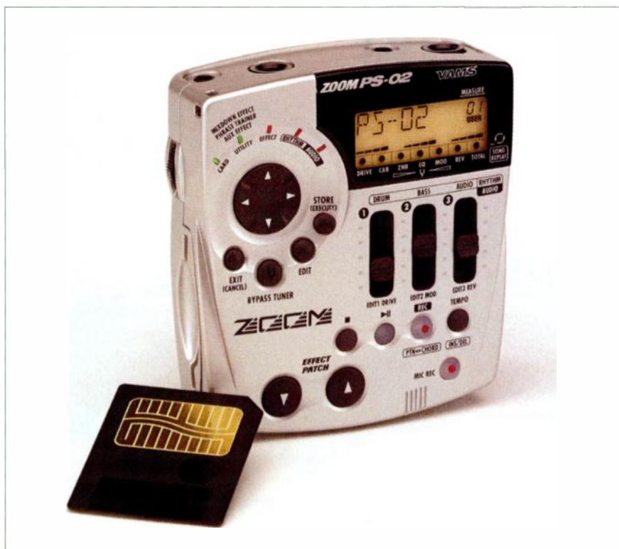
The Zoom PS-02 Palmtop Studio is a 3-track audio recorder (with 30 virtual tracks), a bass and drum machine, and a standalone effects processor that almost fits in your shirt pocket. Maximum recording time is determined by its SmartMedia card's capacity.
