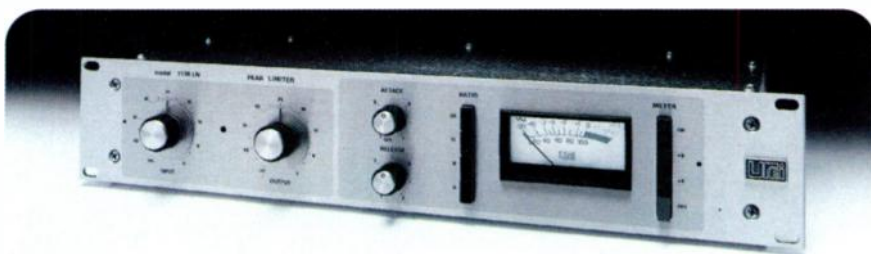
FIG. 2: The UREI 1176 limiting amplifier came in three styles: the original had a black face, the first revision a silver face with a blue stripe, and the second revision (shown here) a silver face. All remain favorites of many pro mixers for processing vocals, bass, and other instruments.
