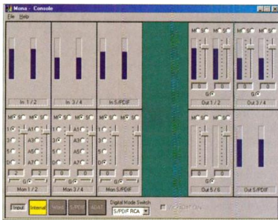
FIG. 3: Echo Console offers onscreen control of Mona's input monitoring and output levels and several other parameters.
