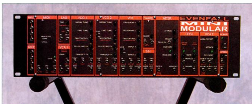
FIG. 8: The Evenfall Mini Modular is a full-featured, semi-modular synthesizer. It includes a built-in MIDI-to-CV converter, sample and hold, and a waveshaper.
