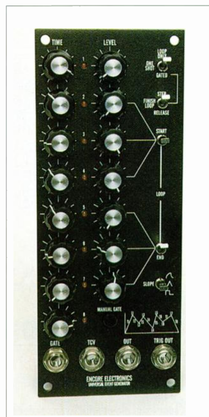
FIG. 7: The Universal Event Generator is a microprocessor controlled module that can be used as an 8-stage envelope generator, sequencer, or LFO.
