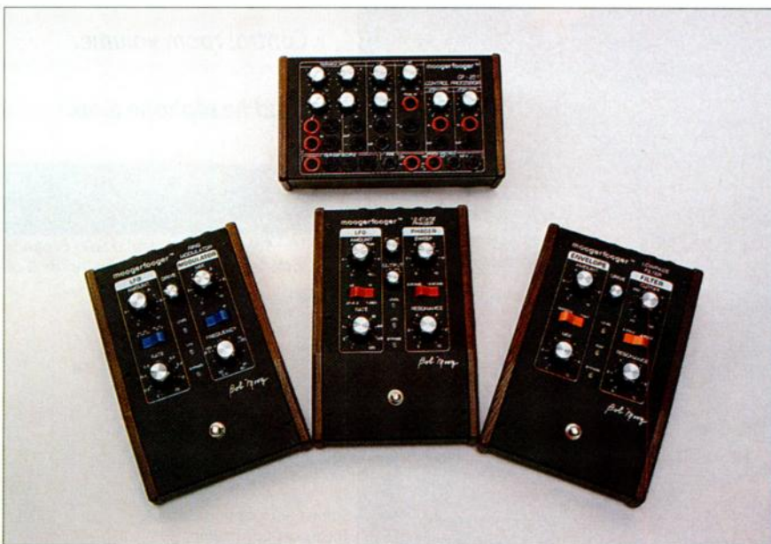
FIG. 3: With the addition of the CP-251, the Moogerfooger line of effects from Big Briar can be combined to form a simple but effective synthesizer.
