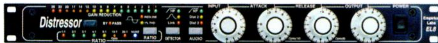
FIG. 3: The Empirical Labs Distressor is one of the more popular modern compressors among pro mixers, due both to its great sound and extreme versatility. Note the "Nuke" ratio setting.
