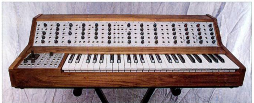
FIG. 2: The Analogue Systems Sorcerer combines two rack spaces of modules with a 4-octave keyboard, MIDI I/O, and a joystick controller.
