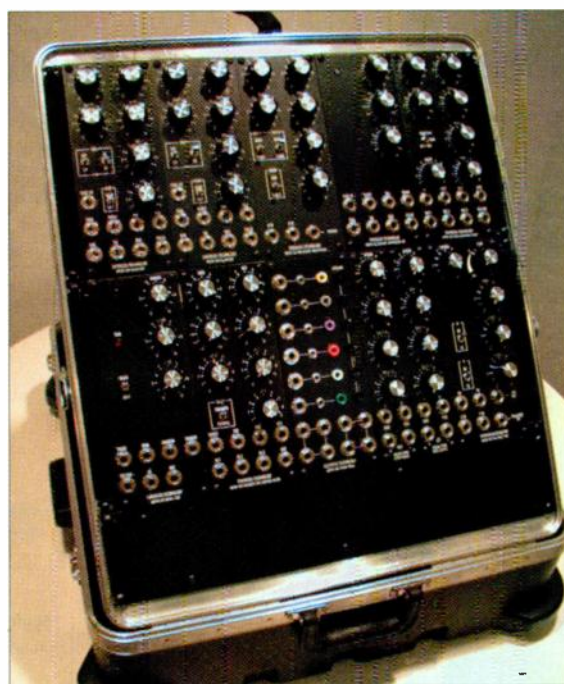
FIG. 13: The MOTM modules from Synthesis Technology are designed to fit into an SKB road case.
