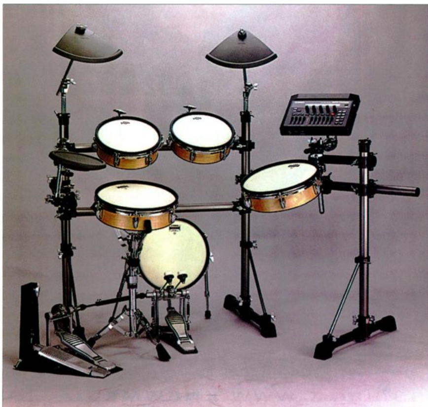
FIG. 21: Yamaha's DTXtreme electronic drum-set system combines a GM-compatible multitimbral drum module with a selection of Real Head Pads.
