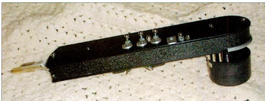
FIG. 15: Nyle Steiner makes the MIDI EVI to order. Like the Akai EWI, the EVI uses touch-sensitive buttons, but it is fingered like a trumpet rather than like a sax.
