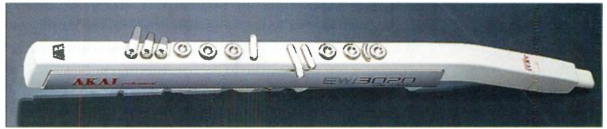
FIG. 12: The EWI3020, Akai's third-generation MWC, uses touch-sensitive buttons rather than moving keys.
