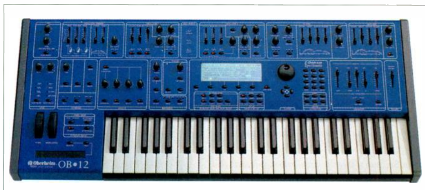
FIG. 1: Dozens of knobs, sliders, and buttons are arranged in functional blocks on the OB-12's front panel and provide plenty of hands-on access to real-time control.
