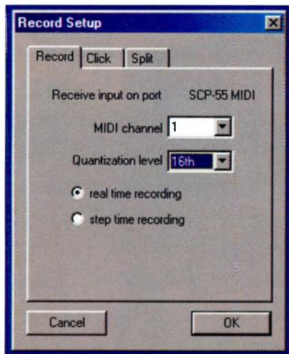
FIG. 3: The Record Setup window allows you to set the quantization level for real-time MIDI input or to specify step-recording instead.
