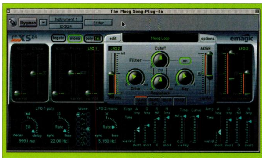
FIG. 1: EXS24's main Editor control panel has an intuitive user interface that includes an excellent lowpass filter, two LFOs, and two ADSR envelope generators. Many of the sliders in the window's upper portion are split, letting you set a modulation range.
