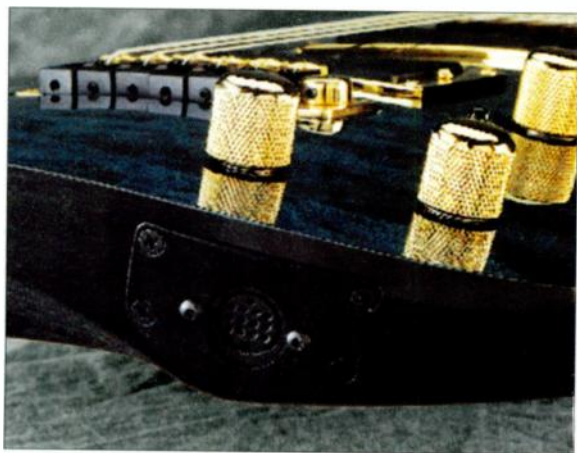
FIG. 1: The 13-pin jack has become the standard conduit for the divided string pickups to the converter unit, where the analog signal is converted to MIDI data.
