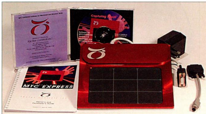
FIG. 1: The Tactex MTC Express comes with a cross-platform application program interface for creating instruments and controllers.
