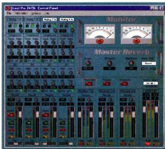
FIG. 3: The Direct Pro's Control Panel window emulates a 10x2 hardware mixer, which lets you control the four physical inputs, the system's onboard effects, and six playback channels from a multitrack audio application.
