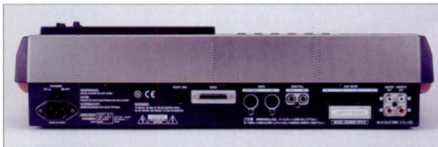
FIG. 2: The DPS16's uncluttered back panel provides stereo main outputs, stereo monitor outputs, four aux sends, S/PDIF I/O, two MIDI ports, and a SCSI connector.
