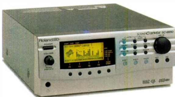
The SC-8850 Sound Canvas from Roland ED provides the user with high-quality GM1, GM2, and GS sound sets in a tabletop unit with a USB connection.
