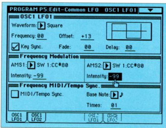
FIG. 1: For an excruciatingly slow LFO, assign a modulator such as SW1 to both of the LFO's Frequency Modulation inputs.
