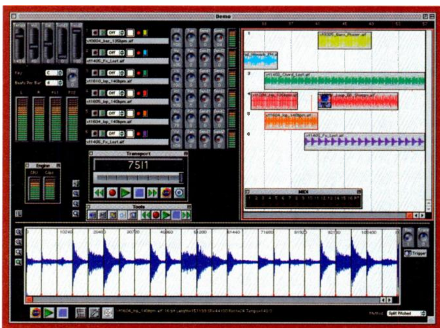
FIG. 1: Phrazer's track display appears to the right of its customizable set of controls; a movable divider lets you reveal more of the display. The sample editor at the bottom of the window lets you edit loops and adjust split points.
