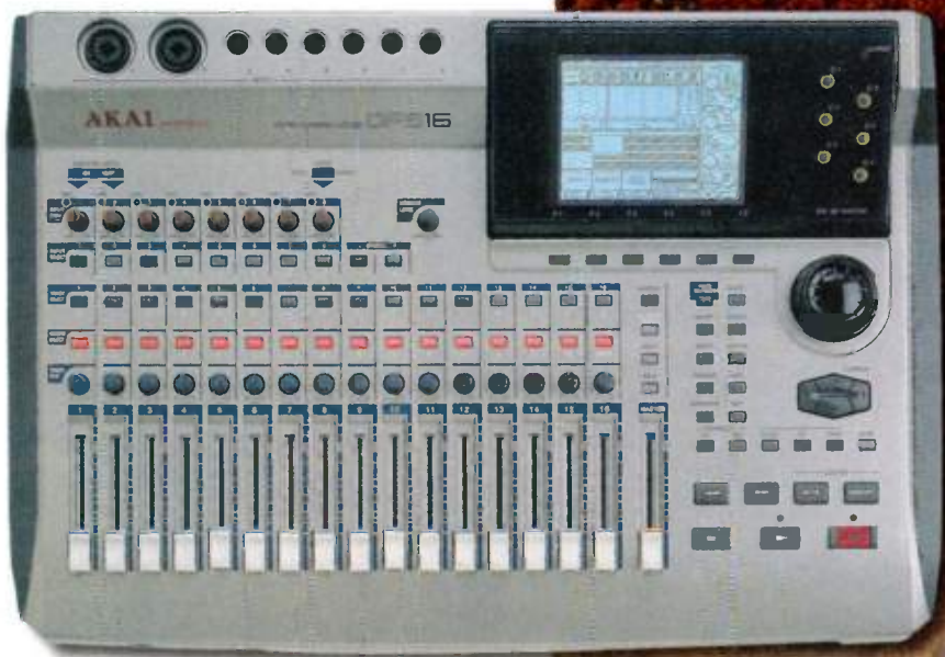
FIG. 1: The DPS16 has 16 nonmotorized channel faders and one main fader. Dedicated buttons and knobs are supplemented by soft controls whose functions appear in the tilt-up display. Two of the eight analog inputs accept XLR or 1/4-inch plugs and offer switchable phantom power.
