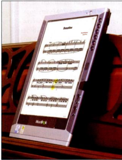
FIG. 2: AMuseTec's MuseBook Score relies on MusicXML for its combination of music-performance recognition and its automatic page-turning capability.
