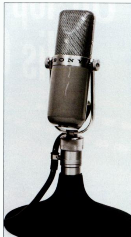
FIG. 2: One of the mics that Chiccarelli likes to use for various instrument applications is the Sony C37A, an out-of-production tube mic.
