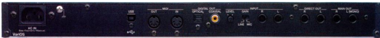
FIG. 2: The VariOS's rear panel provides ports for analog and digital audio and MIDI, as well as a USB port for connecting to your computer.
