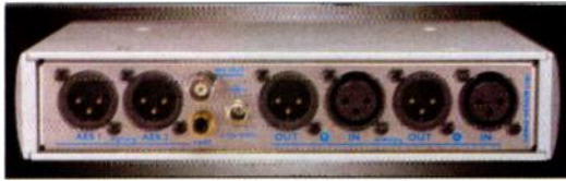
FIG. 2: The V3 has dual AES/EBU digital outputs, a S/PDIF output, a BNC word-clock out, and balanced XLR analog I/O.
