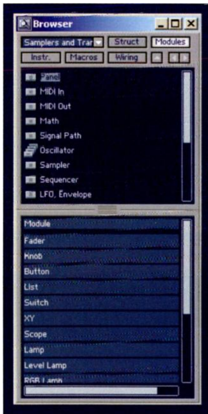
FIG. 2: Reaktor 4's new Browser window toggles between several views. The Modules shown here can be dragged directly into the Structure window for inclusion in an Instrument.
