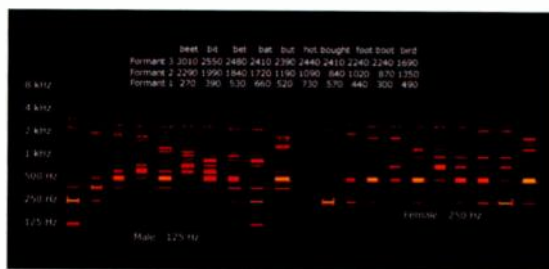
FIG. 4: This spectrogram shows an analysis of synthesized vowel sounds using a subtractive synth and three formants. The ten vowels on the left use a 125 Hz source (male), whereas those on the right use a 250 Hz source (female). The formants and vowels are shown in the inset at the top.
