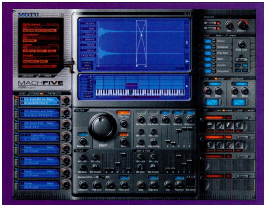
FIG. 1: MOTU's MachFive 1.07 uses a single control panel with eight functional areas. The File Browser and Part sections (left) manage presets on disk and in memory. The Display Area and Keygroup parameters (center) handle multisample management. The Master section, Part parameters, LFO section, and FX section (right) control output parameters, LFO selection and routing, and effects.
