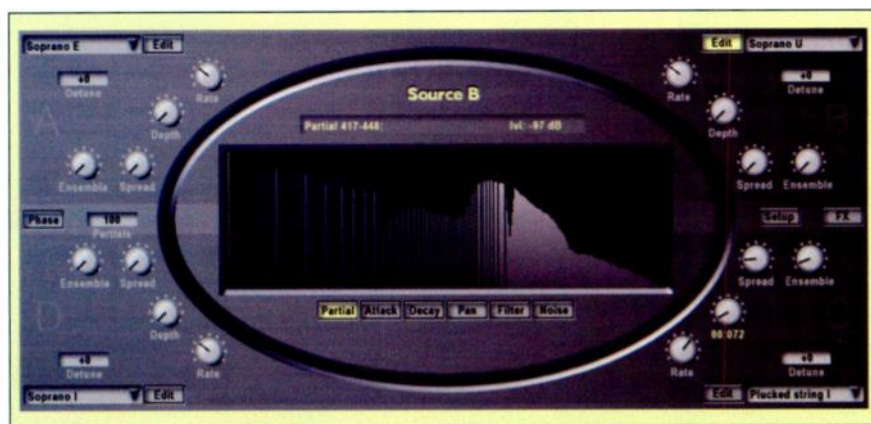
FIG. 2: Cube allows you to control the amplitudes of as many as 512 partials. Each of its four Sound Sources has its own parameters for the partials and for the major sound-processing functions.
