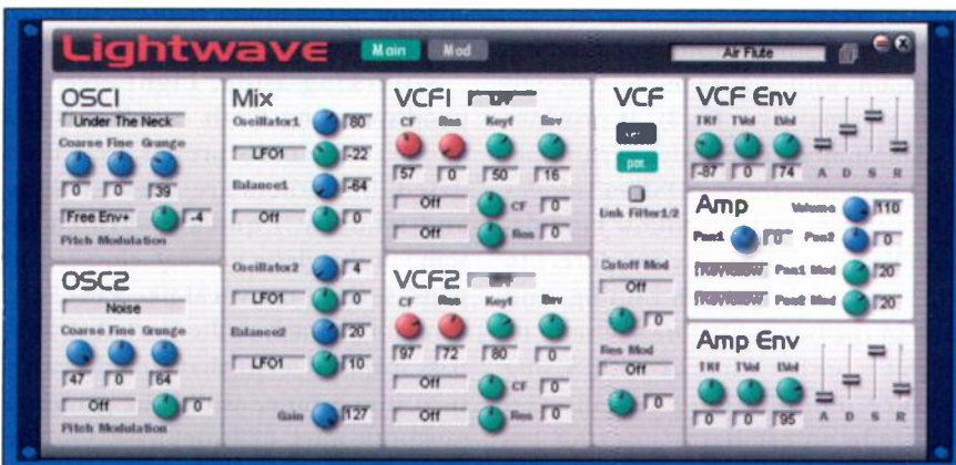
FIG. 3: Noah's Lightwave synth is a two-oscillator design with dual multimode filters and two LFOs (not shown on this panel).
