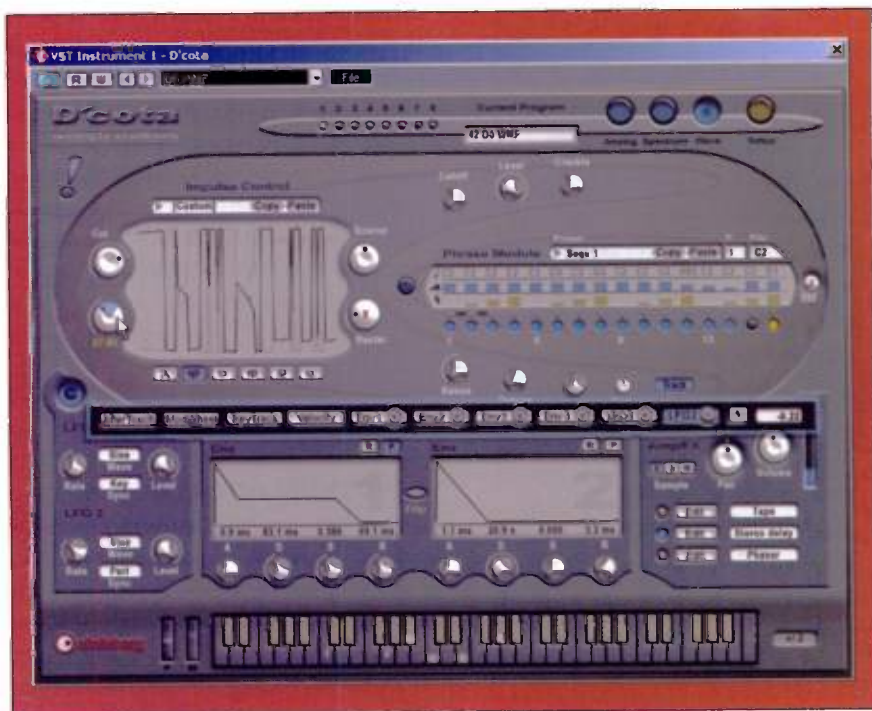
FIG. 2: D'cota's Wave panel includes a simplified Spectrum tone generator (left) and a step sequencer (right). The horizontal bar above the envelopes is for editing modulation routings.
