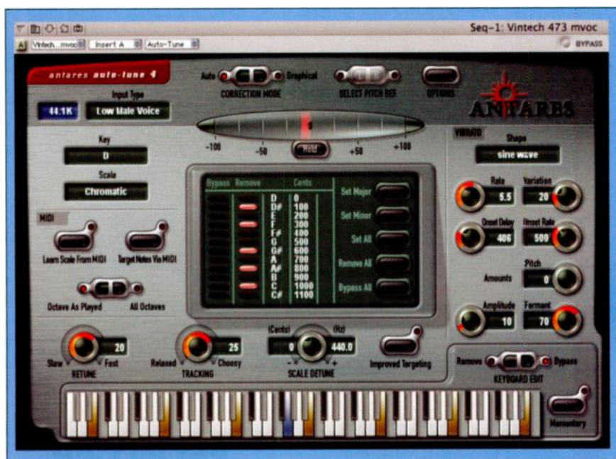
FIG. 1: One of the improvements in Auto-Tune 4 is the Virtual Keyboard, which shows the currently detected pitch (blue key), scale notes (white and black keys), bypassed notes (brown keys), and removed notes (gray keys). Scale notes can also be input from the keyboard.
