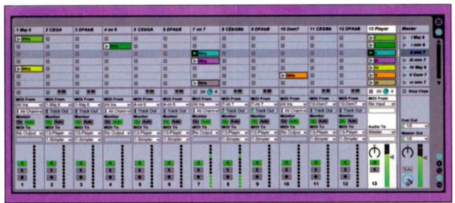
FIG. 3: Live's robust signal-routing scheme allows MIDI tracks to take their input from and send their outputs to any other track as well as any hardware or ReWire MIDI device.
