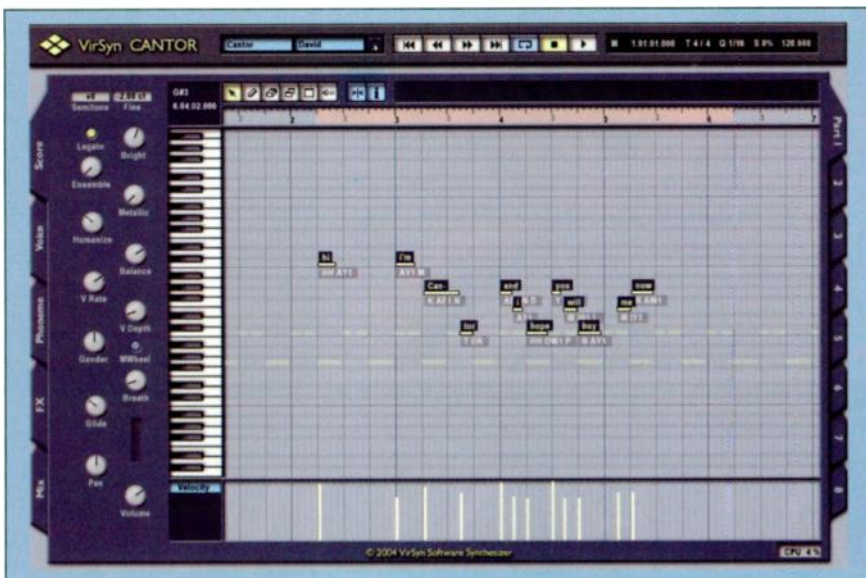
FIG. 1: VirSyn Cantor's Score editor is used for entering and editing notes and lyrics.
