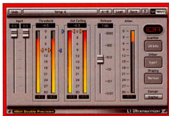
FIG. 2: The L1 Maximizer plug-in from Waves is highly regarded for its ability to tame peaks transparently, allowing the overall gain of a track to be increased without affecting its perceived dynamic range.
