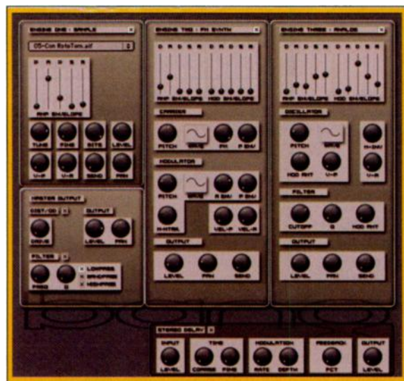
FIG. 1: Cycling '74 Mode's Bang drum synth has three sound engines: a one-shot sample player (left), an FM synth (center), and a classic analog synth (right). Distortion, filter and delay effects round out the module.
