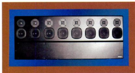
FIG. 1: Each IOSONO panel has 8 tweeters, 8 midrange drivers, and 16 power amps.
