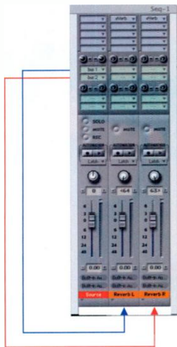
FIG. 1: Using two mono reverbs can be a good alternative to using a stereo reverb. In this example from Mark of the Unicorn's (MOTU's) Digital Performer 4.12, the source track is bused to two mono instances of MOTU's eVerb plug-in, which are panned left and right.
