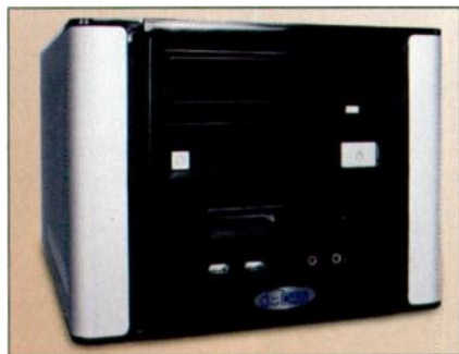
FIG. 1: The compact, lunchbox-style DAWin QB-4 Mini PC DAW (pictured above) from Digital Audio Wave requires a specially shaped motherboard but still fits full-size PCI cards.
