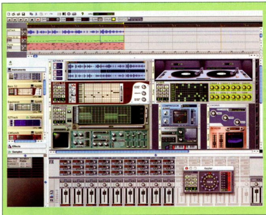
FIG. 1: Arturia Storm's studio is centered on a rack full of virtual gear. The rack includes the sequencer (top), mixer (bottom), and browser (left).
