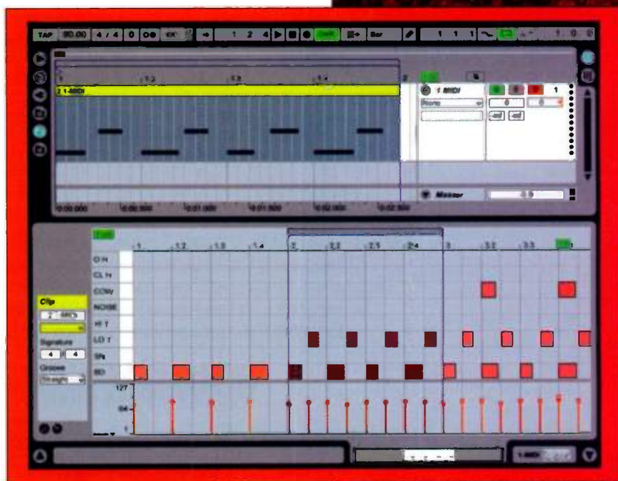
FIG. 1: In Ableton's Live 4.0, all three overdub passes of a one-bar recording are kept in the same MIDI clip, allowing previous takes to be selected using the loop markers.
