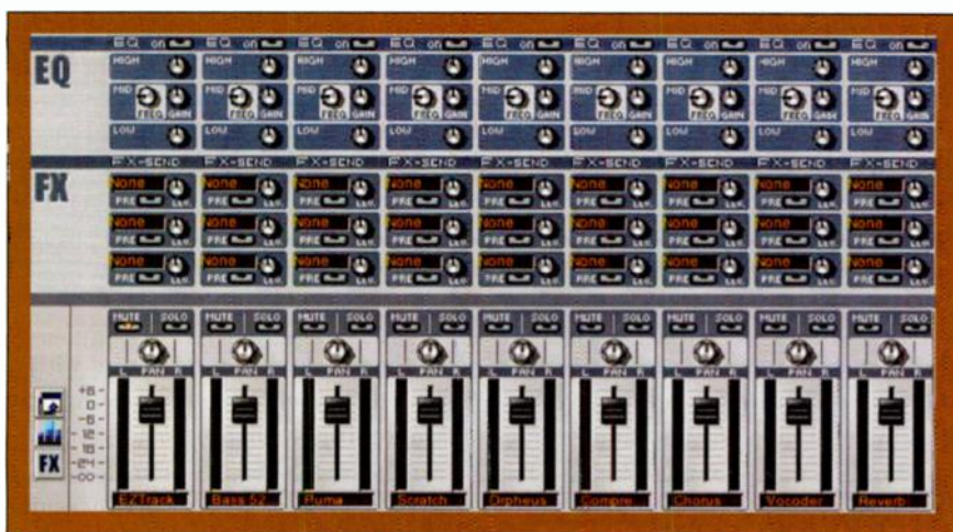
FIG. 3: Storm's mixer has channels for each instrument and effect. Three-band EQ and effects-send displays are optional.
