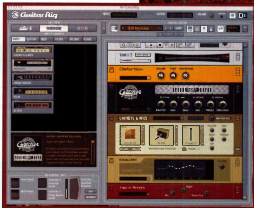
FIG. 1: You add components to your rig by double-clicking their icons in the Left View or by dragging them into the right frame at any spot in the signal chain.
