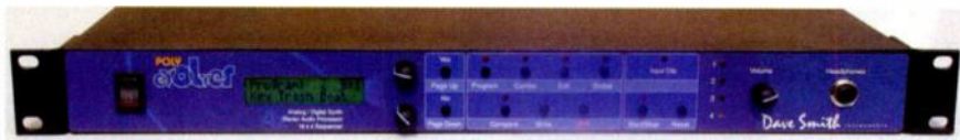
Dave Smith Instruments' Poly Evolver is a 4-voice rackmount version of the Evolver. Combining analog and digital sound engines, it offers four times the sound-generation and sound-manipulation capabilities of the original and adds various new features.
