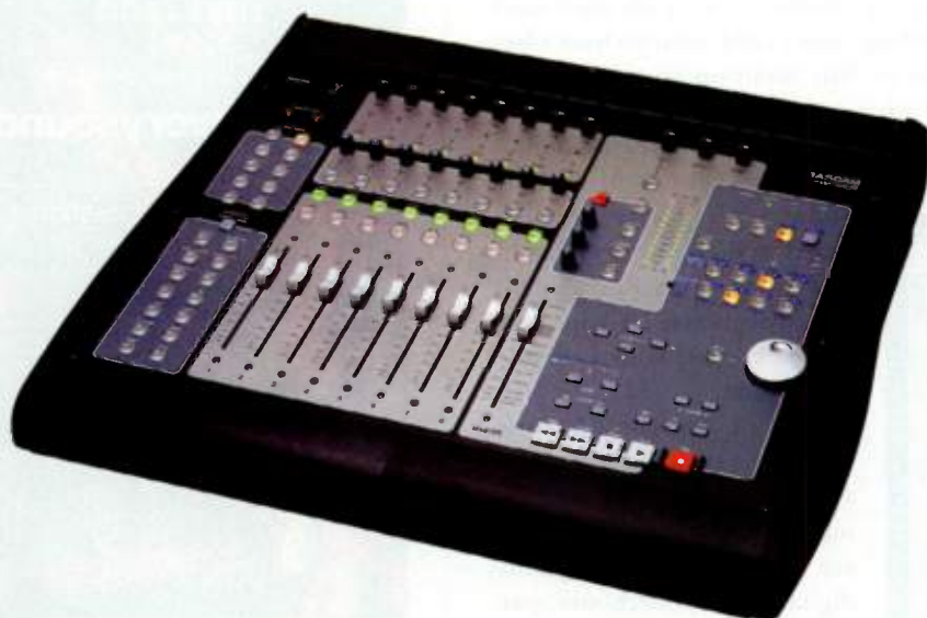
FIG. 1: FireWire connects the Tascam FW-1884 to a Mac or a PC, giving DAW users an 18-channel audio interface, a multipoint MIDI interface, and a control surface with motorized faders. The top panel organizes controls in functional groups, with channel strips in the middle and transport controls on the lower-right side.
