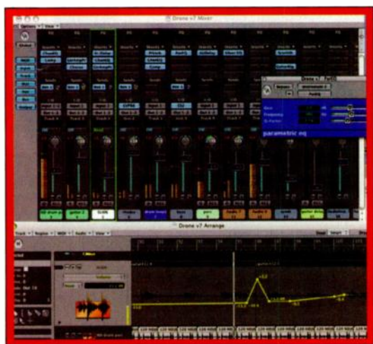
FIG. 1: A digital audio sequencer's mixer, such this one from Apple's Pro Logic 7, offers you powerful features including automation of volume, pan, mutes and effects parameters; recall; and the flexibility of plug-in effects processing.
