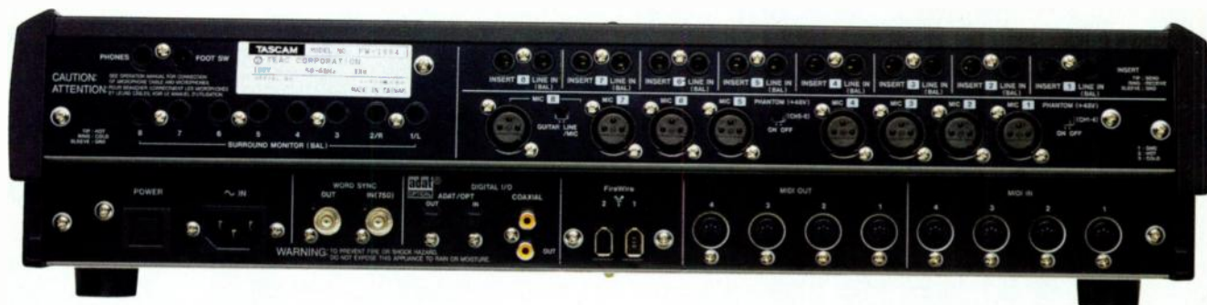
FIG. 2: All of the FW-1884's I/O connections are on the rear panel. Each channel has balanced 1/4-inch and XLR jacks that you can use simultaneously. Four sets of MIDI In and Out ports accommodate 64 MIDI channels.
