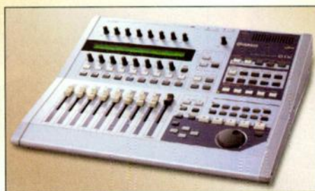
FIG. A: The Yamaha 01X gives you the automation and recall of a sequencer's mixer, with the physical control of a hardware console.
