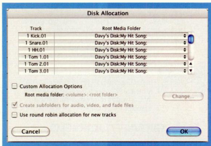
FIG. 2: Pro Tools' Disk Allocation window clearly shows where the audio for each track is being stored and allows you to reassign the files to a different folder.
