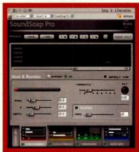
FIG. 2: The Hum & Rumble tab allows for control over low-frequency noise in a range from 20 Hz to 500 Hz.
