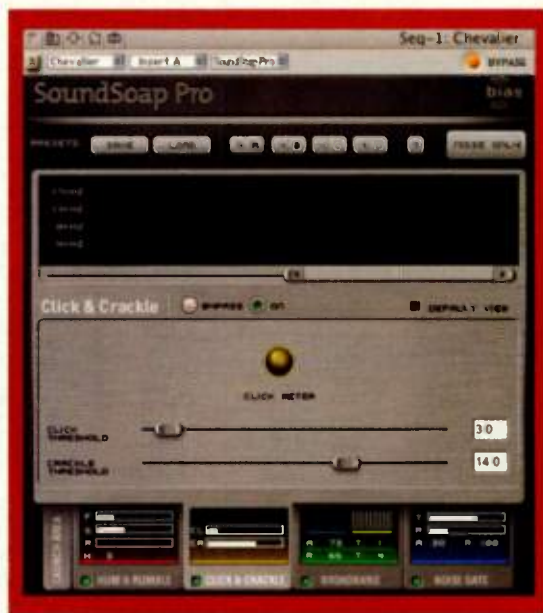
FIG. 3: The Click & Crackle tab has settings designed to eliminate transients (such as those found on vinyl records) and other sources of pops and static sounds.
