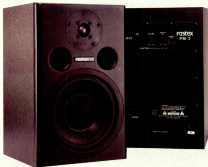
FIG. 3: The Fostex PM-2's amps provide 120W RMS each to the woofer and tweeter, and its rear panel features a variable Tweeter Gain pot and a three-position Woofer Gain switch.
