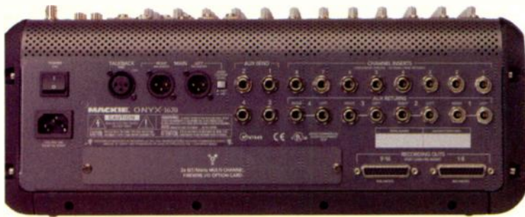
FIG. 2: The 1620's rear panel houses twin DB-25 connectors for direct-out analog recording and a slot for the optional FireWire card.
