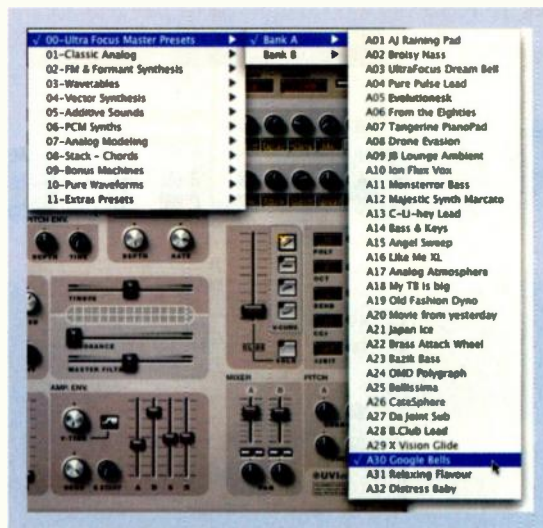
FIG. 2: Presets are arranged in folders and accessed using a hierarchical pop-up menu. Master Presets are organized into two banks, each with 32 dual-layer selections.
