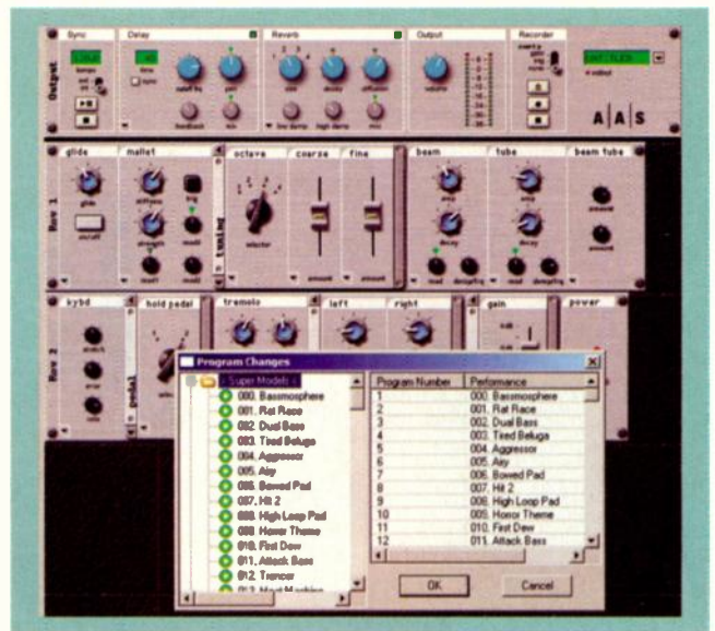
FIG. 2: Tassman 4 now offers a map to associate any preset with a Program Change message.
