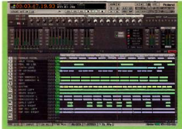
FIG. 4 With the VS20-VGA option installed, the Home screen on an external display reveals pull-down menus, transport controls, and other details you won't see on the LCD.
