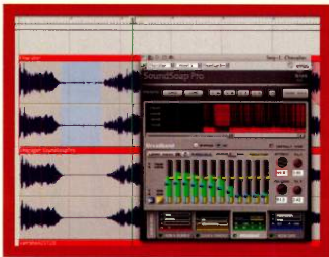
FIG. 4: The Broadband tab contains the Learn button, which takes an instant or user-defined measurement of designated consistent noise such as tape hiss. Visible under the plug-in are the original test track that was imported from DVD and the same track after processing by the Noise Gate module.
