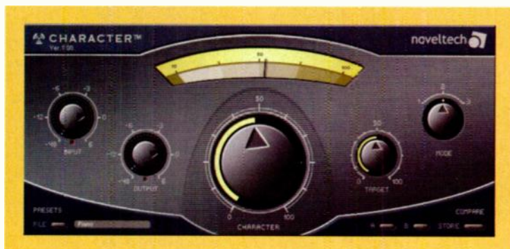
FIG. 2: Character is a simple but powerful spectral enhancer that analyzes incoming audio for frequency and dynamics and adapts its processing accordingly.
