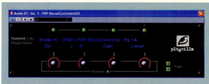
FIG. 2: The PSP Audioware ProZilla series of plug-ins allows you to use a VST host application to configure the plug-in before transferring the effect to the Manifold Labs Plugzilla.
