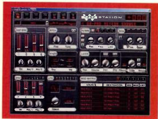
Wusikstation's single-window control panel contains layer selectors (top), a layer settings section (middle), and a modulator and modulation-routing section (bottom).
