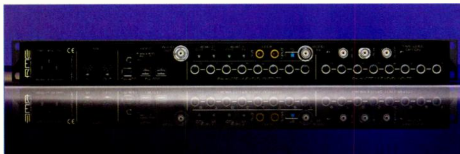
FIG. 2: The rear panel contains analog and digital I/O as well as MIDI and word-clock connections.
