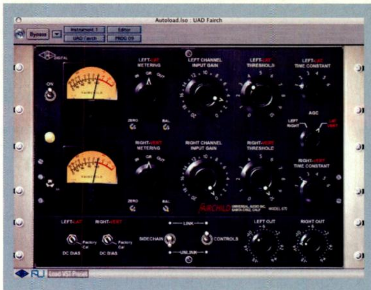
FIG. 1: Universal Audio's UAD-1 Powered Plug-in PCI card runs software models of classic analog hardware compressors and EQs, such as this emulation of the Fairchild 670.
