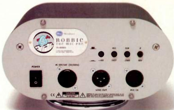
FIG. 2: Robbie's rear panel houses a power switch and buttons for selecting mic or DI mode, phase reverse, -20 dB pad, and 48V phantom power.
