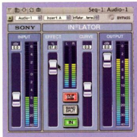
FIG. 3: The Sony InFLATOR plug-in runs on the TC Electronic PowerCore series of DSP accelerators and can be accessed in any VST- or AU-compatible native audio software.
