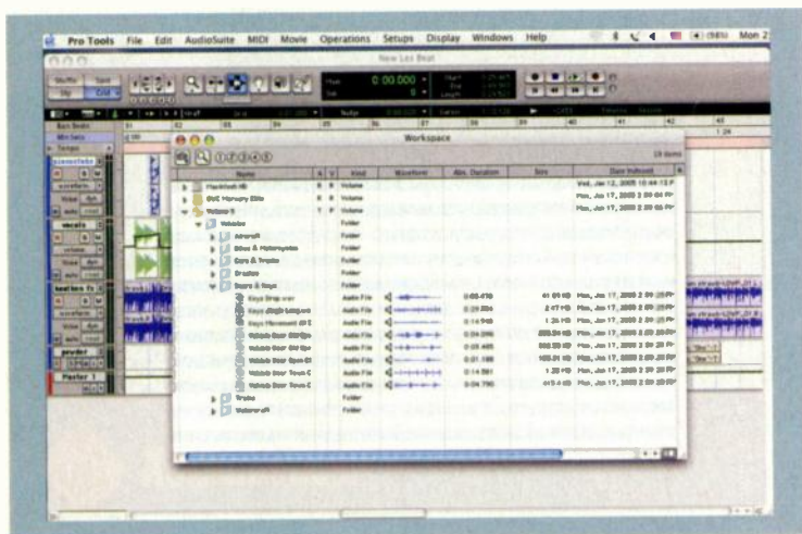
FIG. 2: From the Workspace window, you can see which drives and CDs are mounted and their content. Here, you can see the waveforms for the audio files, read the duration of each, and preview a file by clicking on its icon or waveform.
