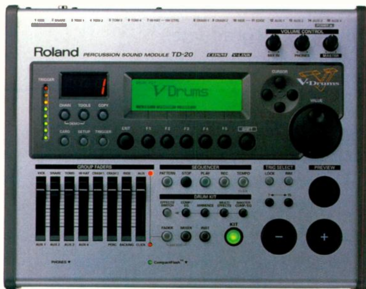
FIG. 2: Whether you're getting the right mix, editing a sound, or recording a sequence, the TD-20 is easy to use: a button is dedicated to nearly every important feature.
