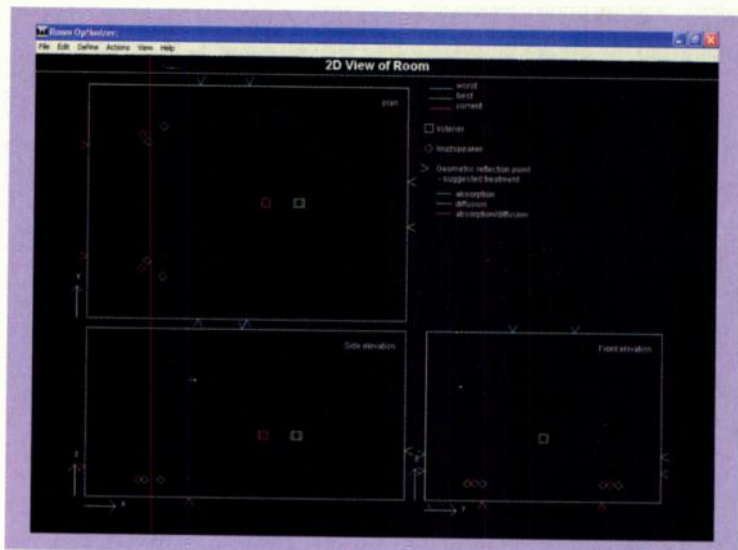
FIG. 4: RPG Diffusor's Room Optimizer software (Win) can calculate the optimal listener and speaker placement based on your room dimensions, speaker type, and other variables.
