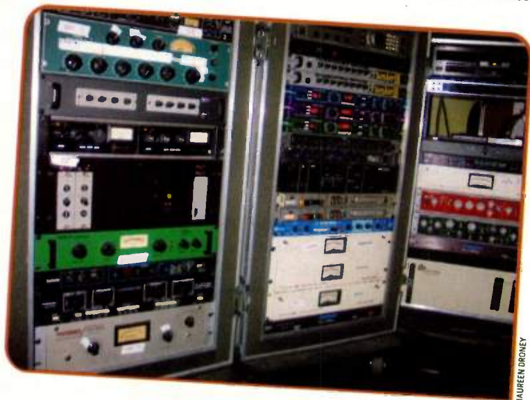
FIG. 1: Among the outboard gear in Wallace's racks is a Teletronix LA-2A (left rack, bottom), a CBS Laboratories FM Volumax compressor (middle rack bottom), and an Altec 1567A tube mixer-amplifier (left rack, second from top).
