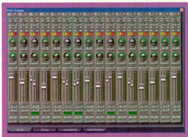
FIG. 3: GS3's revamped DSP Station functions like a mixing board with mute and solo buttons, faders, inserts, and level meters.
