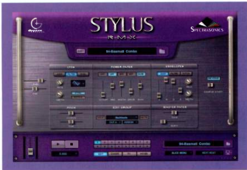
FIG. 1: A variety of options appear on the Edit page of Spectrasonics' Stylus RMX, one of which is its subtractive synthesis engine. Note the use of a synchronized triangle-wave LFO to modulate filter cutoff frequency on backbeats only, as shown in the Edit Group window.
