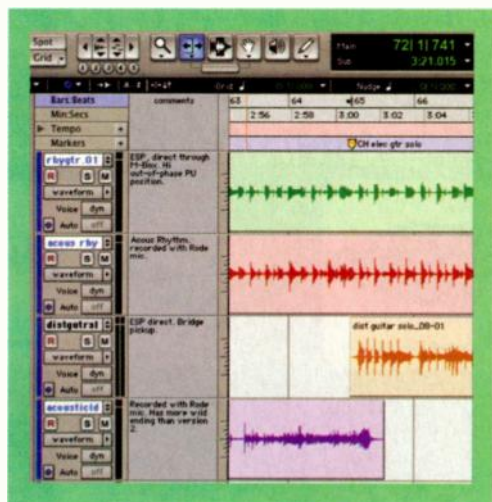
FIG. 3: In Pro Tools, as in many other sequencers, the track comments window lets you make notes about instruments and gear used as well as take status.
