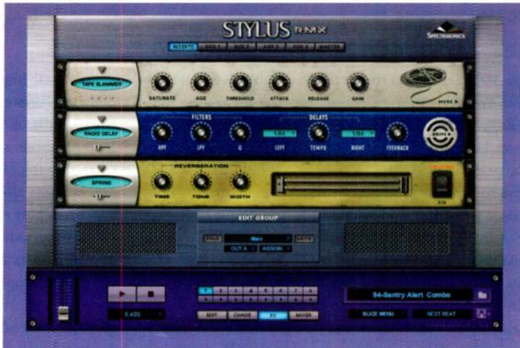
FIG. 4: The Insert rack is one of the many racks of effects in Stylus RMX. Four Aux racks and a Master rack each hold three effects. You can assign different effects for each Edit Group in the Insert effects and place effects in any order.
