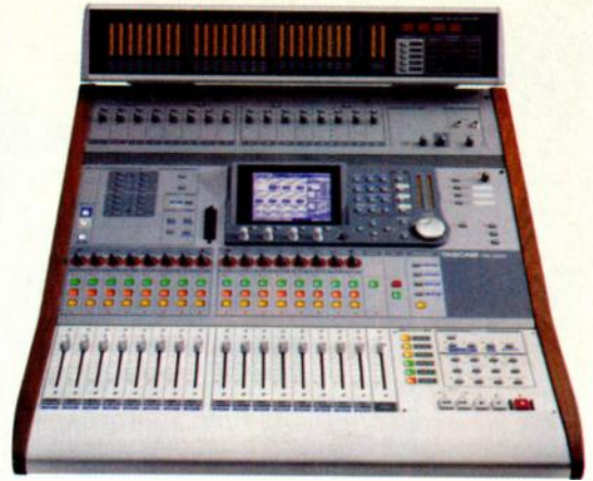
FIG. 15: The Tascam DM-3200 48-channel digital mixer has a wealth of inputs and outputs, motorized faders, plenty of signal processing, support for 6.1 surround mixing, and much more.
