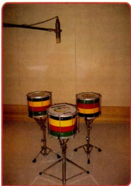
FIG. 3: Three repiques, miked with an AKG The Tube condenser mic.
