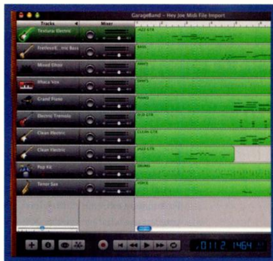
FIG. 3: Dropping a Standard MIDI File onto GarageBand's Timeline in the Tracks view creates a multitrack setup with an individual track for each channel of information.
