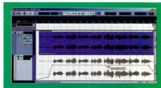
FIG. 3: In Cubase SX3, volume envelopes appear below the audio track that they control, in a separate display space that includes a gray version of the waveform. Note the text at the cursor, which shows the time and the level of an envelope point that has been clicked on.
