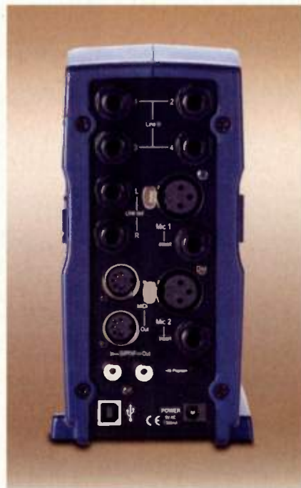
FIG. 2: The Omega's rear panel includes mic and line inputs and main outputs, and S/PDIF, MIDI, and USB ports.
