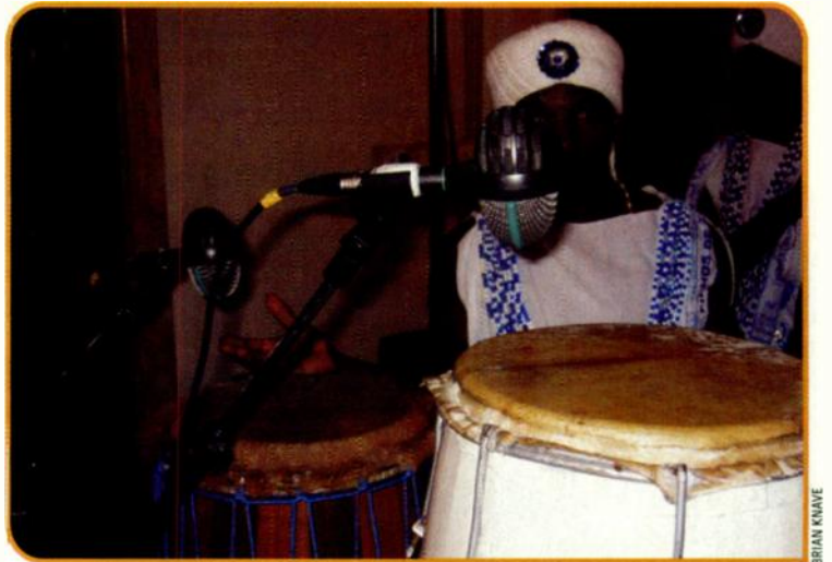
FIG. 4: Groove Studio's AKG D112s get lots of use on drum sessions. Here are two D112s positioned to capture the sound from the tops of the rums.
