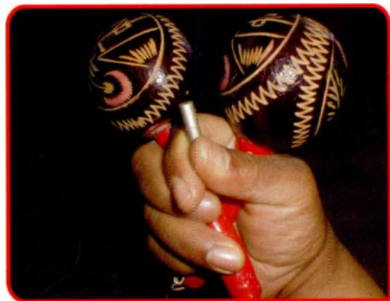
FIG. 4: This nonstandard miking method features a handheld lavalier mic used for capturing maraca sounds.
