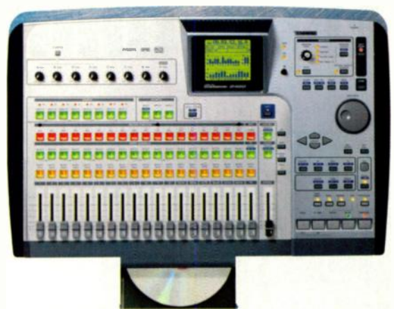
FIG. 11: The Tascam 2488 holds 24 tracks of audio and 8 tracks of simultaneous recording regardless of bit-depth settings. It also has a complete GM-compatible synth.
