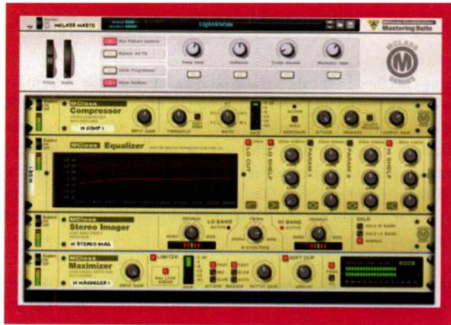
FIG. 3: The MClass mastering suite combines maximizer-style limiting for finalizing your mixes, parametric EQ, stereo enhancement, and a compressor.
