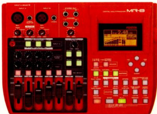
FIG. 3: The diminutive form factor of the Fostex MR-8, combined with a pair of XLR jacks, CompactFlash storage, and battery power make it a good choice for recording outdoors.
