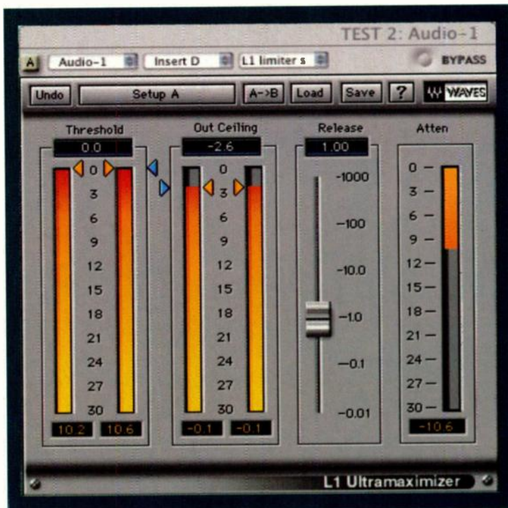
FIG. 1: If you experiment with overloading effects plug-ins, it's useful to put a limiter, such as the Waves L1, at the end of the chain.
