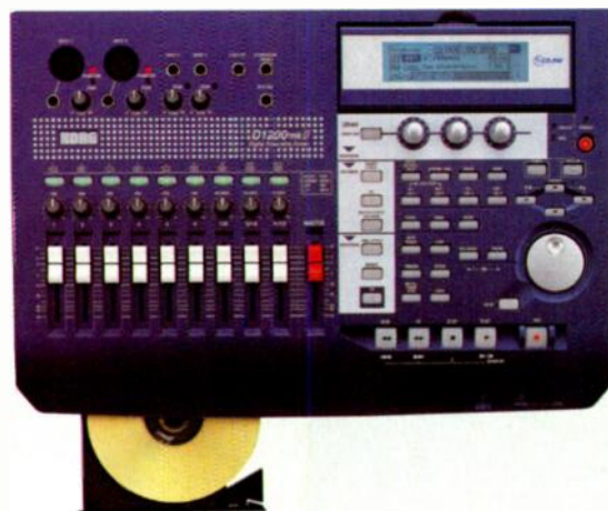
FIG. 9: The Korg D1200mkII lets you bounce all tracks down to overwrite a stereo pair of normal tracks, and includes the content of the target tracks. You can also bounce to virtual tracks.
