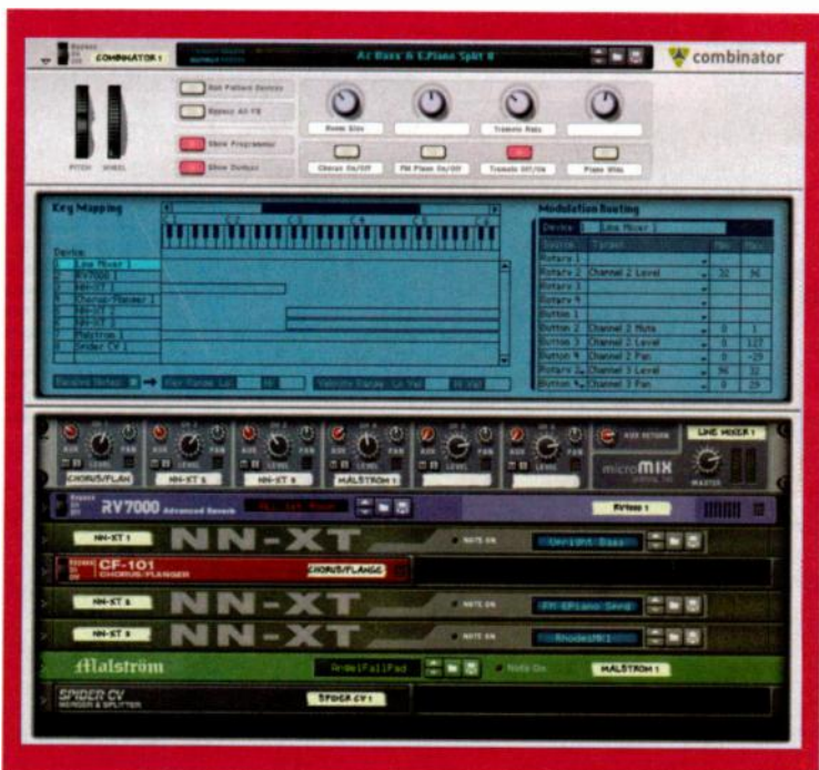
FIG. 2: The new Combinator is really a rack within the rack that allows you to combine several Reason devices into a single patch, called a Combi.
