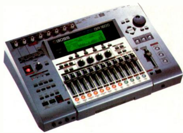
FIG. 7: Buttons on the Boss BR-1600CD give you direct access to application-specific DSP processes, such as the Vocal Tool Box.
