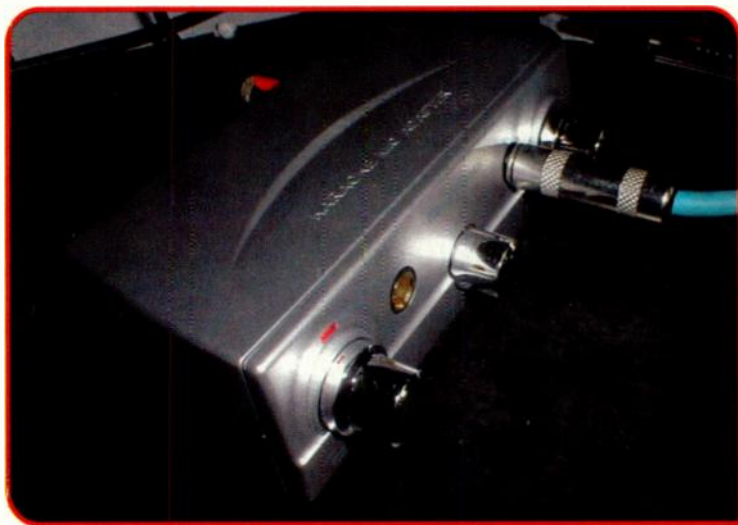
FIG. 3: Try using inexpensive consumer electronics, such as this Radio Shack Karaoke Mic Adapter (that features echo), as insert effects during mixdown.
