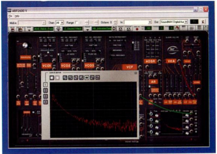
FIG. 3: The tracking generator lets you draw as many as four independent curves to use as modulation sources within 2600 V's architecture.
