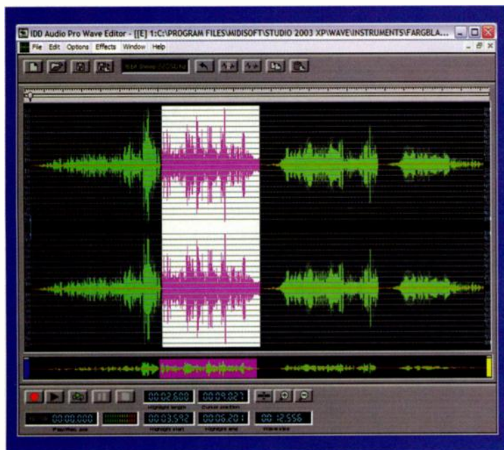
FIG. 13: AudioPro Wave Editor expands Studio Ensemble 2003's audio capabilities by adding waveform editing, normalization, simple noise reduction, and other DSP processes.
