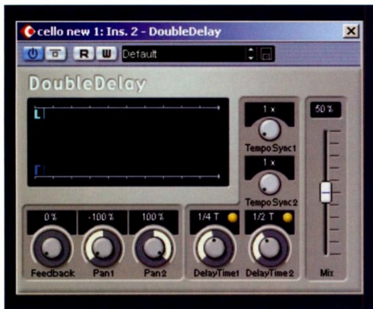
FIG. 1: The stereo delay in Cubase SX3 includes a separate delay time and output panning knobs for the two delay lines. The wet/dry mix slider is at the right side of the screen.
