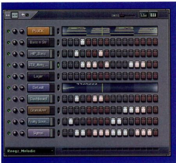
FIG. 1: FL Studio's Step Sequencer lets you program soft synths and samplers using familiar techniques that were originally developed in the '70s for programming drum machines.
