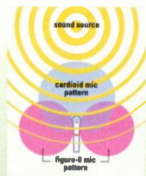
FIG. A: With M-S miking, a directional mic is used to pick up the middle of the stereo image, and a figure-8 mic is used for the sides.
