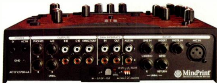
FIG. 2: The TRIO's rear panel has jacks for connecting two pairs of headphones, three pairs of speakers, a tape recorder, a computer audio interface, an outboard processor, a stereo keyboard, a guitar, and a microphone—all at the same time.
