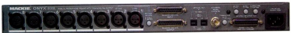
FIG. 2: The rear panel is where you find the XLR mic inputs, the analog line inputs and outputs (on DB25 connectors), and the various digital outputs.
