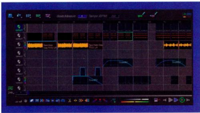
FIG. 5: The Montage Room is a 16-track audio sequencer for mixing files rendered in MetaSynth's other Rooms.
