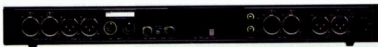
FIG. 2: The Rosetta 200's rear panel has two sets of XLR analog I/O, AES, S/PDIF, word clock, ADAT, and a pair of MIDI jacks for use with the company's FireWire extension card.
