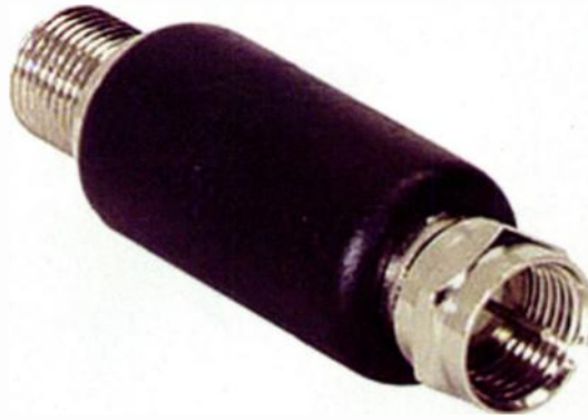
FIG. 10: Inserting an isolation transformer between the cable wire and your cable box or video recorder will alleviate hum that appears on video and computer monitors.
