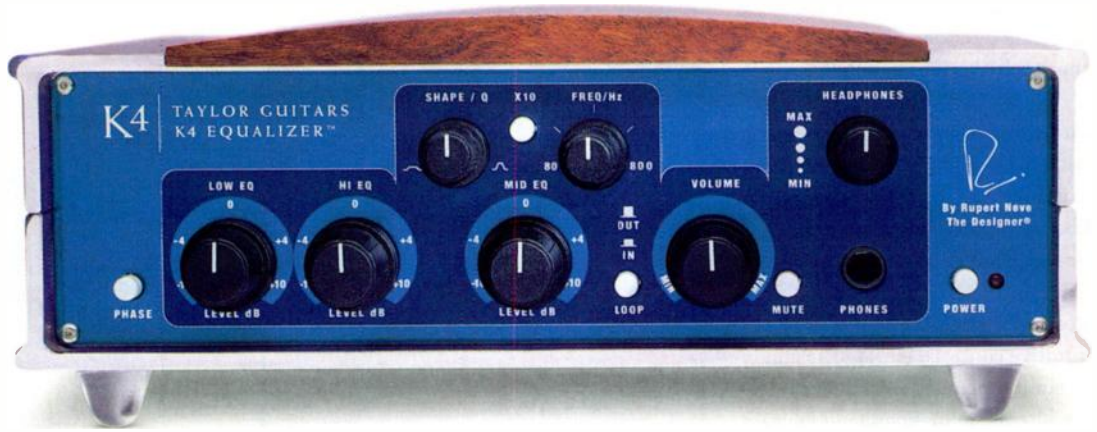
FIG. 1: Taylor's K4 Equalizer operates on either two C batteries or the included external power supply. A front-panel power LED changes from green to red when battery power is running low.
