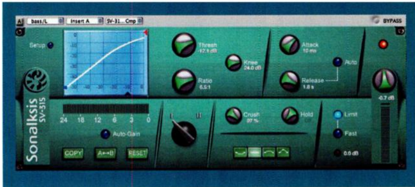
FIG. 1: SV-315 has two choices of compression curves (settings I and II). Crush and Hold knobs and a limiter section control the treatment of transients. Alternative sidechain-filter buttons are located below the Crush and Hold controls.
