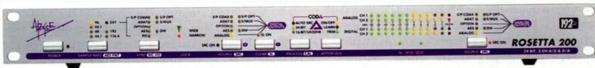
FIG. 1: The Apogee Rosetta 200 has two channels of high-grade A/D/A conversion and a multitude of routing options.
