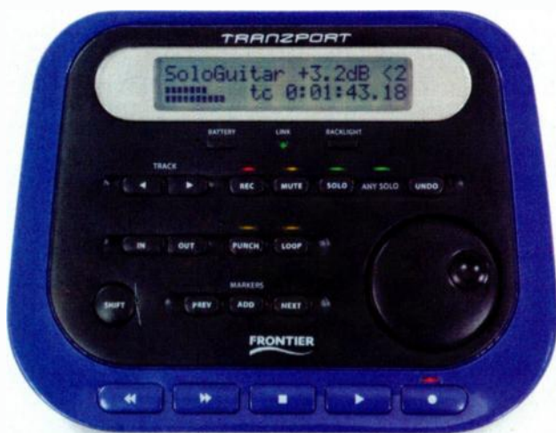
FIG. 1: Frontier Design Group's compact TranzPort wireless DAW controller is an excellent solution for controlling recording devices remotely. It is a flexible unit that would be suitable for many studios.
