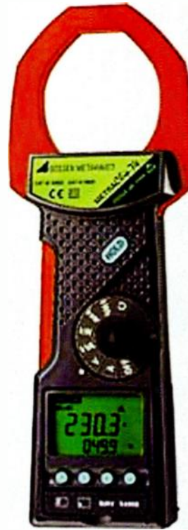
FIG. 4: A clip-on ammeter can be used to measure current consumption at the breaker box. The orange jaws open so that the power wire can be inserted.
