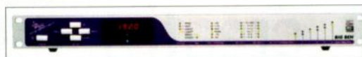
FIG. A: Apogee's Big Ben has a jitter-free clock source at sampling rates as high as 192 kHz for multidevice digital systems.
