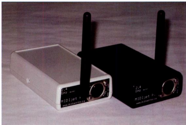
FIG. 2: The Classic MIDI Works MIDIjet Pro lets you set unique transmitter and receiver channels for as many as 31 separate wireless MIDI systems working in close proximity.
