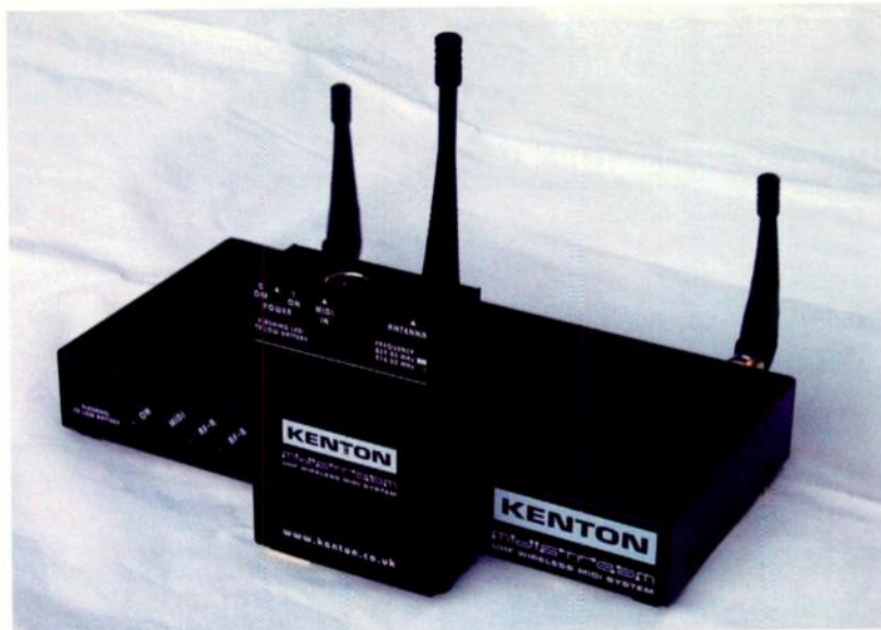
FIG. 1: The Kenton MidiStream wireless MIDI system sports a second antenna-and-receiver system. Should reception weaken over one antenna, the second can receive the signal.
