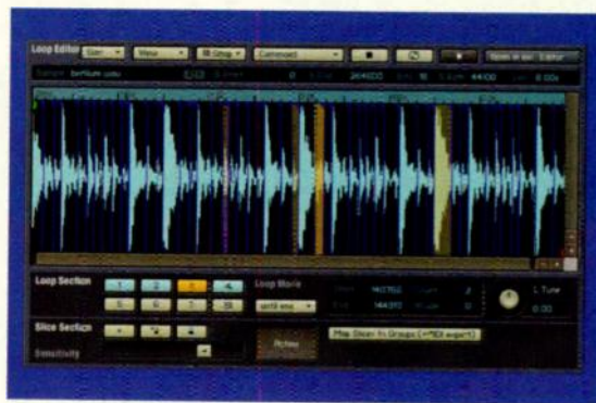
FIG. 3: The tear-off Loop editor serves two purposes: beat slicing and loop management. As many as eight loops can be defined simultaneously.
