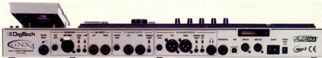
FIG. 2: The GNX4's rear panel is where connections are made for its various types of I/O, which include analog and digital audio, and MIDI.
