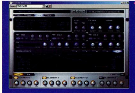
FIG. 3: The Dimension soft synth has four sample-playback oscillators and built-in effects. The unlabelled horizontal line at the lower right of the screen is used for keyboard scaling.
