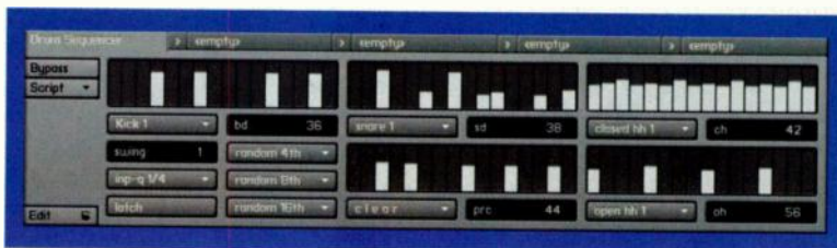
FIG. 5: The Script Processor allows as many as five scripts to be run in series. The factory drum-sequencer script is shown here.
