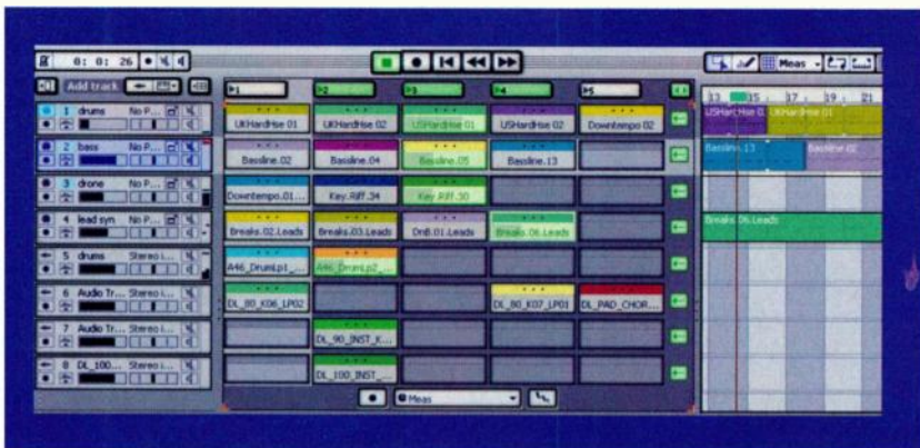
FIG. 2: MIDI and audio patterns loaded into the GrooveMatrix can be triggered interactively onstage. Patterns that are playing currently are light green and display progress bars.
