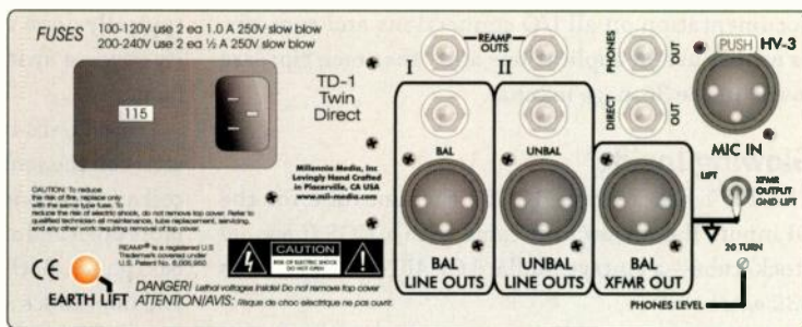
FIG. 2: The rear panel includes a range of outputs such as balanced and unbalanced ¼-inch and XLR jacks and a pair of ¼-inch reamp outputs for rerecording guitar parts.
