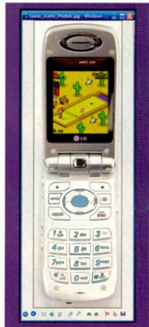
FIG. 2: Windows PCs are often the platform of choice for hardware emulators, such as Qualcomm's BREW emulator pictured here. An emulator is used to test sounds before delivery to a client.
