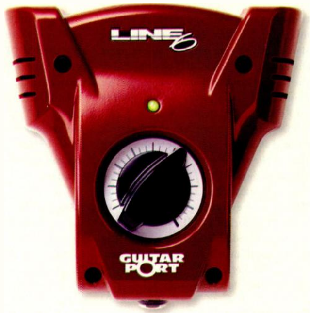
FIG. 1: The GuitarPort USB interface is the lone hardware component in the GuitarPort RiffTracker bundle. All user-interface functions, except for setting input volume, are handled in software.
