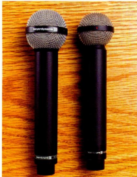
FIG. 10: The beyerdynamic M 260 and M 160 are unusual in the field of ribbon mics because they are end-address and have a hypercardioid polar pattern. The two mics, however, sound very different from each other, especially in the low-frequency response.
