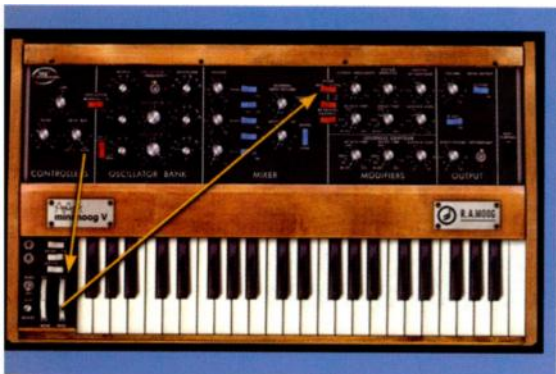
FIG. 1: This Arturia Minimoog patch uses noise to modulate the filter cutoff frequency. The amount of modulation is controlled by the Mod Wheel.
