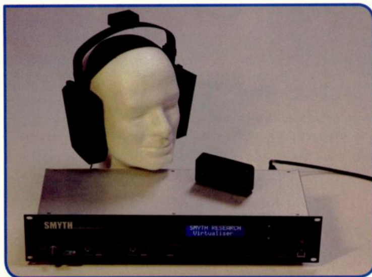
FIG. 1: The SVS system creates custom surround simulations for each user and room, and it includes a head tracker that senses the wearer's head position, so that the virtual speakers appear to remain stationary as the head moves.
