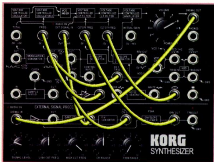
FIG. 1: The Korg MS-20 monophonic synth had a patching matrix, which is reproduced here in Korg's new software version of the same instrument.
