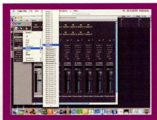
FIG. A: This figure shows the list of ReWire ports available to Logic. Note that some are named bus and some are named channel . Logic uses whatever term is given to it by the slave to identify each port.
