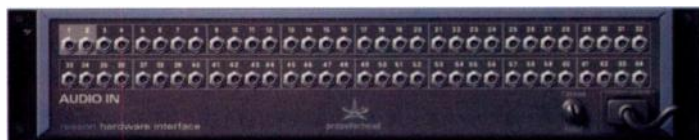
FIG. 2: Propellerhead Reason can supply as many as 64 channels of audio data to a ReWire host. The figure above shows the rear panel of the Reason rack where the 64 ReWire audio ports are accessed.
