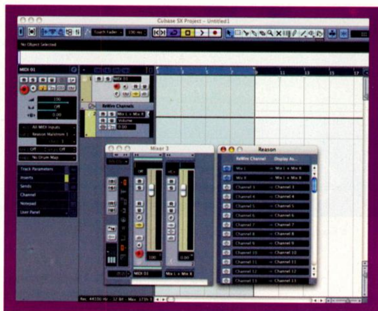
FIG 4: In this figure, the output of a Cubase MIDI track is directed to a Reason Malstrom device, and Reason's audio output is directed to a ReWire channel that is activated in the Device Manager.
