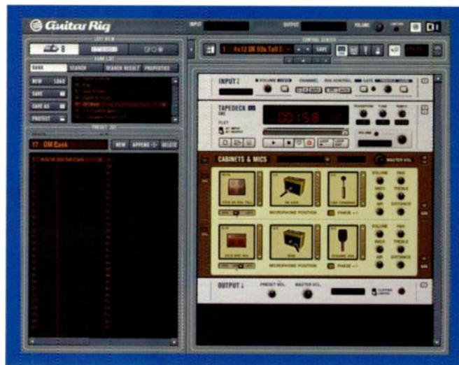
FIG. 4: Native Instruments Guitar Rig gives a large variety of speaker-cabinet models, microphone types and placements, and other options for dialing in your virtual cabinet.
