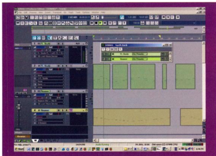
FIG. 1: Sonar's Synth Rack (shown here in track 1's data area) is used to create audio and MIDI connections to the ReWire slave.
