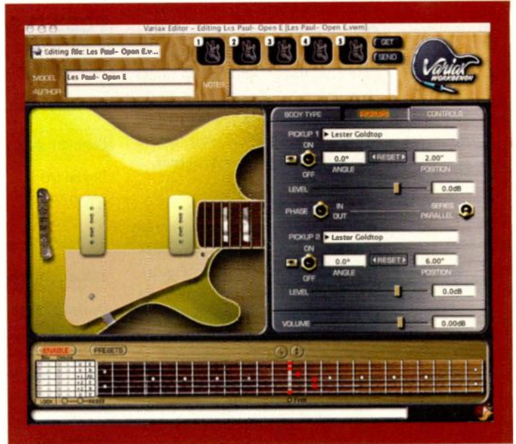
FIG. 3: Variax Workbench software allows you to construct your own custom guitar models and transfer them to your Variax's internal memory.
