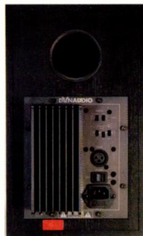
FIG. 2: The BM5A's rear panel includes an array of three equalization switches that can be set flat or provide bass shelving, midrange cut, or treble filtering.
