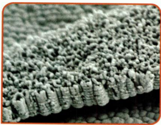
FIG. 1: Titanium dioxide nanotubes could dramatically decrease the energy cost of fabricating solar cells, and their efficiency will increase if the nanotubes can be grown longer than the 360 nm structures shown here.
