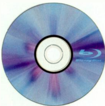
FIG. 3: This year will see the emergence of two new competing storage technologies: Blu-ray (pictured here) and HD-DVD. They will offer rewritable discs that can hold 25 GB and 15 GB, respectively.
