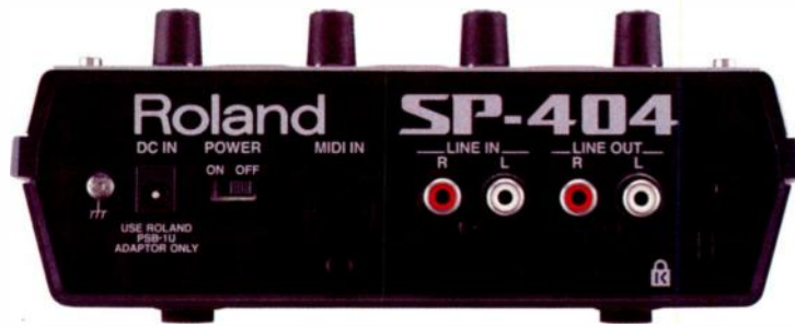
FIG. 2: Powered by a line-lump adapter or AA batteries, the SP-404 features MIDI In, stereo line-level I/O, and an antitheft cable slot. The front side has a headphone jack, a CompactFlash slot, and a mono mic input with level trim.
