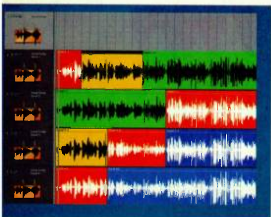
FIG. 2: One way to help keep track of the takes you're comping is to color code them by quality. If your sequencer allows for color coding of individual regions (such as in this example from Logic Pro), you can even color code individual phrases.
