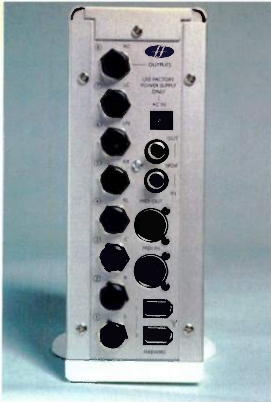
FIG. 2: The Saffire's rear panel has analog audio and S/PDIF jacks, as well as FireWire and MIDI ports. The power terminal attaches to the included DC adapter, but because the Saffire is normally powered by the FireWire bus, the adapter is required only for 4-pin FireWire connections.
