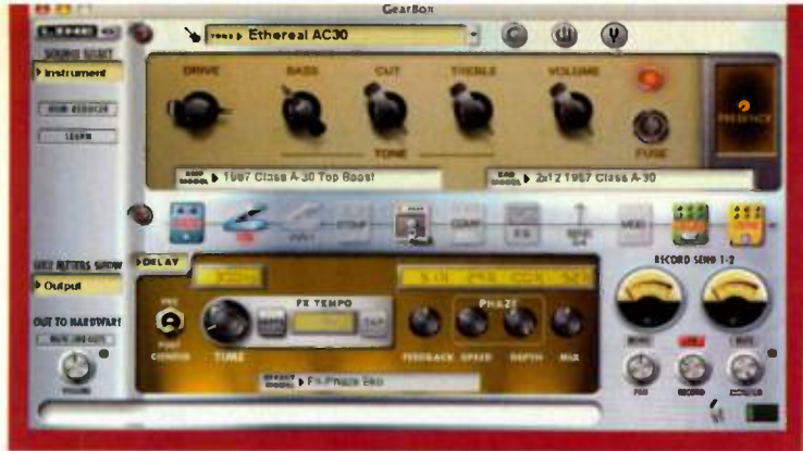
FIG. 3: The UX2 includes Line 6's GearBox software, which offers control over the TonePort hardware and access to the Line 6 amplifier and effects models.
