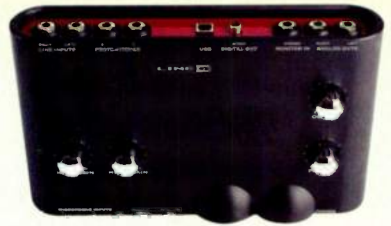
FIG. 2: This photo shows the top and rear panels of the UX2. There are knobs to control mic gain, headphone volume, and output volume.
