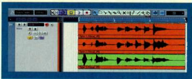
FIG. 3: Many sequencers, including Steinberg Cubase SX (pictured here), allow you to record vocal takes as nested tracks within a single track. Such features facilitate vocal comping by making it easy to manipulate and audition the various takes.
