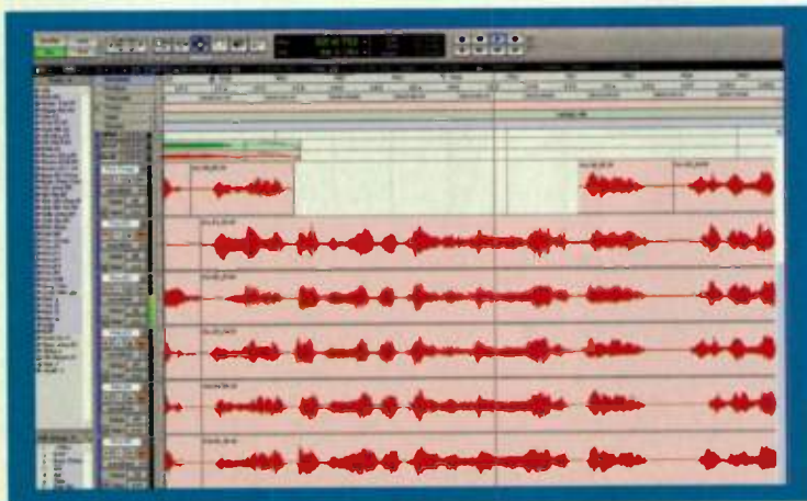
FIG. 4: Rogut's method for auditioning tracks when comping uses Pro Tools|HD's Mute Frees Assigned Voice feature. In this example, when the transport gets to the "hole" in the Vox Compt track, the audio from the track below will play for that section.
