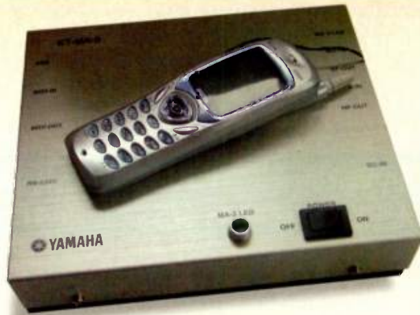
FIG. 2: Because it contains the same sound chip used in many phones, the Yamaha MA-3 synthesizer is useful for previewing your ringtones as they will sound on the actual handset hardware.
