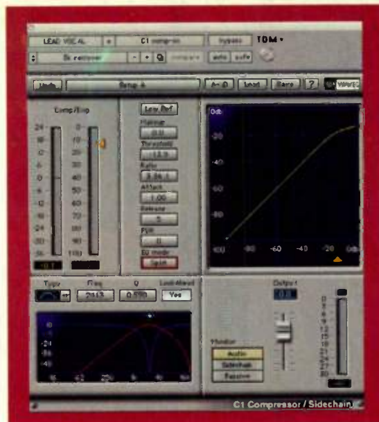
FIG. 1: One of Pensado's favorite dynamics plug-ins is Waves C1 Compressor/Sidechain. This screen shot shows the settings he used for Mary J. Blige's vocals on "Be Without You."
