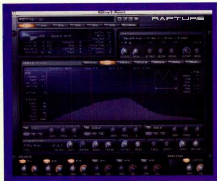
FIG. 2: Rapture's modulators include a dedicated step generator for pitch, filter cutoff, filter resonance, pan, and amplitude.
