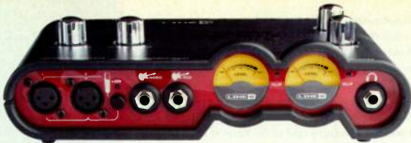
FIG. 1: The TonePort UX2 USB interface lets you plug in guitars, microphones, and line-level effects, and send the output to either analog or digital gear.
