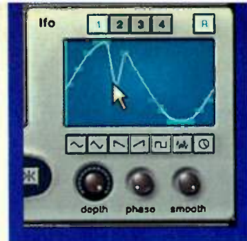
FIG. 3: By clicking-and-dragging on the LFO waveform in Steinberg XpHraze, you can change its shape. The smoothing knob controls how smooth or stepped the waveform will be.
