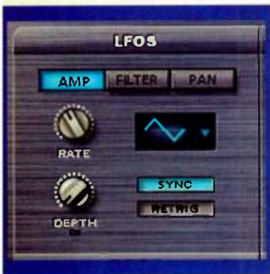
FIG. 2: The buttons along the top in the LFO section of Spectrasonics Stylus RMX may look like destination selectors, but in fact, RMX has three separate LFOs, each with a single dedicated output routing. One LFO modulates the output amplitude of the voice, another modulates filter cutoff, and another modulates panning. Because RMX is a percussion instrument, it has no pitch LFO.
