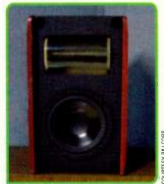
FIG. 2: A semicylindrical midrange/tweeter driver could be mated with a conventional woofer to cover the entire frequency spectrum while radiating the mids and highs evenly along the vertical axis.
