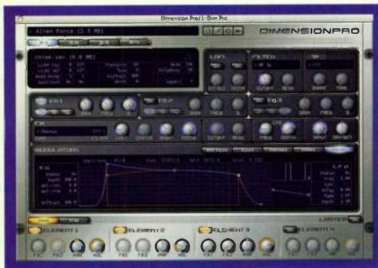
FIG. 1: Dimension Pro's Element control panel houses multisample and DSP controls (top), EQ and effects controls (middle), and graphical filter and LFO controls (bottom).
