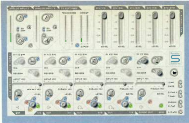
FIG. 3: SaffireControl furnishes a software front end for the hardware. It gives you complete control of input and output levels, signal routing, and plug-ins, allowing the Saffire to function as either a mixer or a standard sound card.
