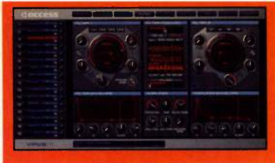
FIG. 3: VirusControl is a software plug-in that integrates the Virus TI with audio sequencers. The Filter page offers control of two filters, two envelope generators, and the amplifier.
