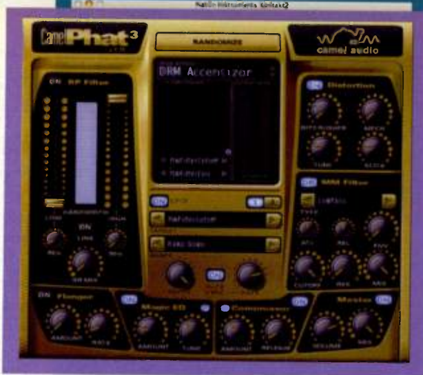
FIG. 1: CamelPhat's control panel layout mirrors the signal flow from BP Filter (top left) to the master output (bottom right).
