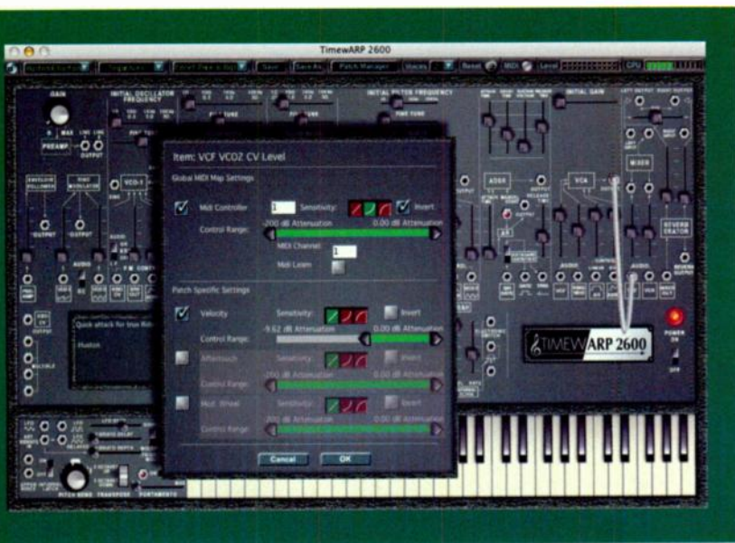
FIG. 2: TimewARP 2600 responds to a wide range of MIDI continuous controllers. Most parameters have a dialog box such as the one shown here to set up MIDI control.
