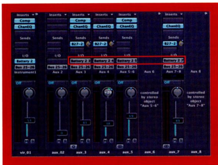
FIG. 1: The red box indicates where to select the appropriate Battery output pairs for each aux object in the Logic Environment window.
