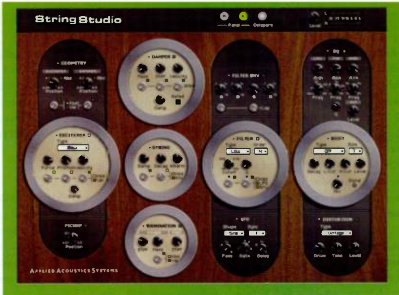
FIG. 1: Control panel B houses the settings for the elements of the physical model.
