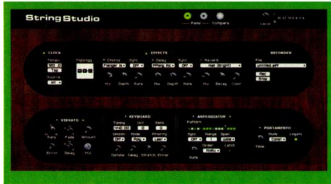
FIG. 2: Control panel A contains the effects controls (top) and controller settings (bottom).
