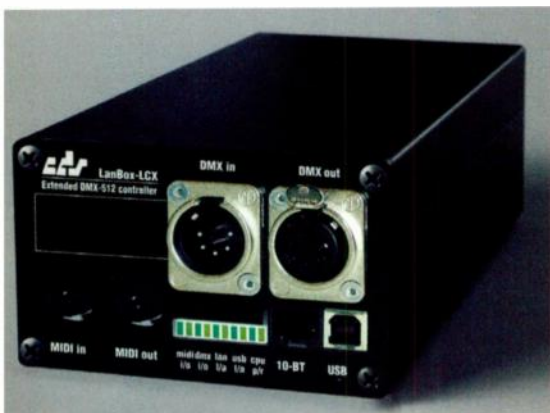
FIG. 1: The LanBox-LCX theatrical controller can send and receive messages in the DMX lighting protocol or in the MIDI protocol. It can be connected to a computer via USB or Ethernet.
