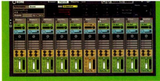
FIG. 3: A Kore Performance hosts KoreSounds, which you can enable, split, and select using Performance presets.
