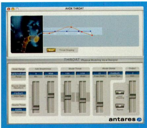
FIG. 3: Antares Throat models the human vocal tract. Not surprisingly, it is most convincing when you use it to make subtle rather than drastic changes to vocal characteristics.
