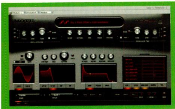
FIG. 2: Modulo offers two oscillators and plenty of modulation options.
