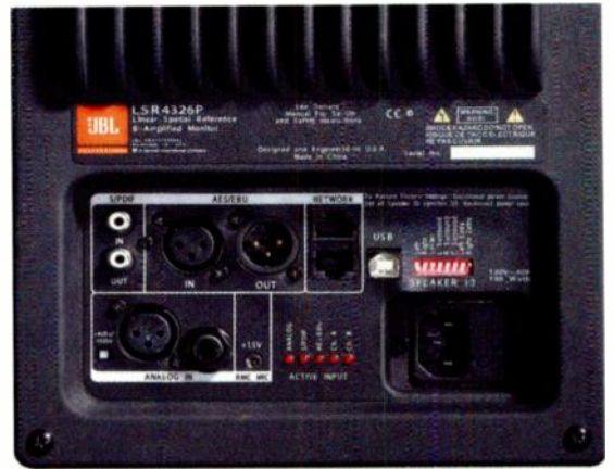
FIG. 2: The LSR4326P's rear panel provides XLR and TRS analog connections, AES/EBU and S/PDIF digital connections, and USB and Ethernet ports for control functions, as well as a phantom-powered input for the RMC measurement mic.
