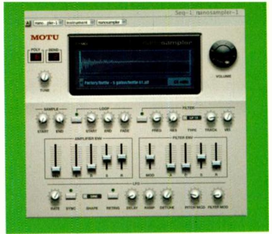
FIG. 3: Nanosampler makes it easy to add a MIDI-triggered sample to your project.
