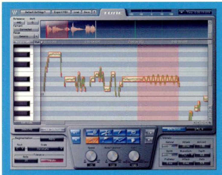
FIG. 10: Waves Tune is a multifORMAT plug-in that can scan and manipulate pitch and tempo for tracks as long as ten minutes. Pitch changes appear as a series of blocks and curves.
