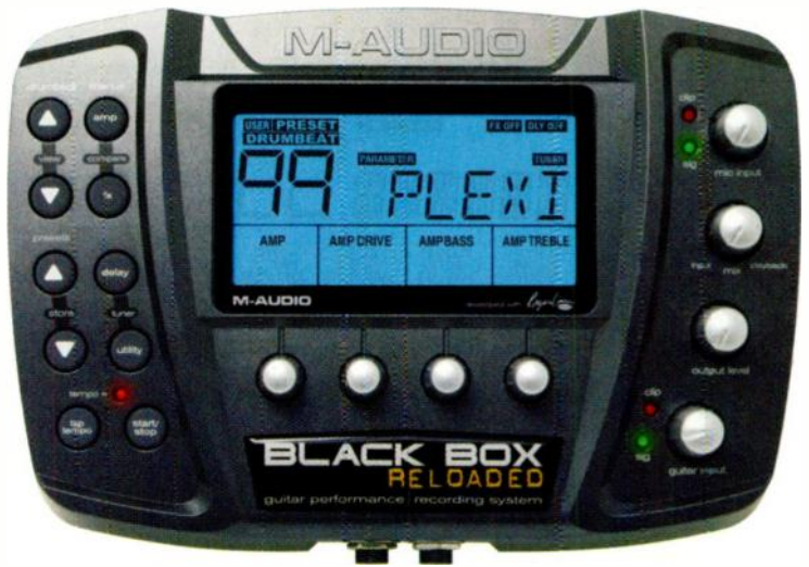
FIG. 2: The M-Audio Black Box is one of several guitar-recording devices on the market that offer amp, cabinet, and effects modeling, and a USB audio interface for recording direct.
