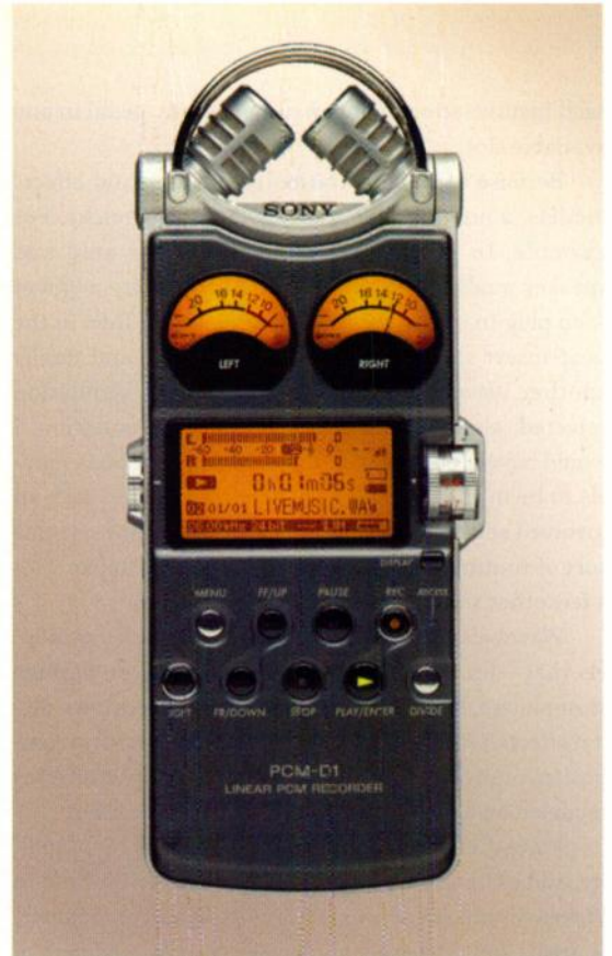
FIG. 1: The meters, LCD readout, and essential buttons are conveniently arranged on the PCM-D1's front panel.
