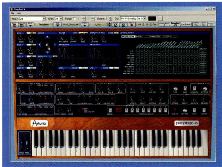
FIG. 1: In Hybrid mode, Arturia Prophet-V combines the features of a Prophet-5 (bottom) and a Prophet-VS (top). The joystick (upper left) can be assigned to two MIDI Control Change messages, so you can sweep through the oscillator mix in real time.
