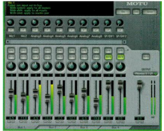
FIG. 3: The CueMix Console software allows easy routing, mix recall, and file management, much of which can also be accomplished from the UltraLite's front-panel controls.
