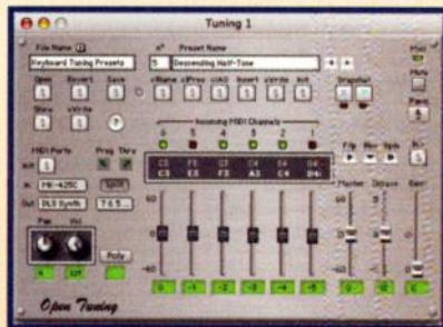
FIG. A: Phi Software Open Tuning 1.5.1 lets you transpose the MIDI output of individual MIDI guitar channels and perform a variety of MIDI mapping tricks.
