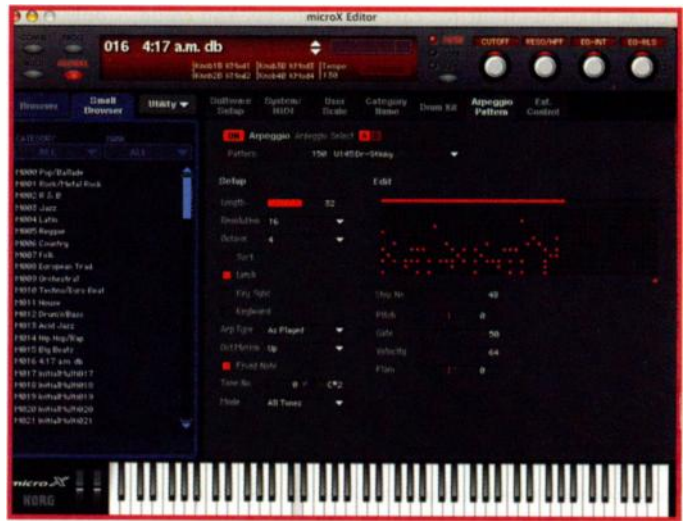
FIG. 3: Running as either a plug-in or a standalone program, the microX editor-librarian updates the keyboard instantly over USB—and vice versa. This screen shot shows the arpeggiator pattern editor, which would benefit from MIDI note input.
