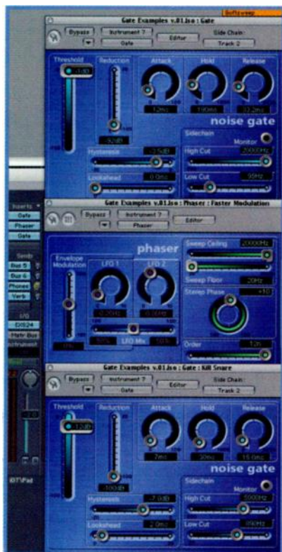
FIG. 1: A phaser is inserted between two gate effects. The different settings on the two gates allow the phaser-processed portion of the signal to be shorter than the nonprocessed part.
