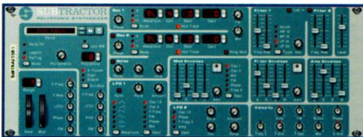
FIG. 1: Although this Subtractor patch in Propellerhead Reason 3.0 has a slow attack, you can set the Amplitude Attack knob in the Velocity section's lower-right corner to speed up the envelope's attack segment with higher Velocities.
