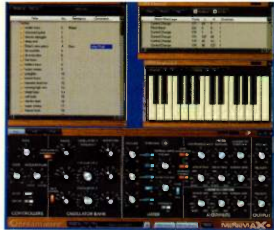
FIG. 3: The Minimax's remote control software offers patch management and control of certain features that are not accessible from the hardware knobs and switches.
