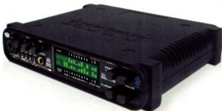
FIG. 1: The MOTU UltraLite's unique features include independent 3-way pad switches and phantom power on mic channels, as well as four active and assignable monitor mixes.
