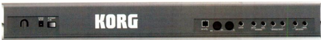
FIG. 2: The microX's back panel includes four audio outputs, three pedal inputs, MIDI In and Out jacks, and a USB port. The keyboard can't run off USB power, though; an AC adapter is required. The headphone jack is at the front.
