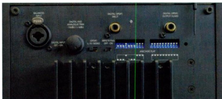
FIG. 2: Twenty DIP switches on the 6D’s rear panel activate filters that compensate for compromised speaker placement, such as on a shelf, against a wall, or in a corner.
