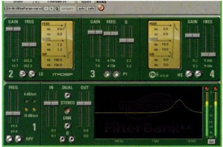
FIG. 1: The EQ component of Project Studio is FilterBank LE. One of its configurations is E4, which offers high and low shelving filters, a parametric band, and a highpass filter.
