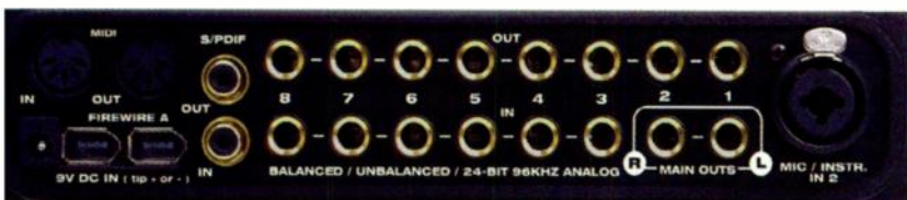
FIG. 2: The UltraLite's extensive I/O includes ten analog outputs and S/PDIF, MIDI, and dual FireWire ports.
