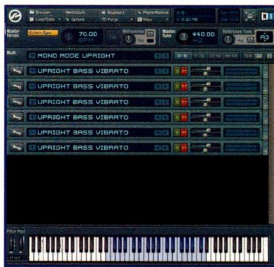
FIG. 4: Here is a multitimbral patch I created in Native Instruments Kontakt 2. Each part uses the same bass patch assigned to one of the six MIDI channels of the guitar, and each part is restricted to single-note polyphony. In addition to conserving CPU cycles, this setup helps the samples perform like a real bass, with successive notes on the same string cutting the previous note short.
