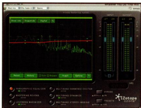
FIG. 5: iZotope Ozone 3 incorporates six mastering processors that alternately share the same window. The graphic display for the Paragraphic Equalizer module is shown here.
