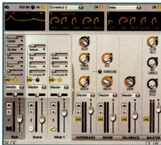
FIG. 2: Strike's mixer allows you to blend mic positions, add insert effects, and control the levels of individual drums through MIDI.
