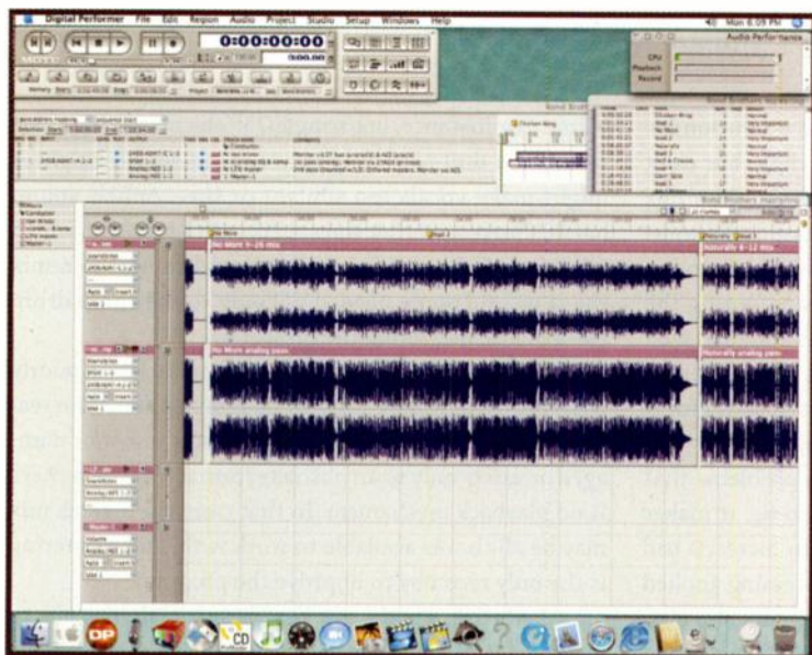
FIG. 1: A multichannel mastering setup in MOTU Digital Performer 5. Each track is routed to a different stereo digital output feeding the same downstream monitoring path so the engineer can monitor each one separately in turn as they all play back. Note the markers placed at the beginning and in peak sections (the latter denoted by the word loud ) of each file.
