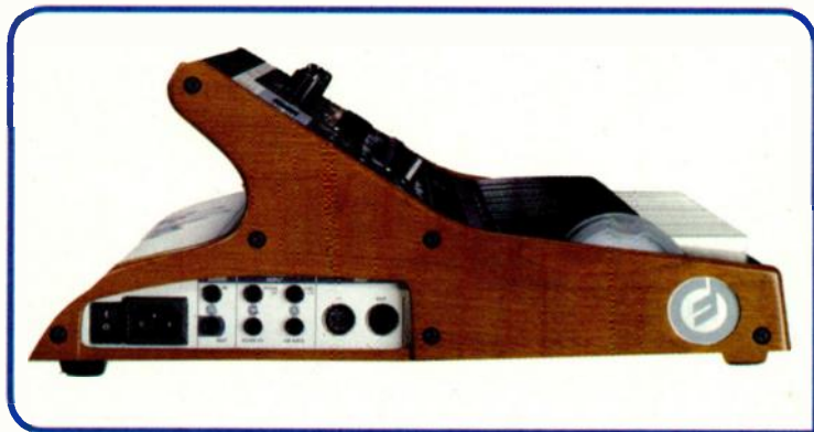
FIG. 2: The Little Phatty's left side panel contains an unbalanced audio output, an unbalanced audio input, a gate input, and control voltage inputs for pitch, volume, and filter cutoff—all on ¼-inch jacks—as well as MIDI In and Out ports and an AC power connection.
