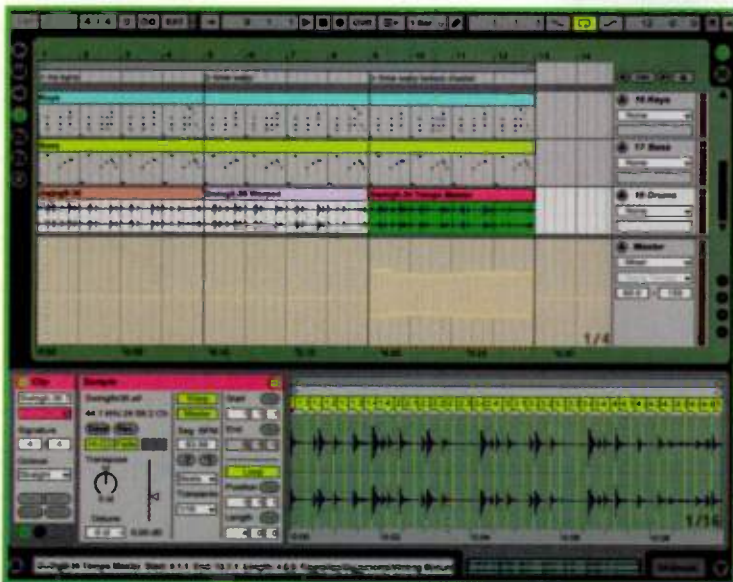
FIG. 1: Assigning an audio clip in Arrangement view as the tempo master automatically generates tempo changes matching the clip's Warp markers.
