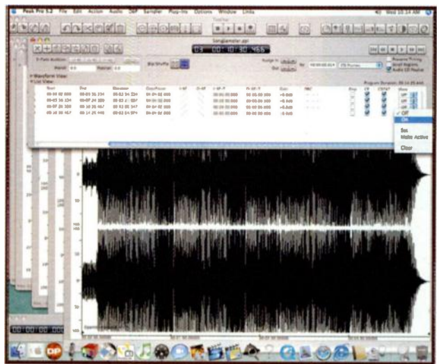
FIG. 2: In the rightmost column of the List view for BIAS Peak Pro's Playlist, Vbox plug-ins can be turned on and off as a group with one mouse-click to facilitate A/B comparisons between dry and processed mixes.
