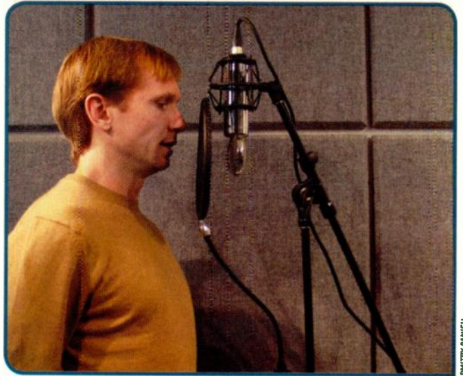
FIG. 4: The most effective miking technique for recording voice-overs is to place the mic between 3 and 4 inches from the voice actor's mouth, with the mic capsule aligned with the actor's upper lip and a windscreen positioned halfway between.
