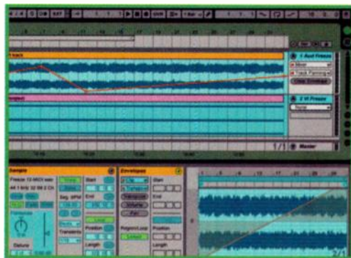
FIG. 2: Frozen tracks render all clips as audio, but you can still move and resize clips and add mixer automation.
